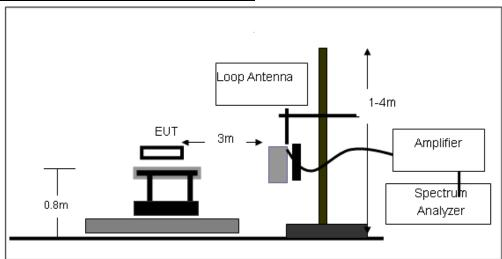
Radiated emission test-up frequency 30MHz~1GHz
