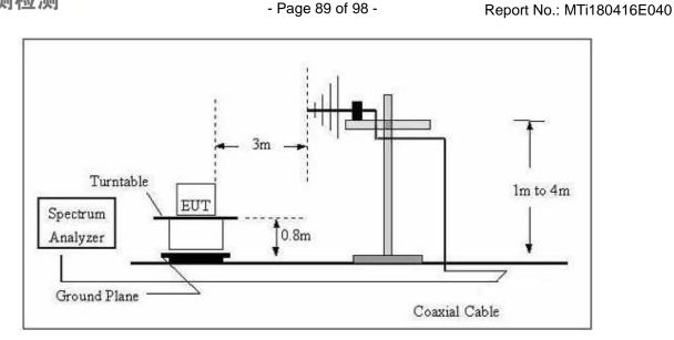
Radiated emission test-up frequency above 1GHz
