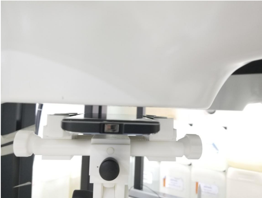
Body Front side(separation distance is 10mm)
