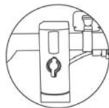
Fill and fix the rubber plug after the charging
