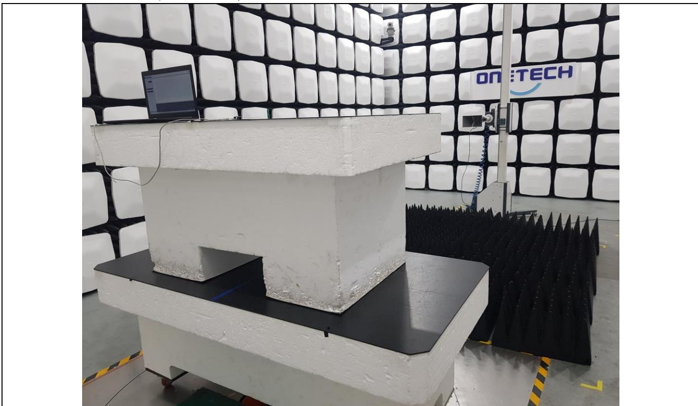
**[Multiple model: BoT-TMA50DS]****- Conducted Emission Test**
