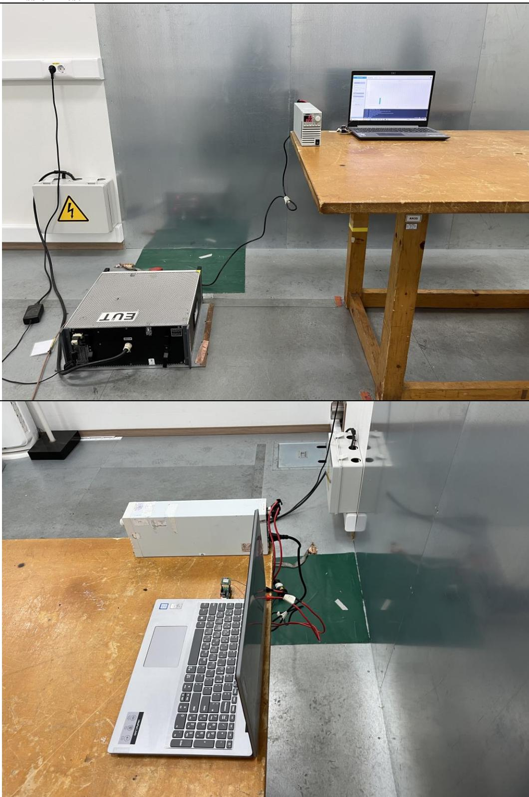
**- Radiated Emission Test (Below 1 GHz)**
