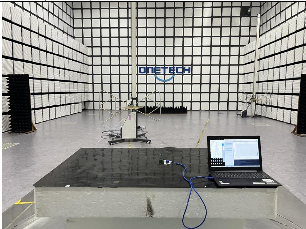
**- Radiated Emission Test (Above 1 GHz)**
