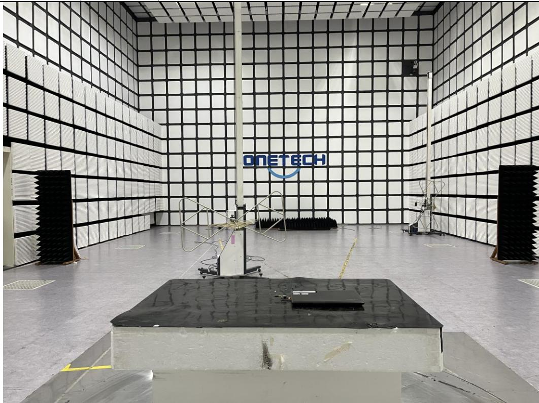
**- Radiated Emission Test (Above 1 GHz)**
