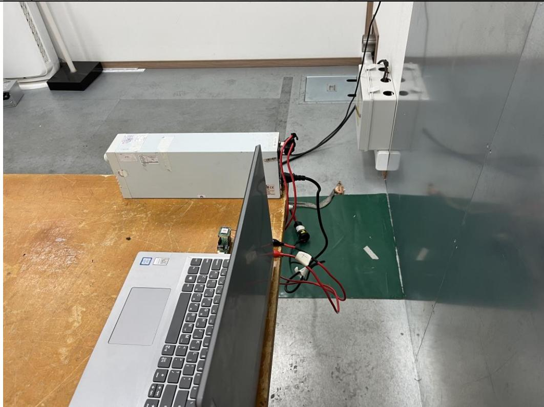
**- Radiated Emission Test (Below 1 GHz)**
