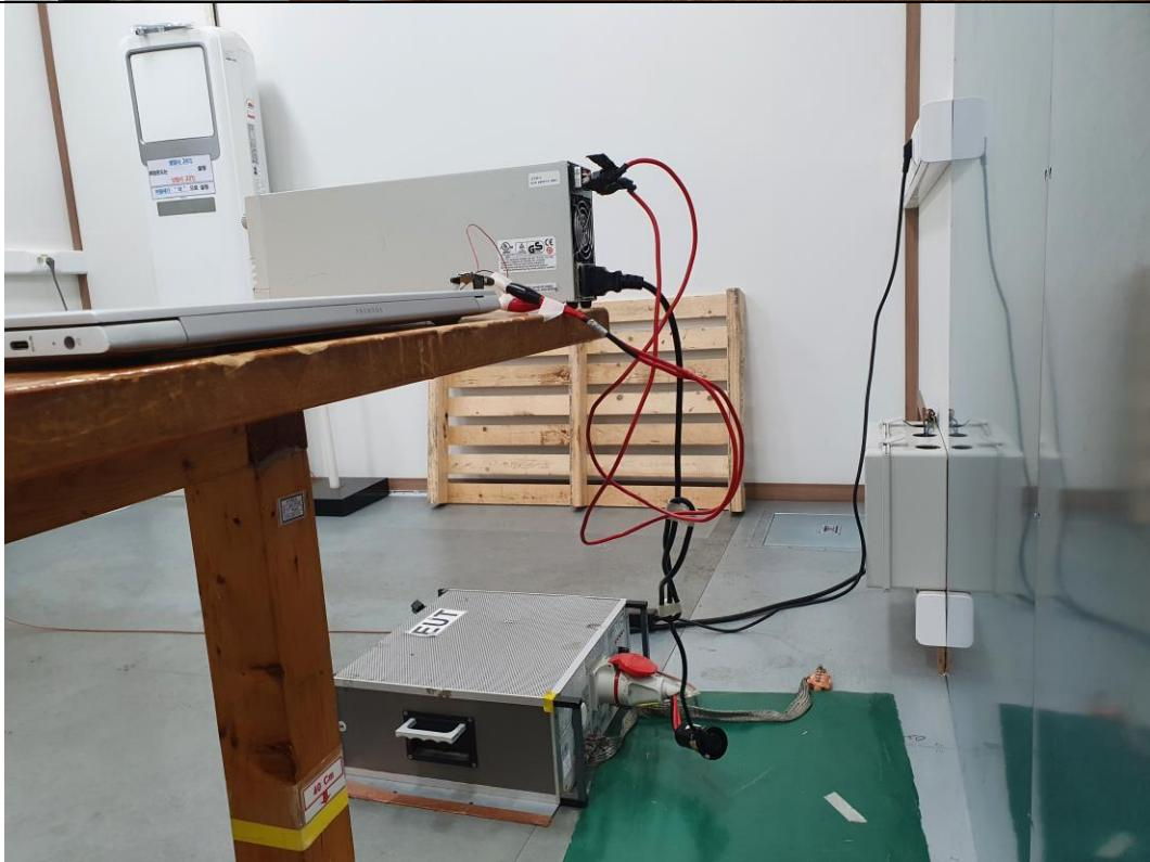
**- Radiated Emission Test (Below 1 GHz)**
