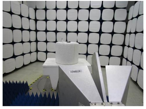
1.3 Radiated Spurious Emissions Test Setup
