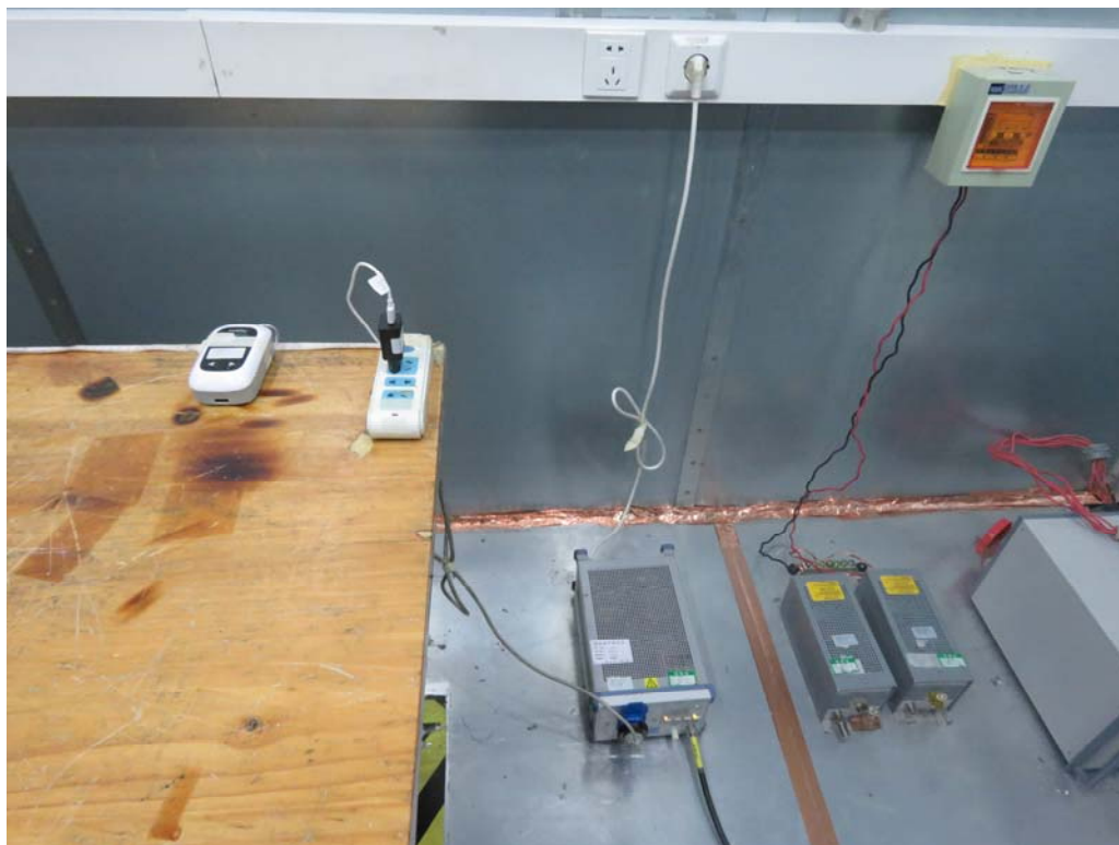
Picture 2 Conducted Emission Test Setup
