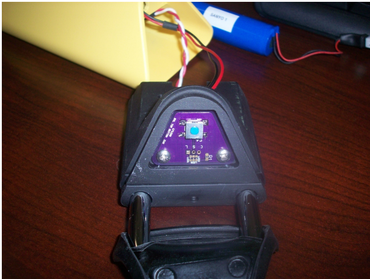
Figure 7. PCB Inside Locking Mechanism (Bar Code Scanner)
