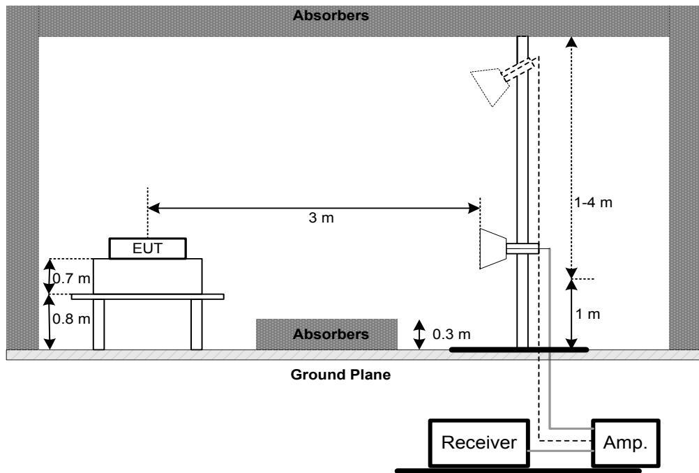
(C) For radiated emissions 9 kHz-30 MHz
