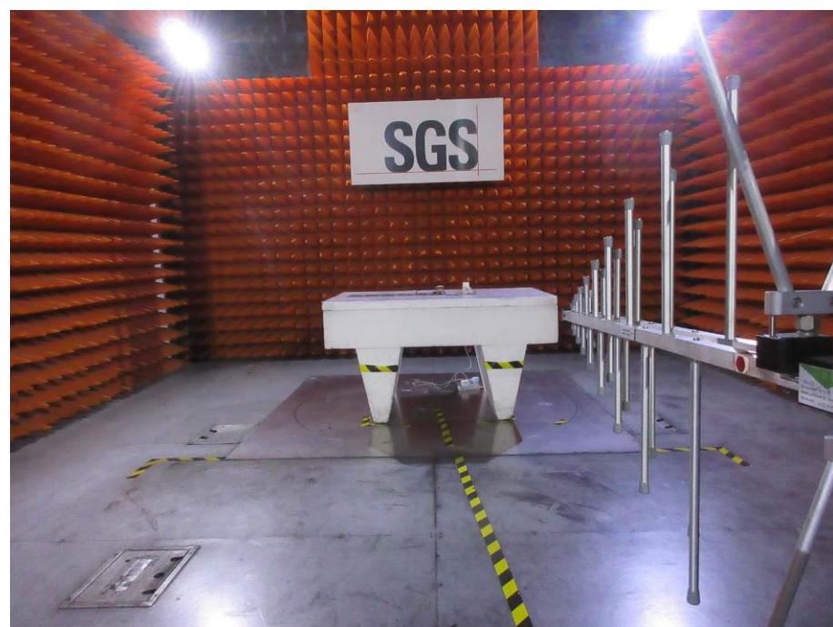
**2.3 Radiated Emissions (Magnetic field Strength)(9kHz-30MHz) Test Setup**
