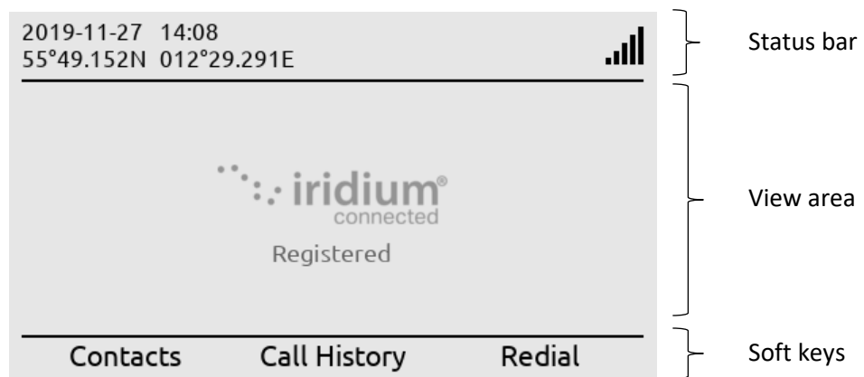
Figure 32: LT-3110S Control Unit - UI display sections
