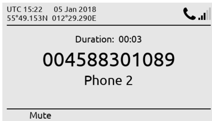
Figure 39: LT-3110S Control Unit – voice call successfully connected.
