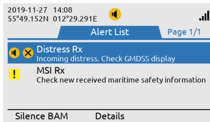
Figure 41: LT-3110S Control Unit - UI alert list
