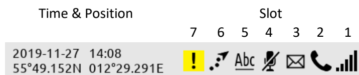
Figure 33: LT-3110S Control Unit - UI status bar
