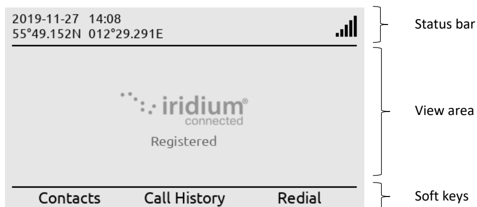
Figure 32: LT-3110S Control Unit - UI display sections
