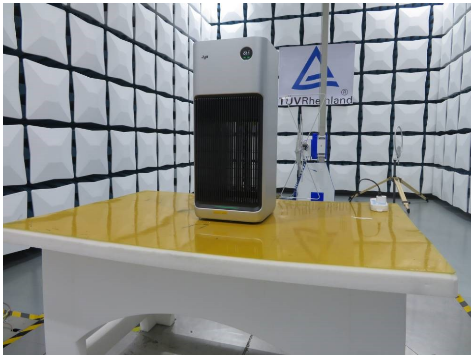
Photograph 2: Set-up photo for Radiated Spurious Emission, 30MHz - 1GHz
