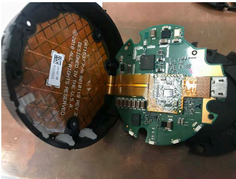
CAT 14535 main board, FPC Atmel and capacitance touch sensor
