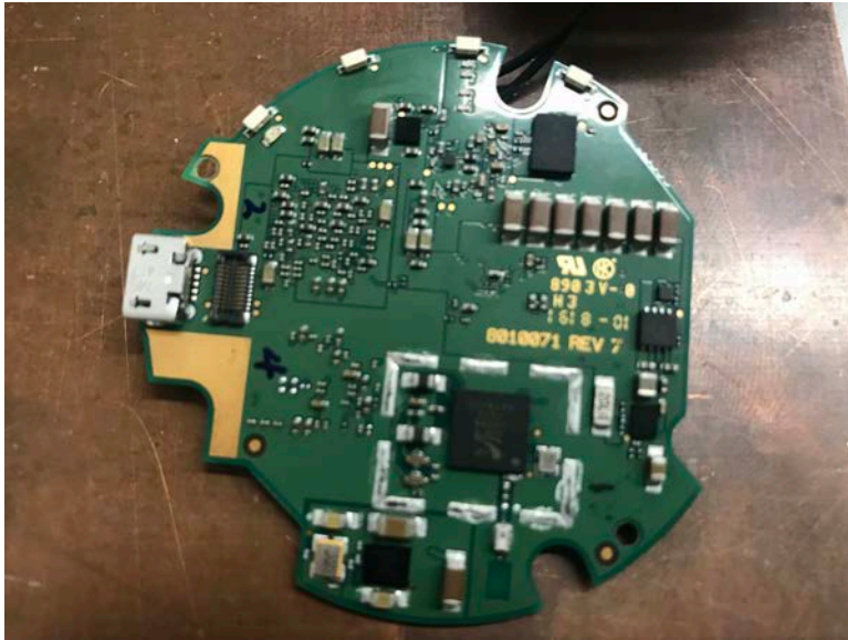
main PCB, top side with Bluetooth SoC
