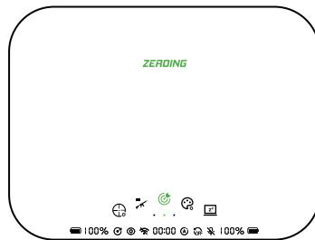
Take a shot, make the cross center of the reticle at point of impact. Short press MENU/REC button to switch zeroing options.
