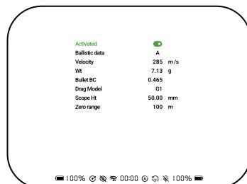
**Ballistic data** - Maximum storage capacity for 5 types of bullets.
