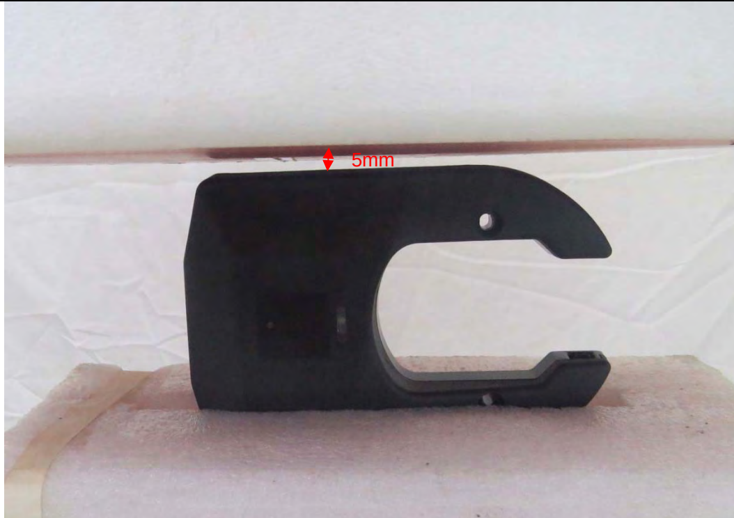
Picture 7: Right Edge, the distance from handset to the bottom of the Phantom is 5mm
