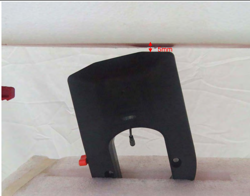
Picture 9: Top-Right Tilt, the distance from handset to the bottom of the Phantom is 5mm
