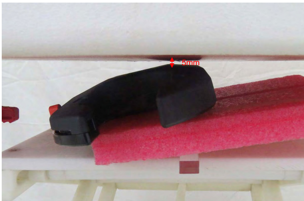
Picture 6: Front-Right Tilt, the distance from handset to the bottom of the Phantom is 5mm
