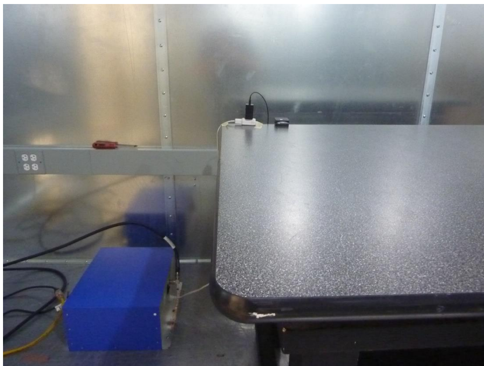
Figure 1: Test Setup for Conducted Emission – Front (AC Mains)
