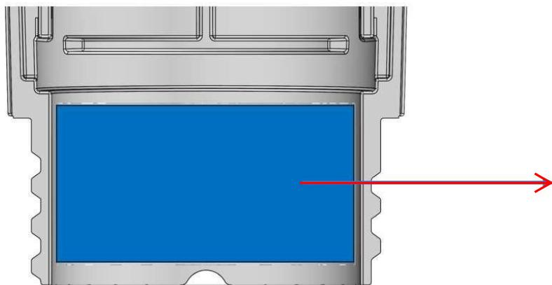
\*The label will be placed inside the battery compartment.
