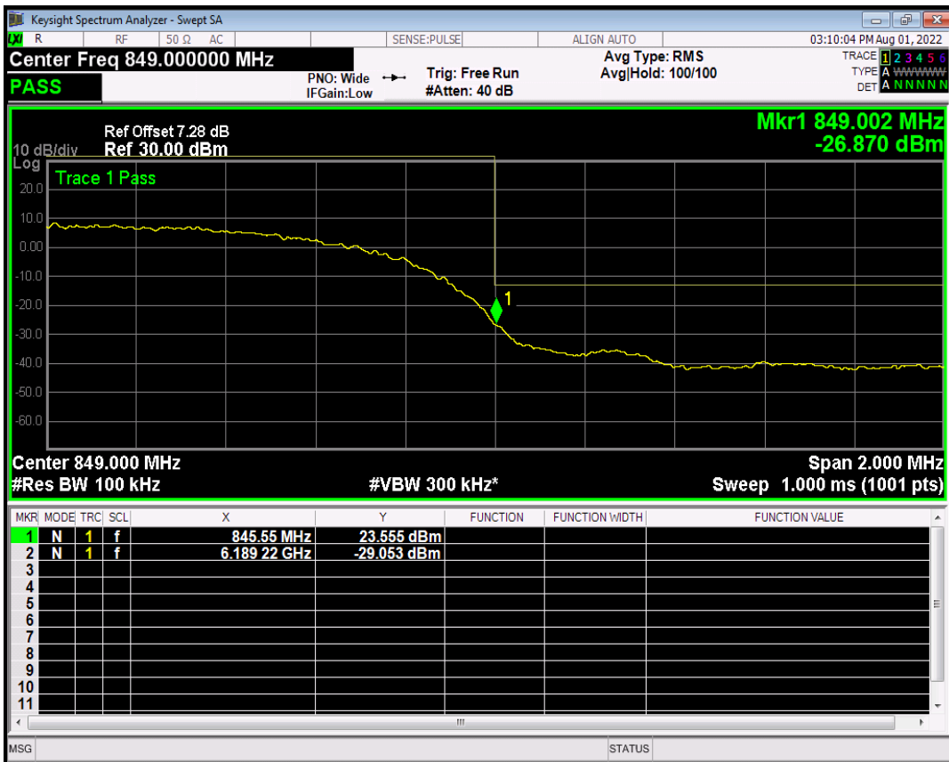
HSDPA Band5 Subtest2 Channel=4233
