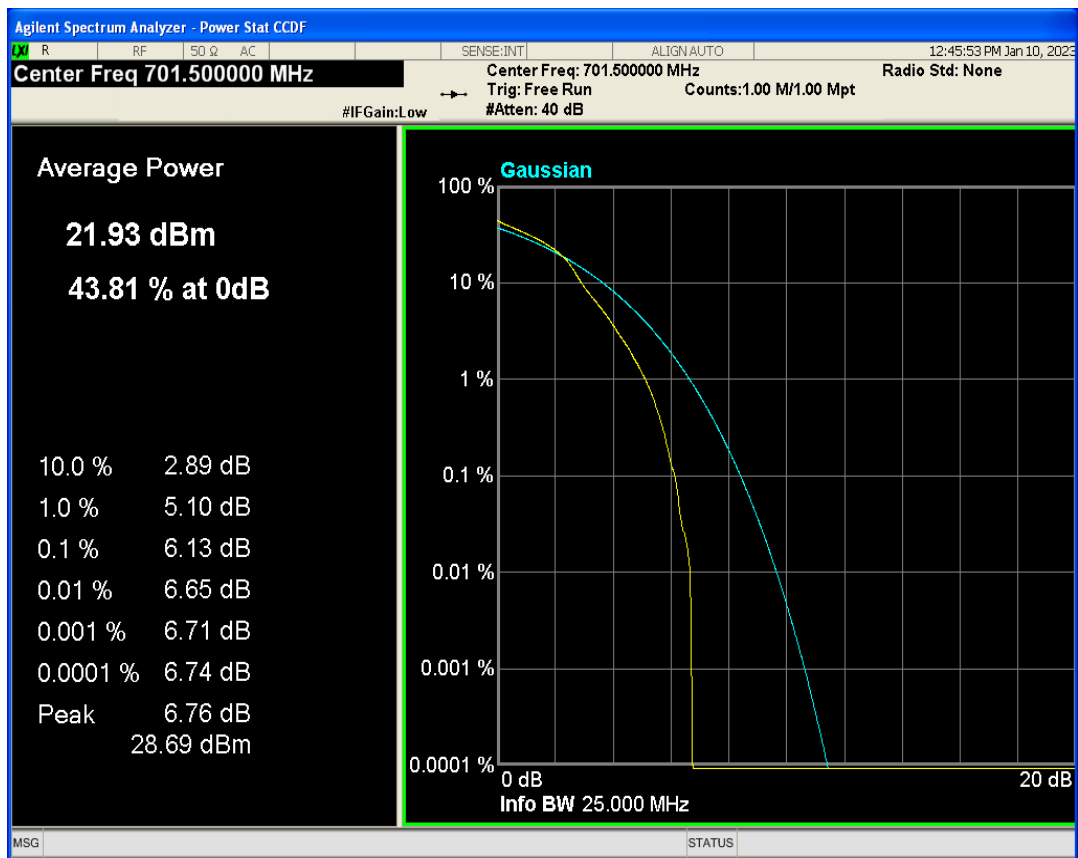
Band12 16QAM BW=5MHz Channel=23095 RB Size=1 Position=#0
