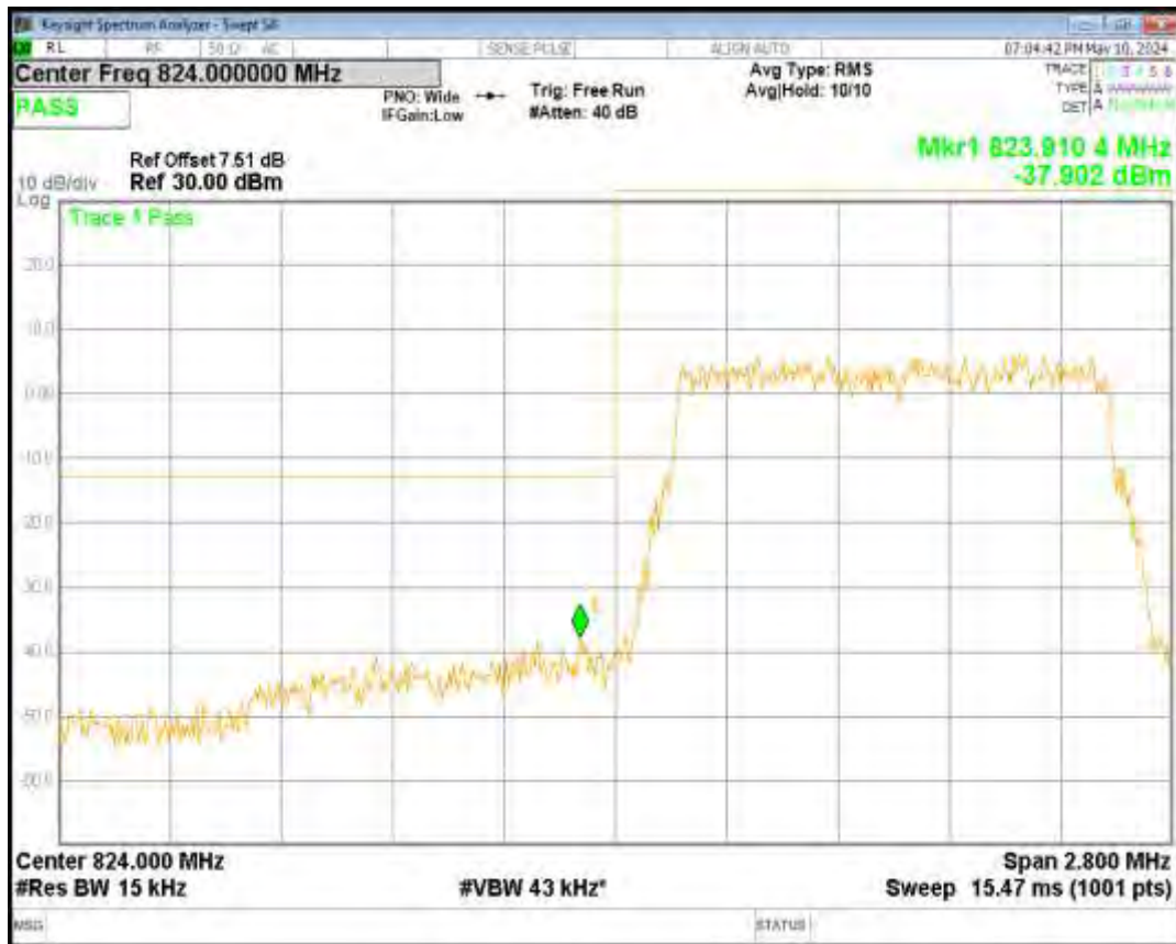
Band26(824-849) 16QAM BW=5MHz Channel=27015 RB Size=25 Position=#0
