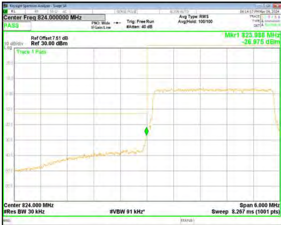
Band5 16QAM BW=3MHz Channel=20635 RB Size=15 Position=#0
