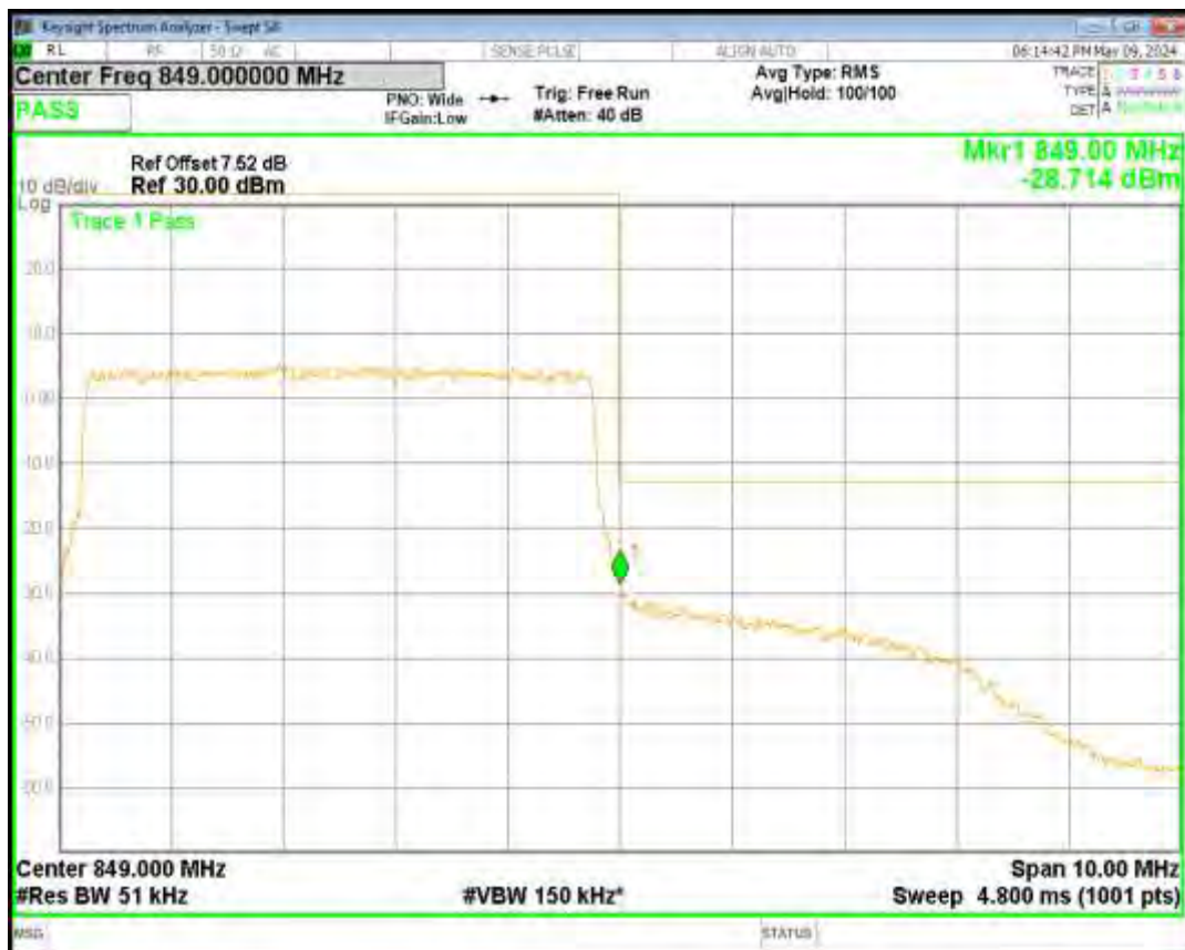
Band66 16QAM BW=1.4MHz Channel=131979 RB Size=6 Position=#0
