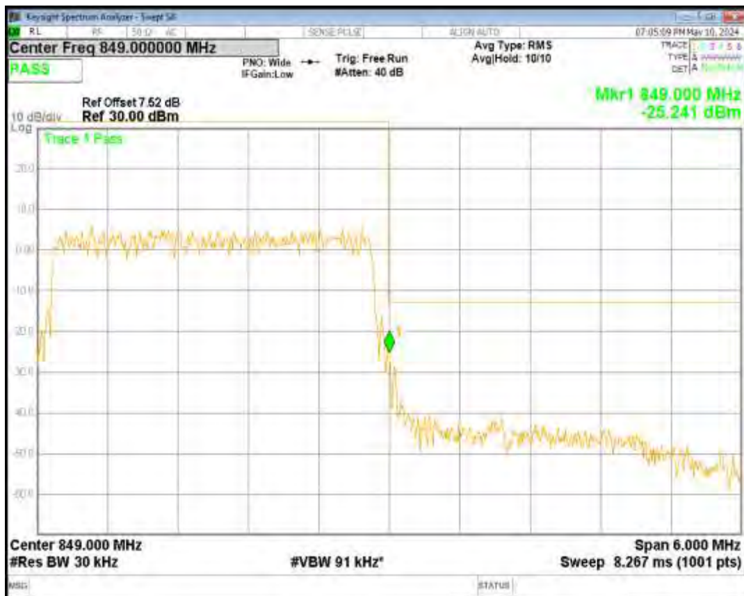
Band26(824-849) QPSK BW=5MHz Channel=26815 RB Size=25 Position=#0
