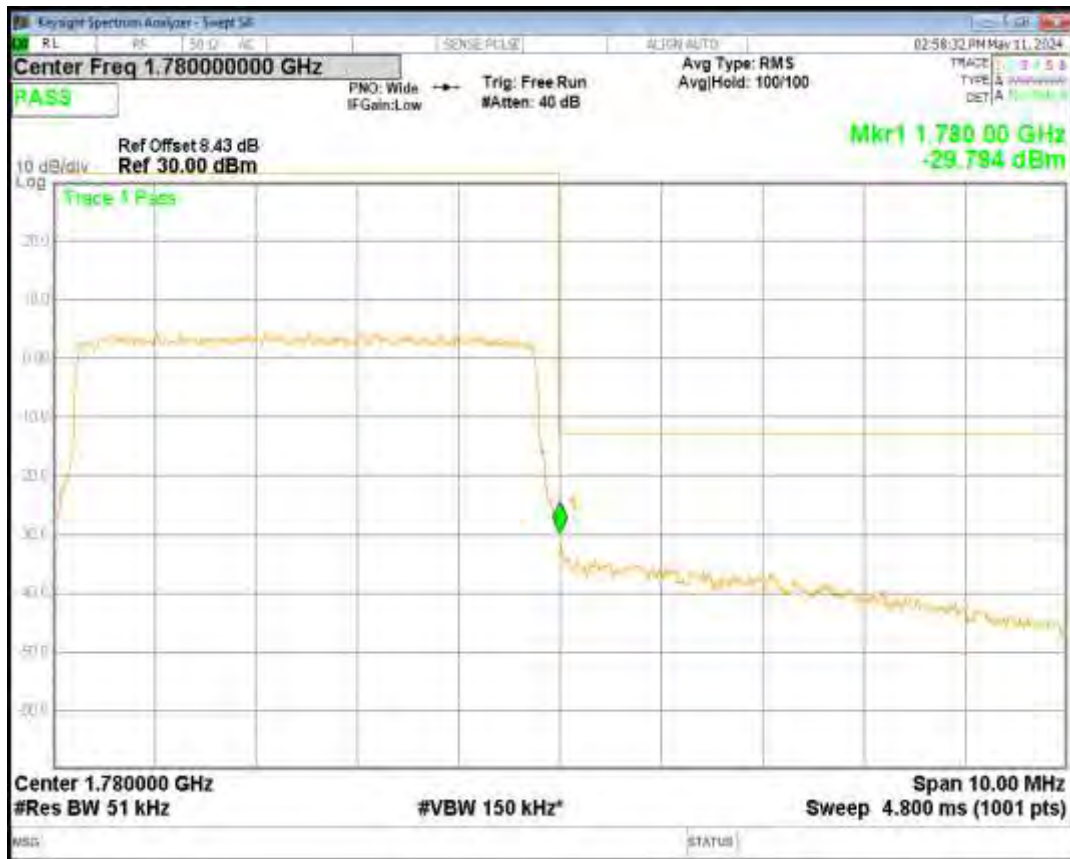
Band66 16QAM BW=20MHz Channel=132072 RB Size=100 Position=#0
