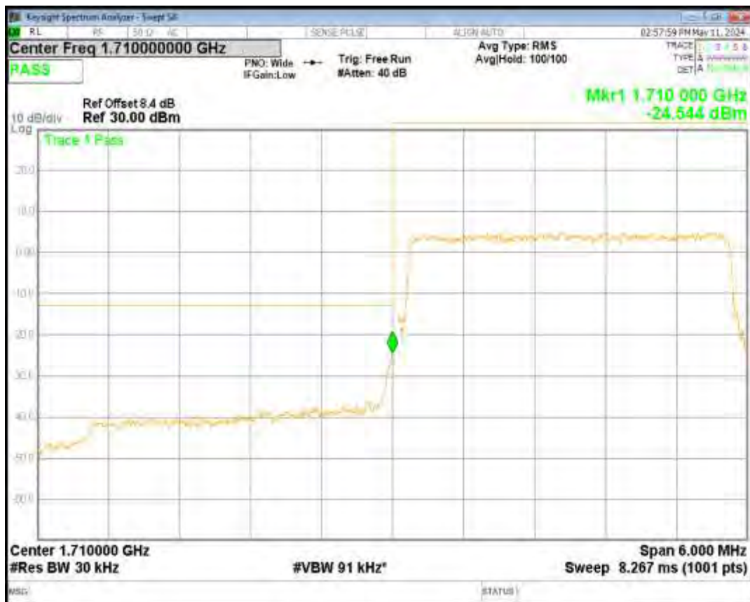
Band66 QPSK BW=3MHz Channel=132657 RB Size=15 Position=#0
