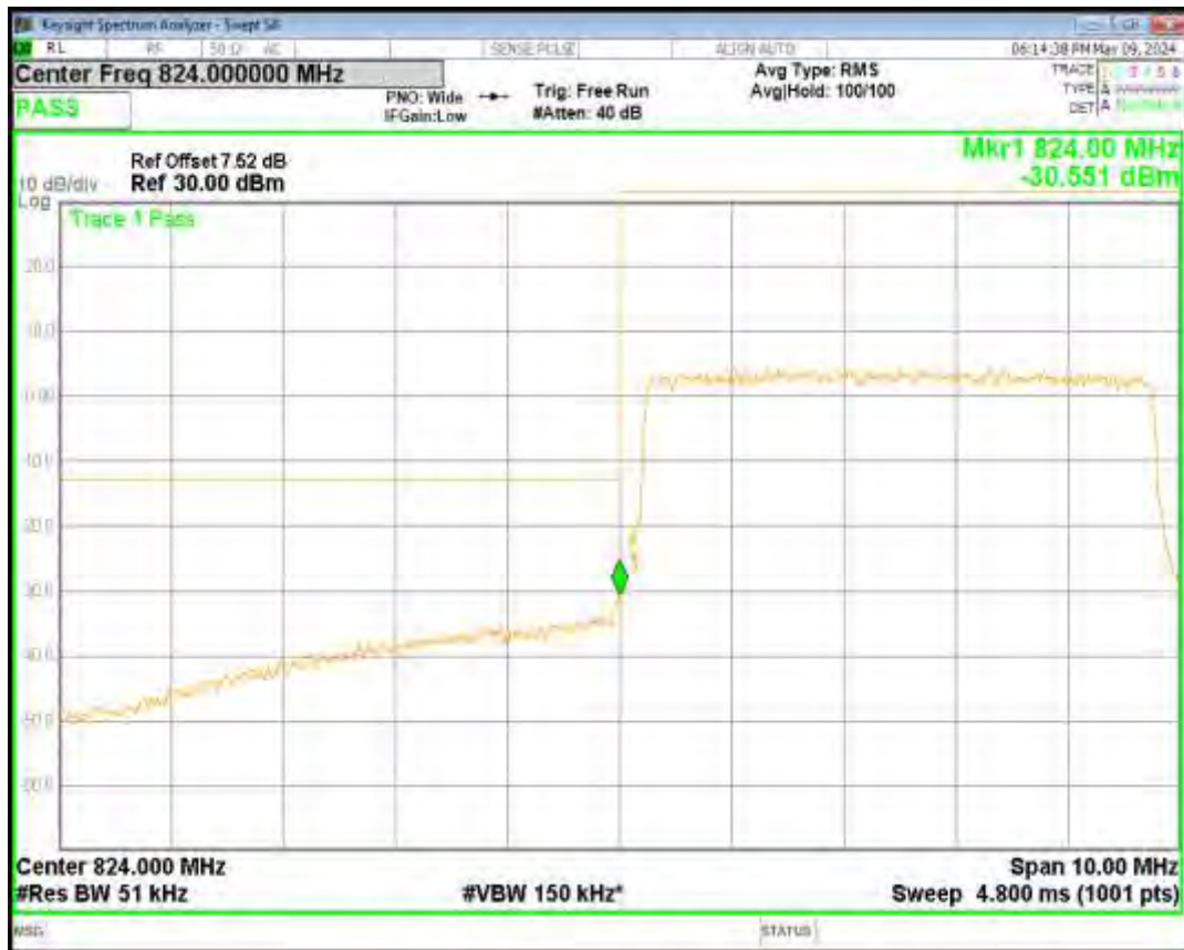
Band5 16QAM BW=5MHz Channel=20625 RB Size=25 Position=#0
