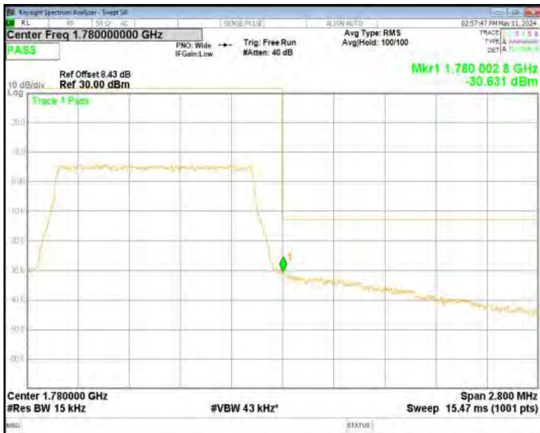
Band66 QPSK BW=1.4MHz Channel=131979 RB Size=6 Position=#0
