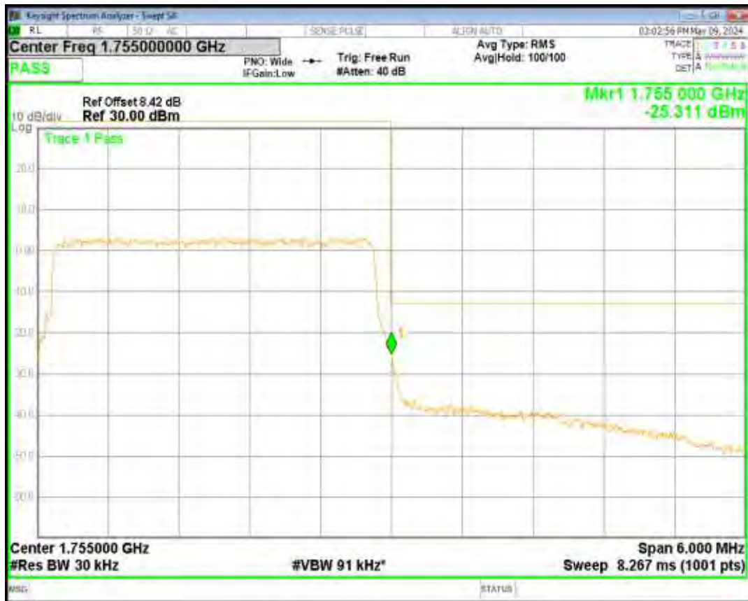
Band4 QPSK BW=10MHz Channel=20350 RB Size=50 Position=#0
