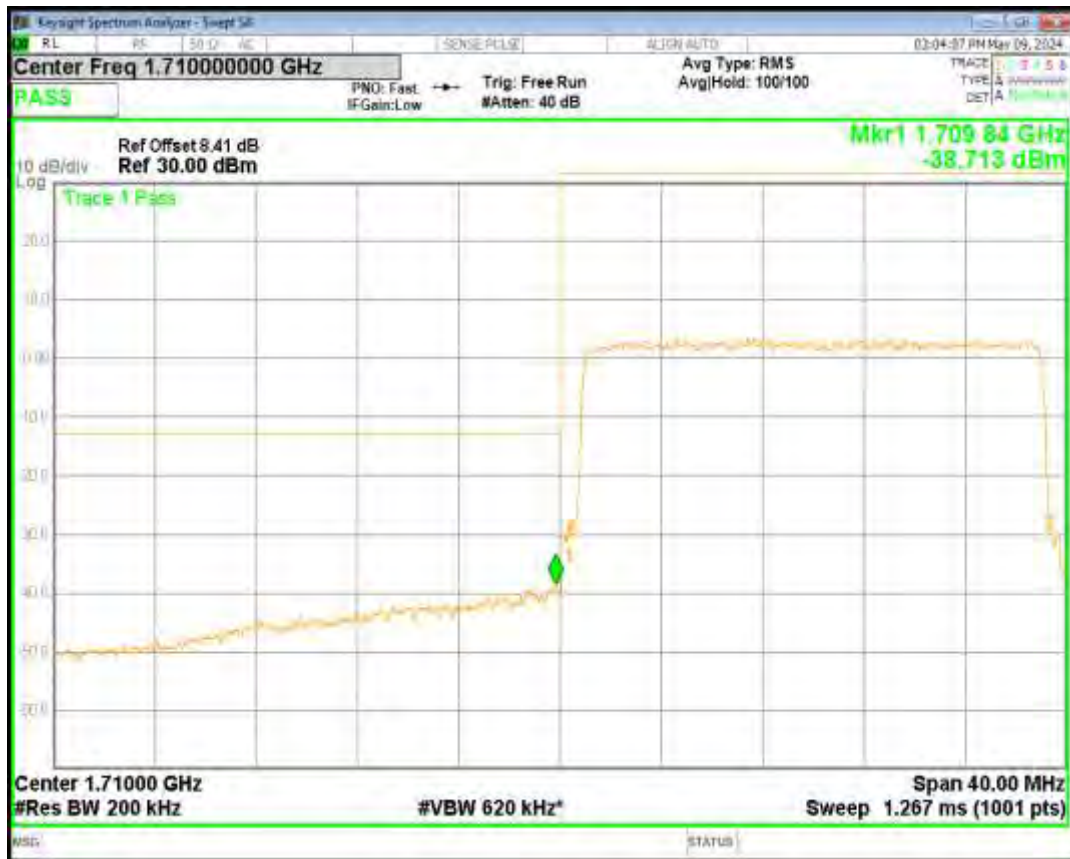
Band4 16QAM BW=20MHz Channel=20300 RB Size=100 Position=#0
