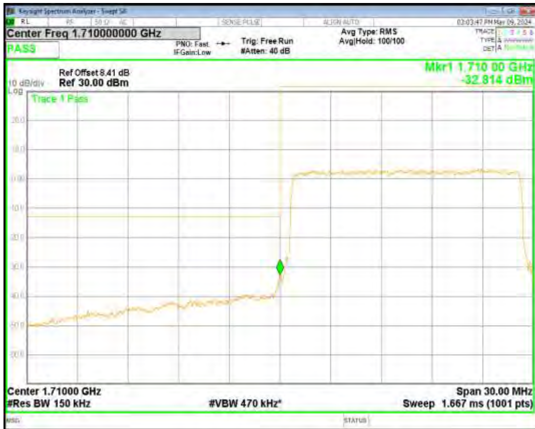
Band4 16QAM BW=15MHz Channel=20325 RB Size=75 Position=#0
