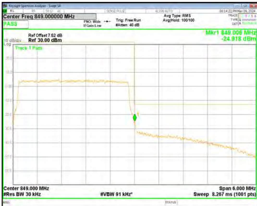
Band5 QPSK BW=5MHz Channel=20425 RB Size=25 Position=#0
