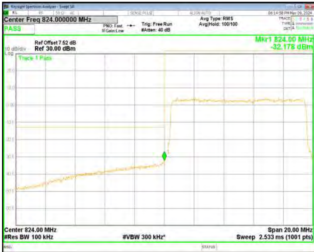
Band5 16QAM BW=10MHz Channel=20600 RB Size=50 Position=#0
