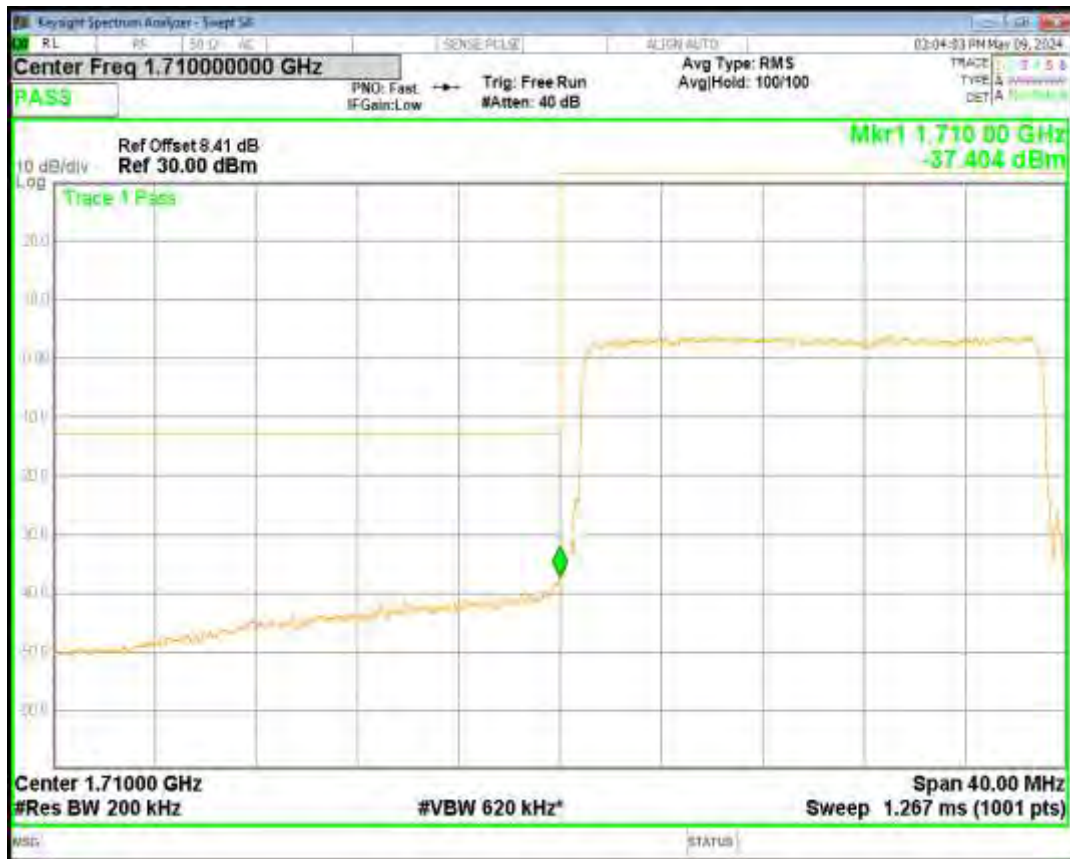
Band4 QPSK BW=15MHz Channel=20325 RB Size=75 Position=#0
