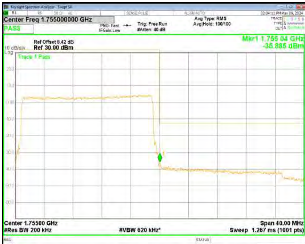
Band4 QPSK BW=20MHz Channel=20050 RB Size=100 Position=#0
