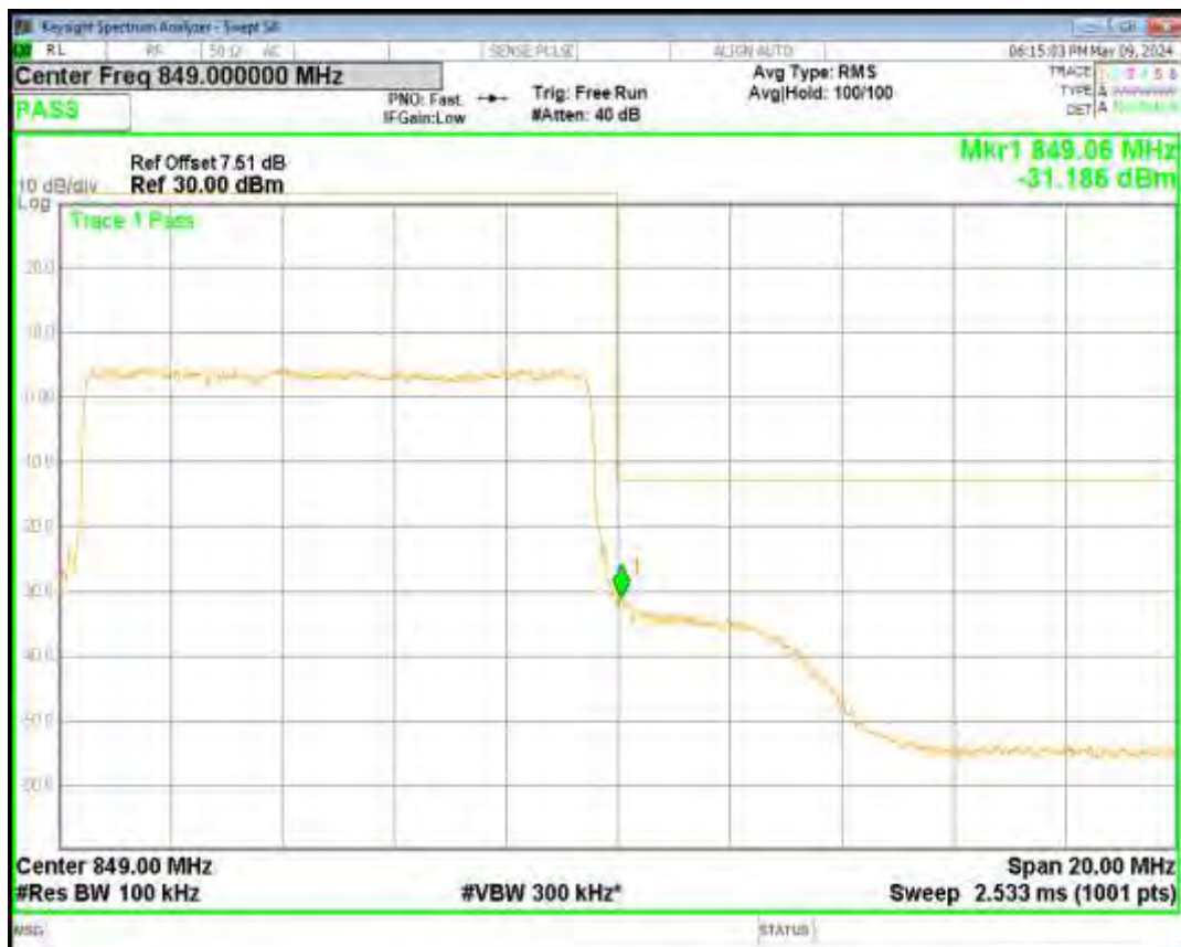
Band5 QPSK BW=3MHz Channel=20415 RB Size=15 Position=#0
