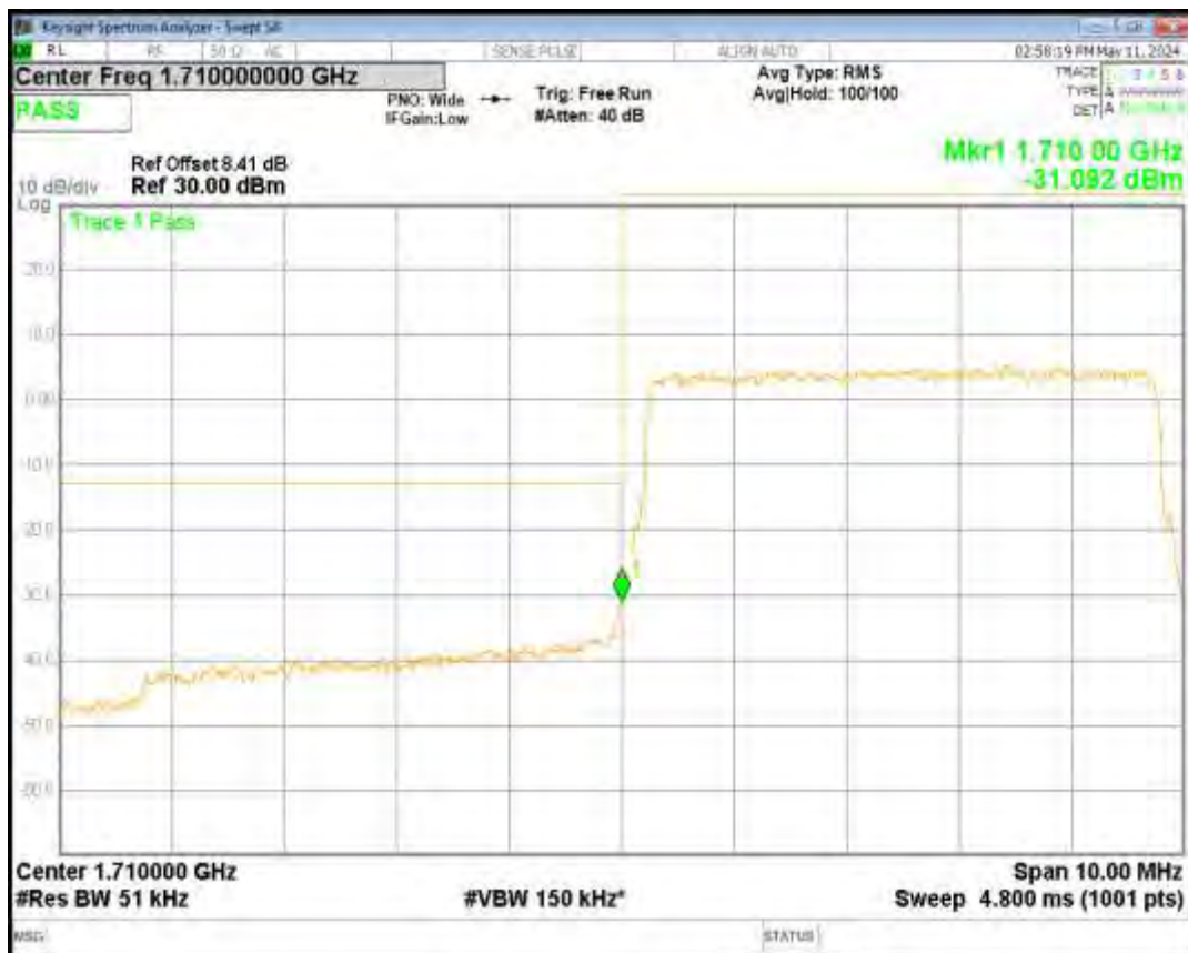
Band66 QPSK BW=10MHz Channel=132622 RB Size=50 Position=#0
