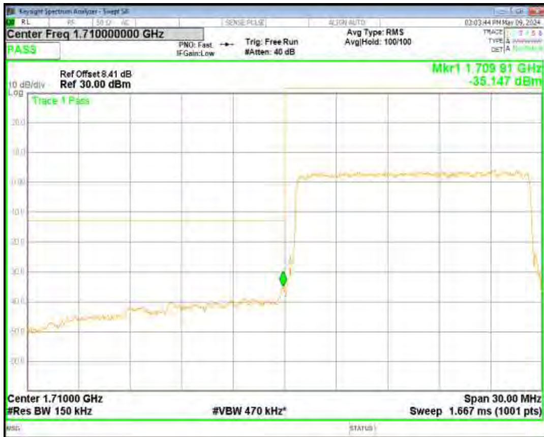
Band4 16QAM BW=5MHz Channel=20375 RB Size=25 Position=#0
