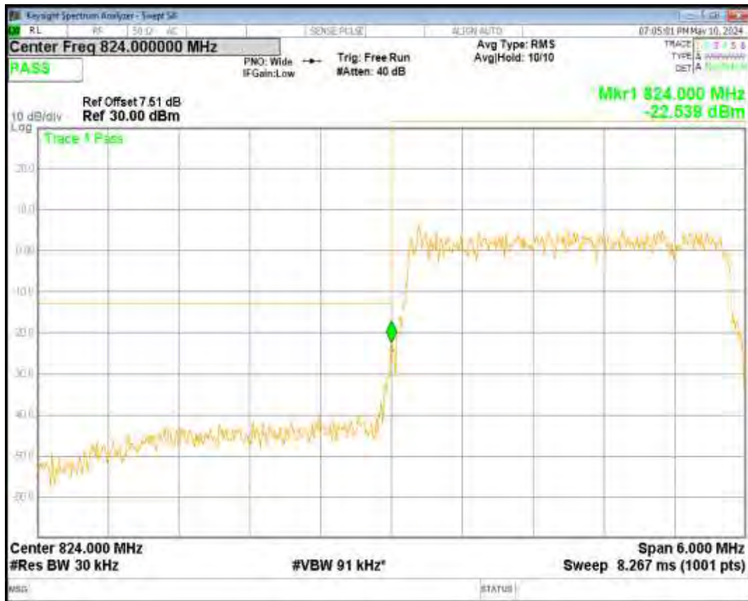
Band26(824-849) QPSK BW=3MHz Channel=27025 RB Size=15 Position=#0
