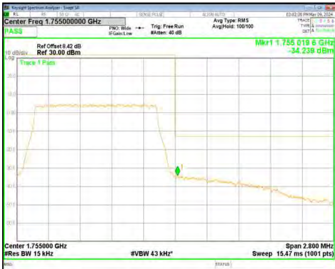
Band4 QPSK BW=1.4MHz Channel=19957 RB Size=6 Position=#0
