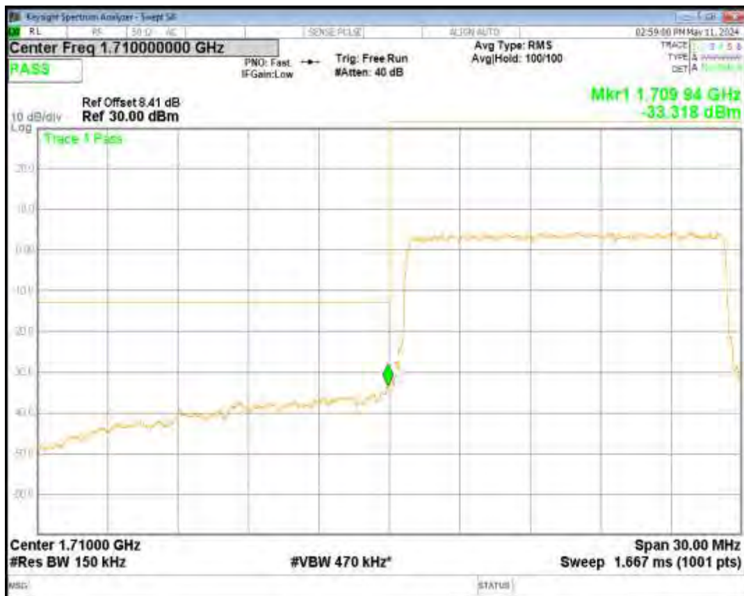
Band66 QPSK BW=15MHz Channel=132597 RB Size=75 Position=#0
