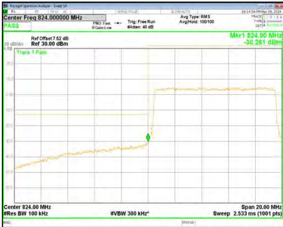
Band5 QPSK BW=10MHz Channel=20600 RB Size=50 Position=#0
