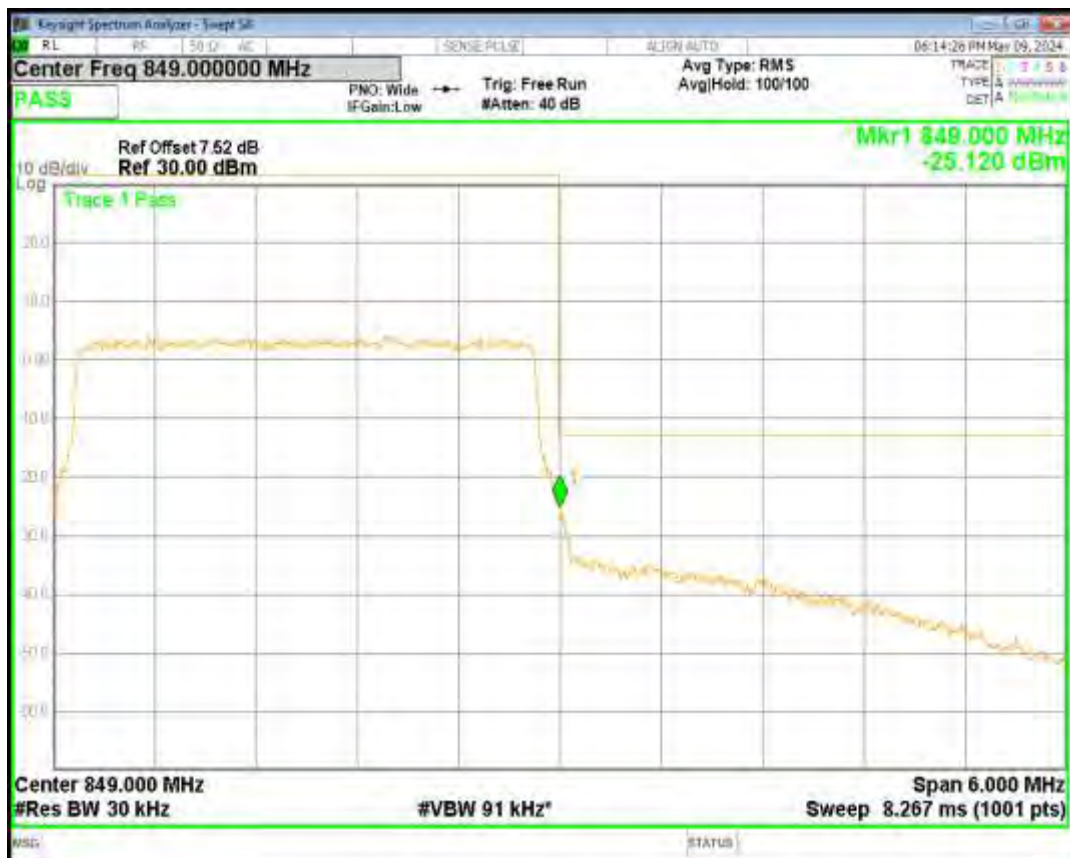
Band5 16QAM BW=5MHz Channel=20425 RB Size=25 Position=#0
