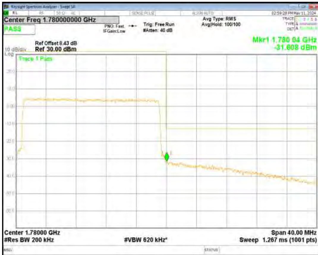
Band66 QPSK BW=3MHz Channel=131987 RB Size=15 Position=#0
