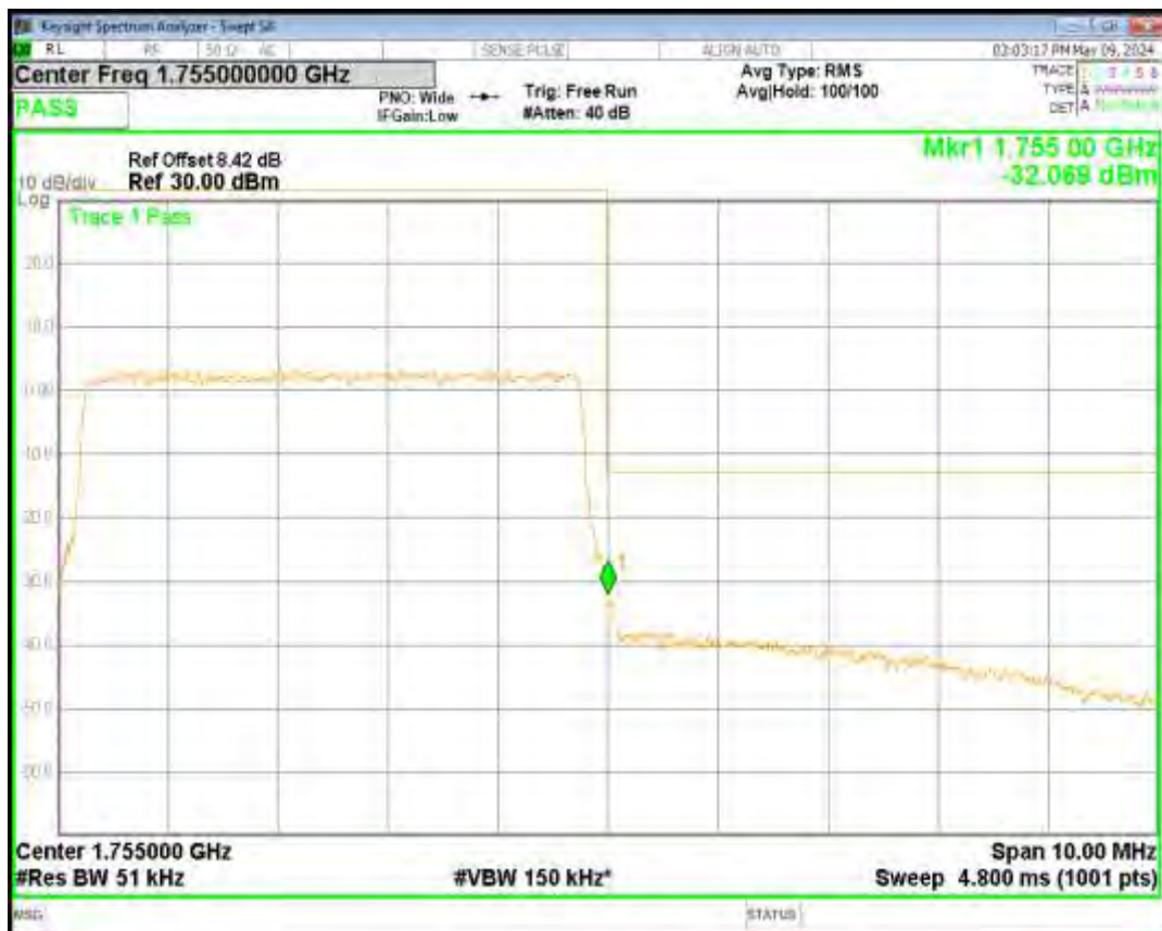
Band4 QPSK BW=10MHz Channel=20000 RB Size=50 Position=#0
