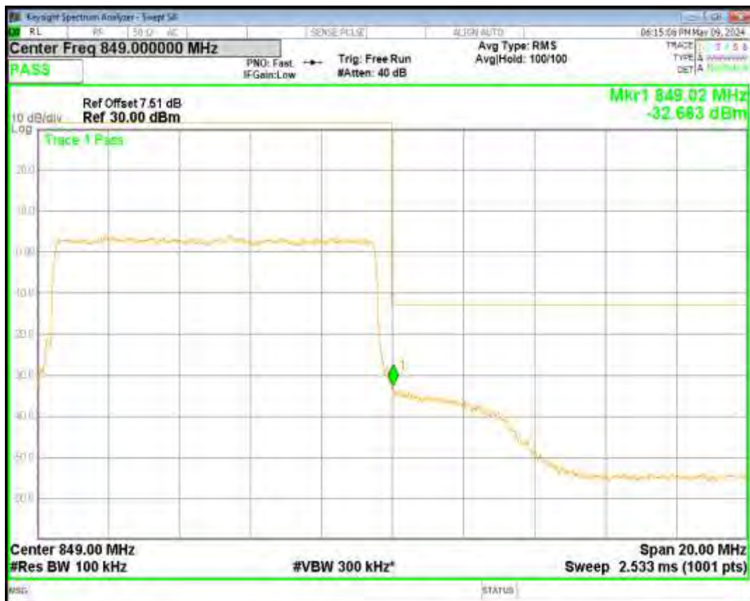
Band5 16QAM BW=3MHz Channel=20415 RB Size=15 Position=#0
