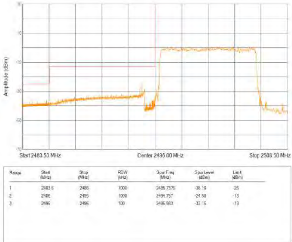
Band41 QPSK BW=10MHz Channel=41540 RB Size=50 Position=#0
