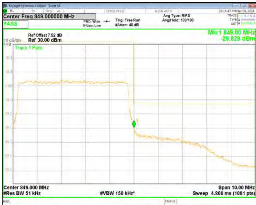
Band5 QPSK BW=1.4MHz Channel=20407 RB Size=6 Position=#0
