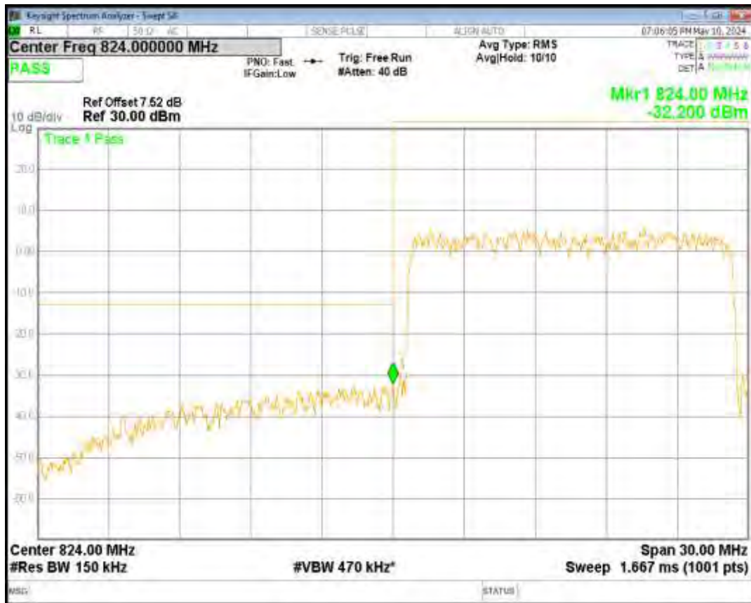
Band26(824-849) 16QAM BW=10MHz Channel=26990 RB Size=50 Position=#0
