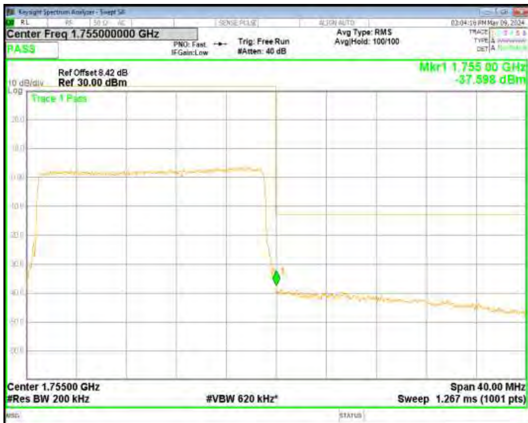
Band4 16QAM BW=3MHz Channel=19965 RB Size=15 Position=#0
