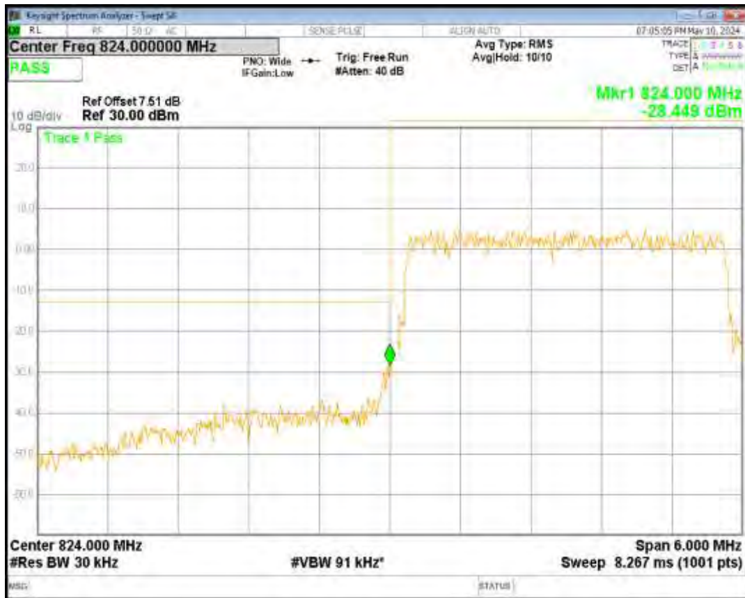
Band26(824-849) 16QAM BW=15MHz Channel=26965 RB Size=75 Position=#0
