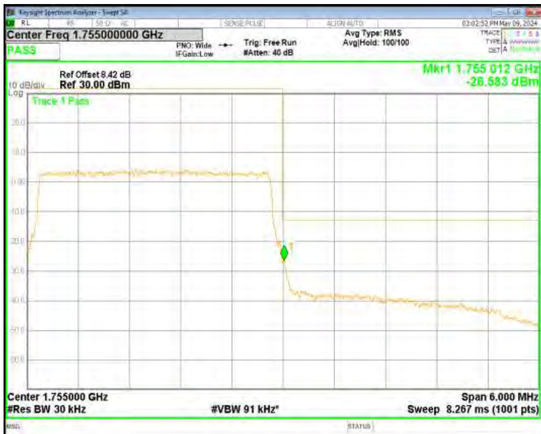
Band4 QPSK BW=3MHz Channel=19965 RB Size=15 Position=#0
