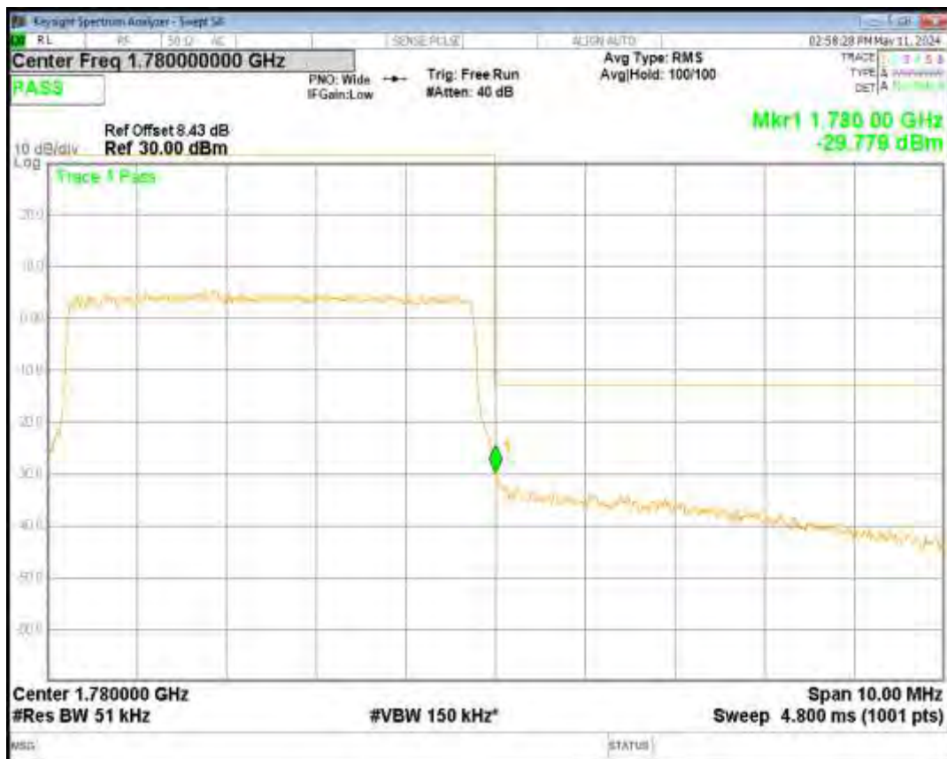
Band71 16QAM BW=10MHz Channel=133172 RB Size=50 Position=#0
