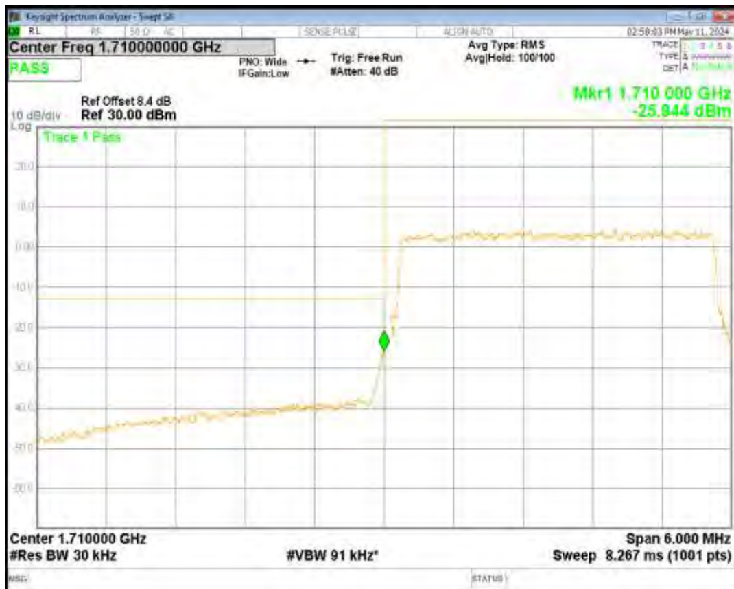
Band66 16QAM BW=5MHz Channel=132647 RB Size=25 Position=#0
