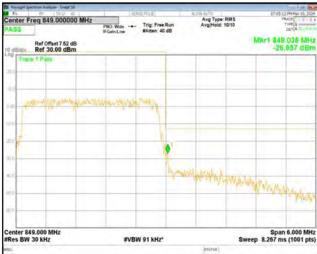
Band26(824-849) 16QAM BW=3MHz Channel=26805 RB Size=15 Position=#0
