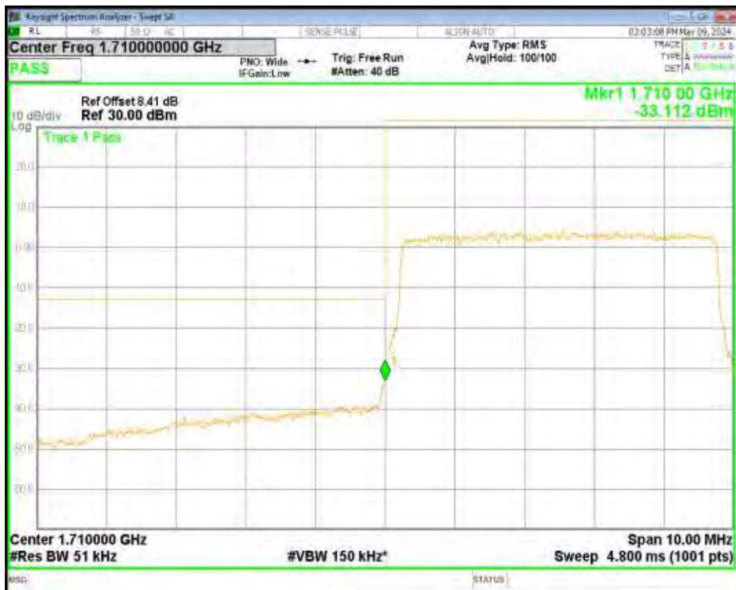
Band4 16QAM BW=3MHz Channel=20385 RB Size=15 Position=#0
