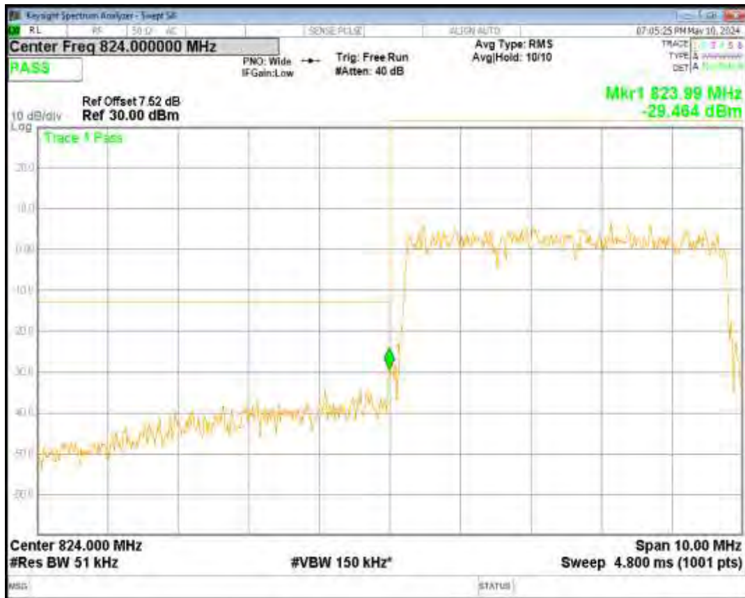
Band26(824-849) 16QAM BW=3MHz Channel=27025 RB Size=15 Position=#0
