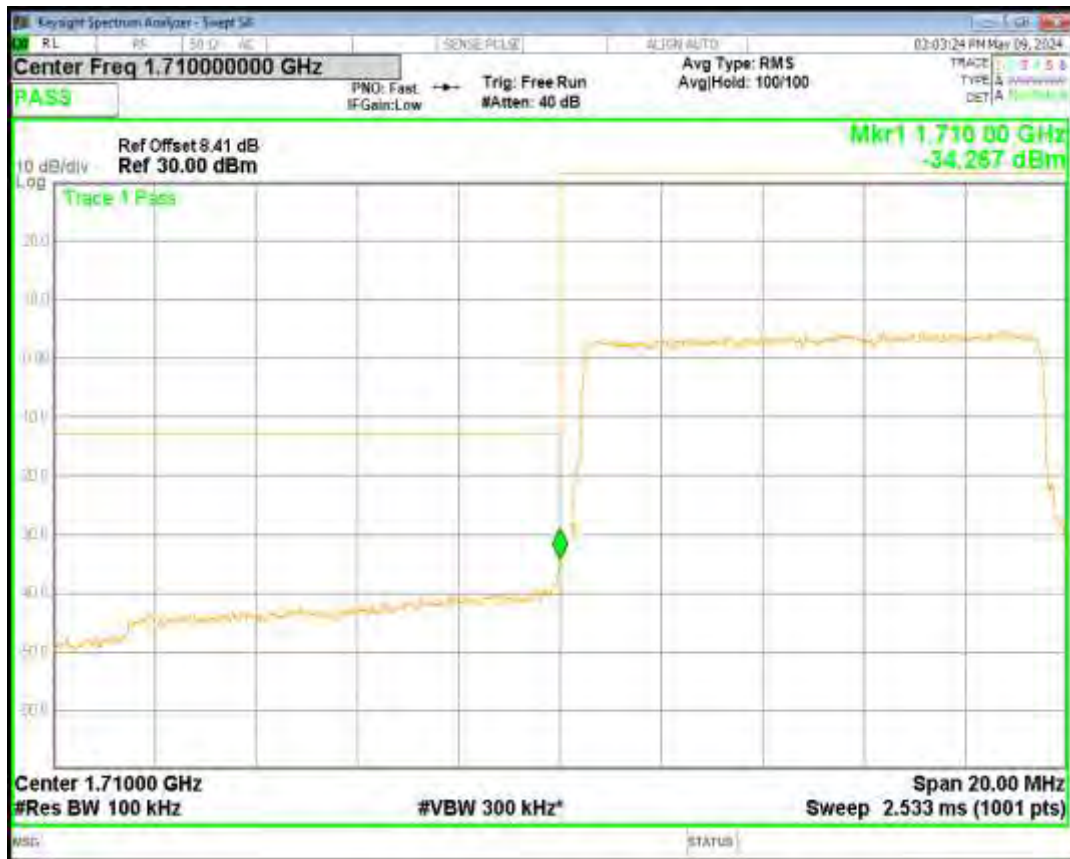
Band4 QPSK BW=1.4MHz Channel=20393 RB Size=6 Position=#0
