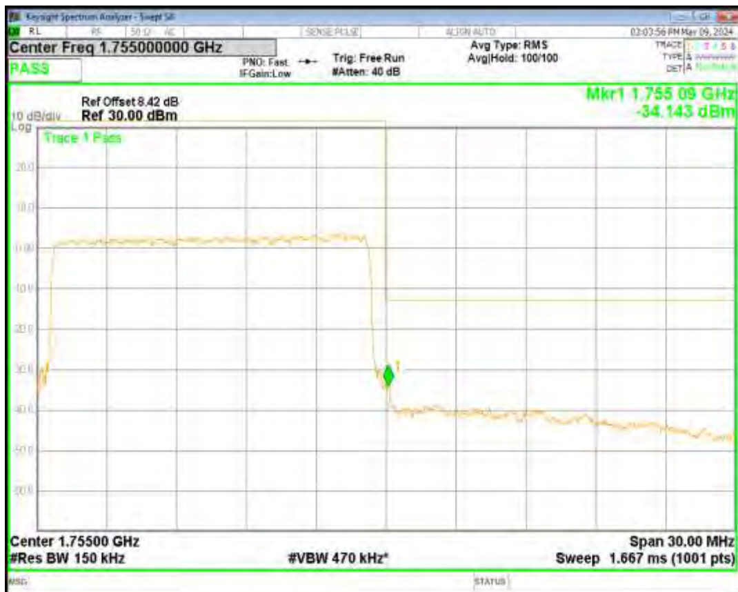
Band4 16QAM BW=20MHz Channel=20050 RB Size=100 Position=#0
