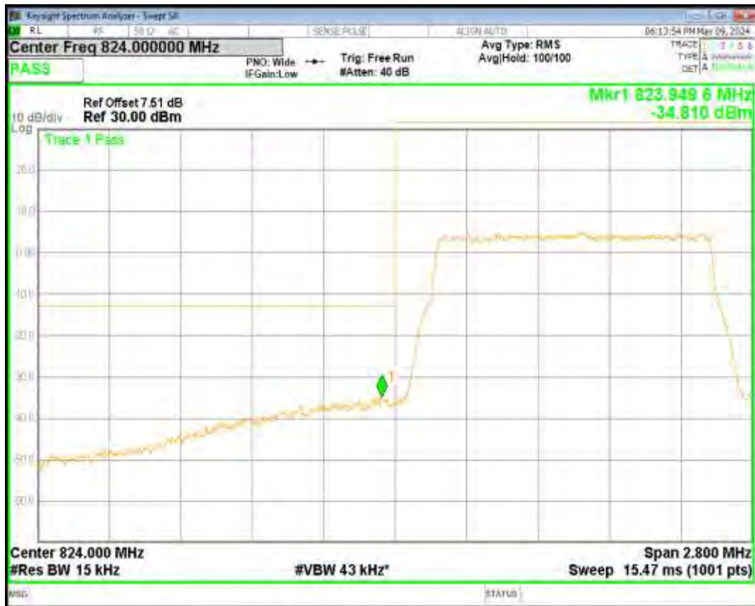
Band5 16QAM BW=1.4MHz Channel=20643 RB Size=6 Position=#0
