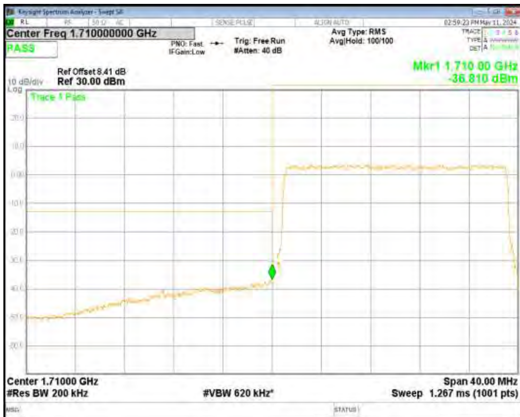
Band66 16QAM BW=15MHz Channel=132597 RB Size=75 Position=#0
