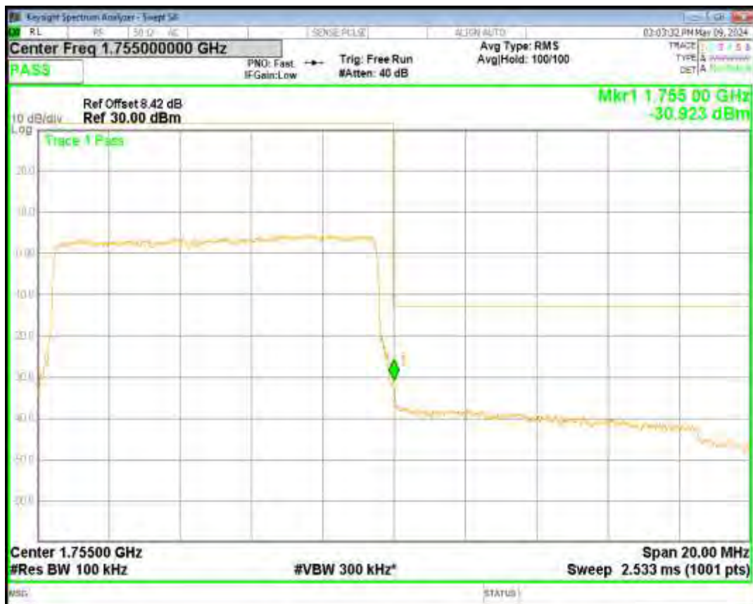
Band4 QPSK BW=5MHz Channel=19975 RB Size=25 Position=#0
