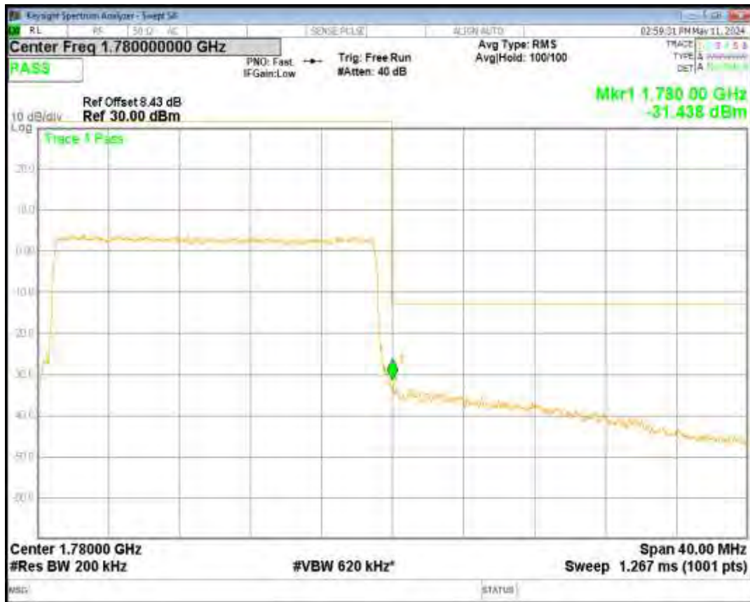
Band66 QPSK BW=5MHz Channel=131997 RB Size=25 Position=#0
