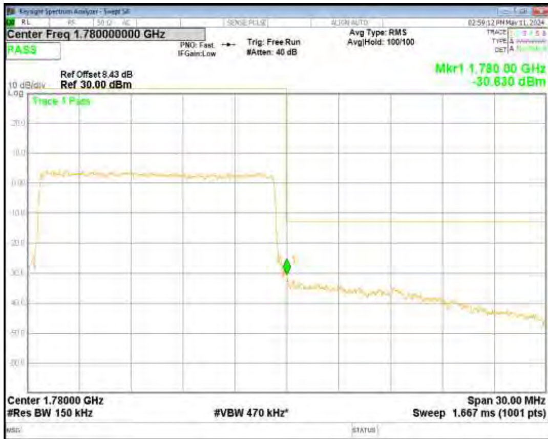
Band66 16QAM BW=15MHz Channel=132047 RB Size=75 Position=#0
