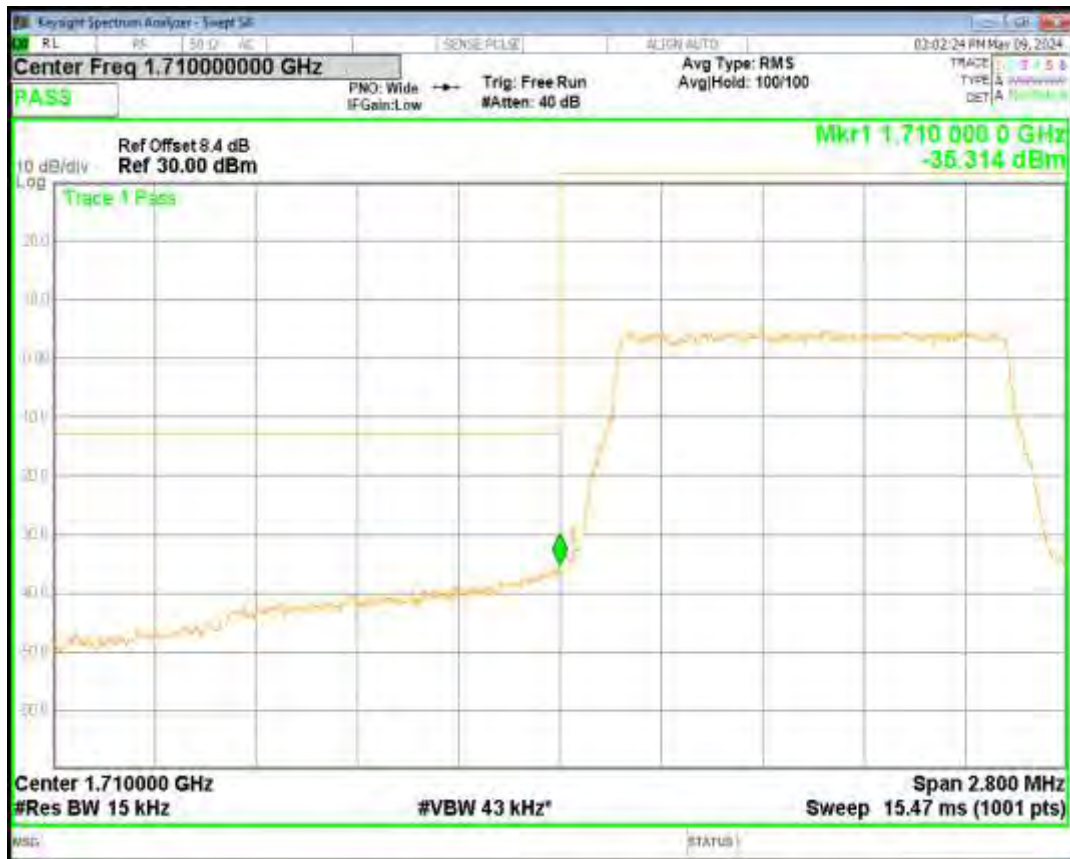
Band4 16QAM BW=1.4MHz Channel=20393 RB Size=6 Position=#0
