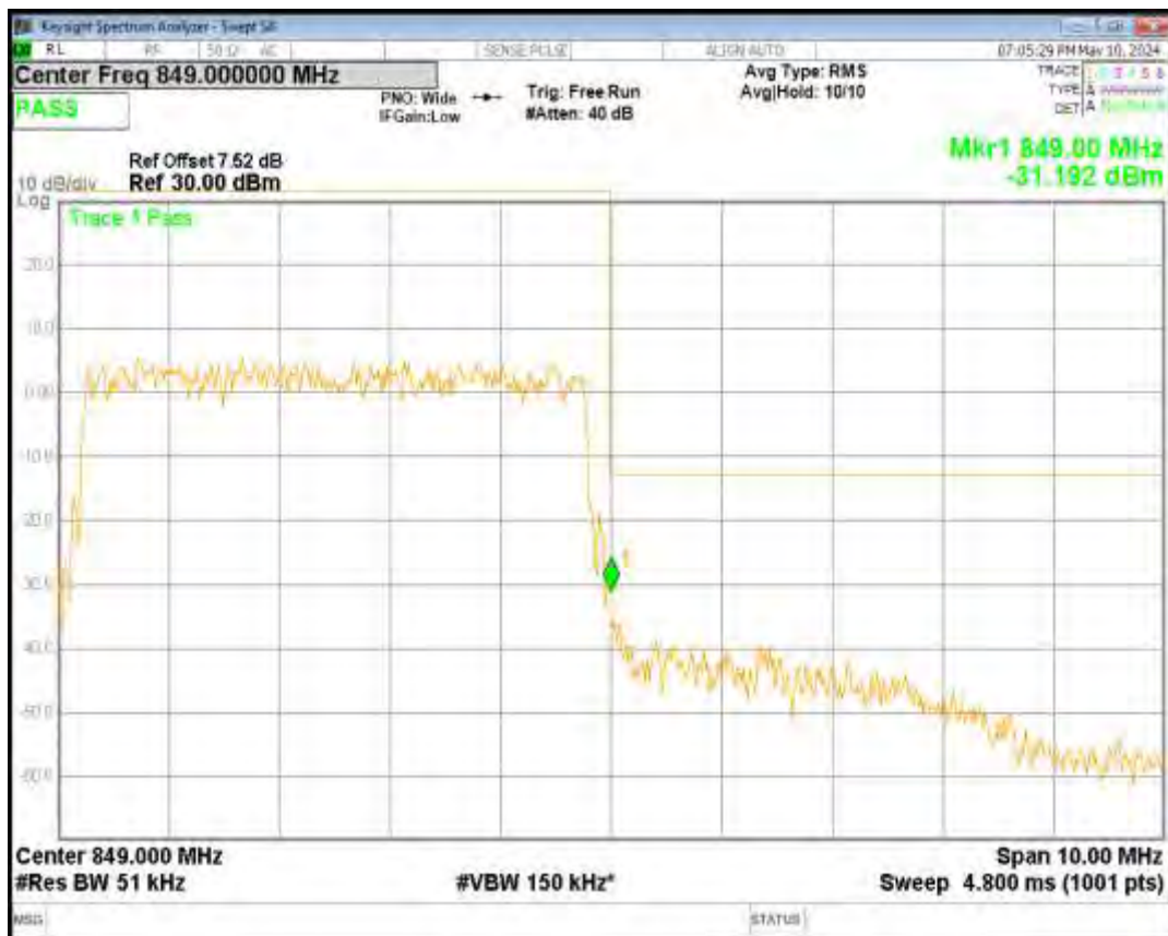
Band4 16QAM BW=1.4MHz Channel=19957 RB Size=6 Position=#0
