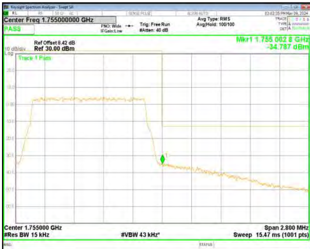
Band4 16QAM BW=10MHz Channel=20000 RB Size=50 Position=#0
