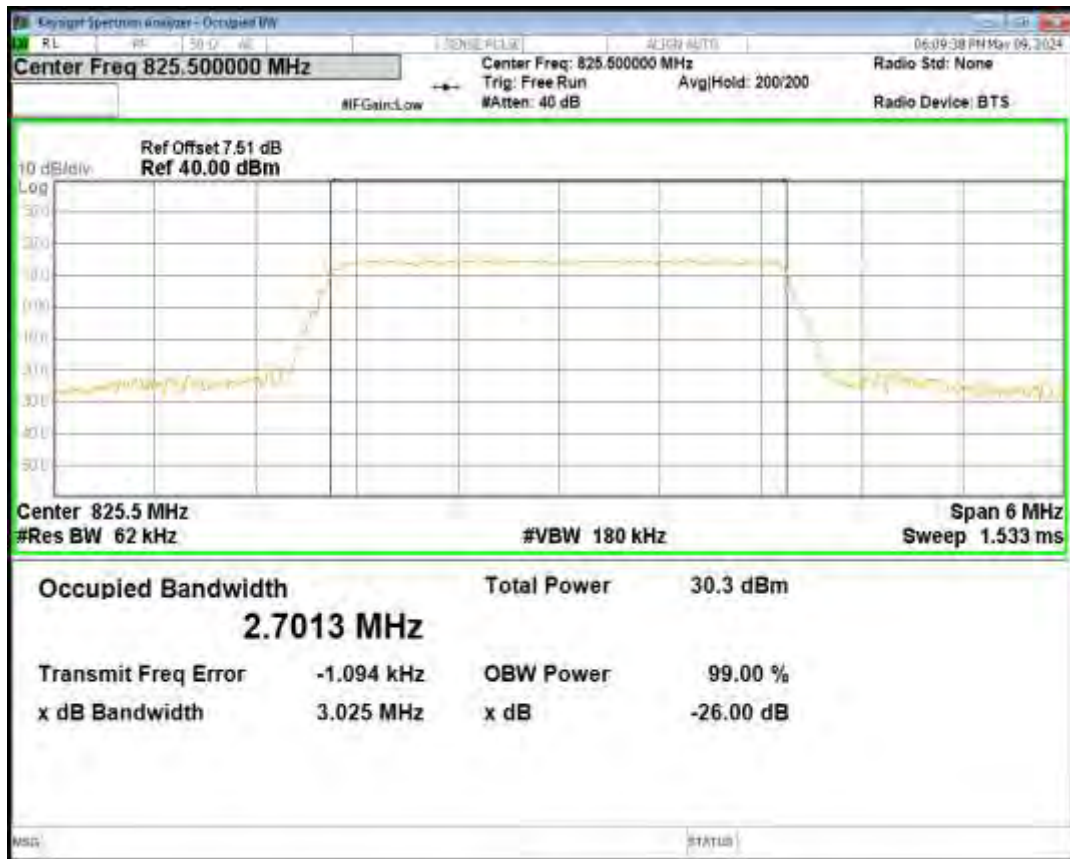
Band5 16QAM BW=3MHz Channel=20525 RB Size=15 Position=#0
