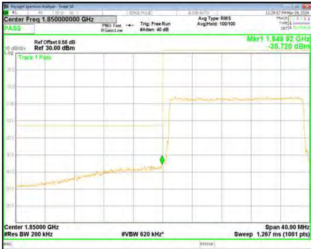
Band2 QPSK BW=1.4MHz Channel=19193 RB Size=6 Position=#0
