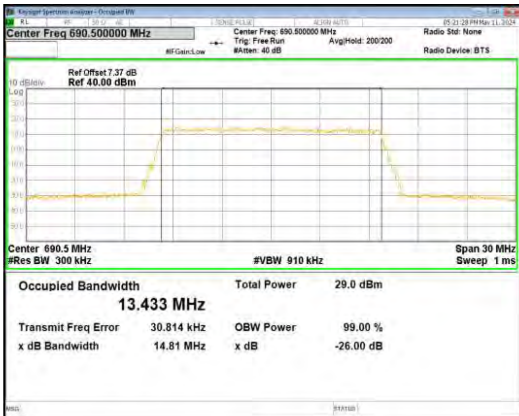
Band71 16QAM BW=20MHz Channel=133222 RB Size=100 Position=#0
