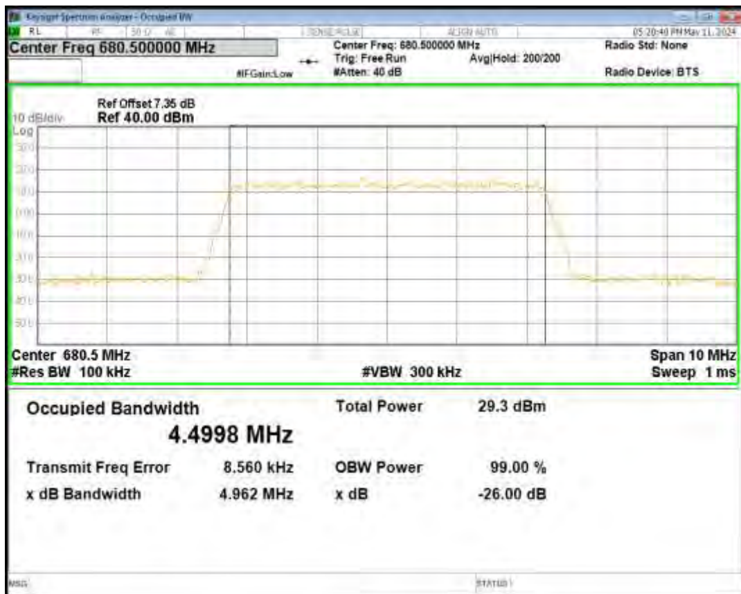
Band71 QPSK BW=15MHz Channel=133197 RB Size=75 Position=#0
