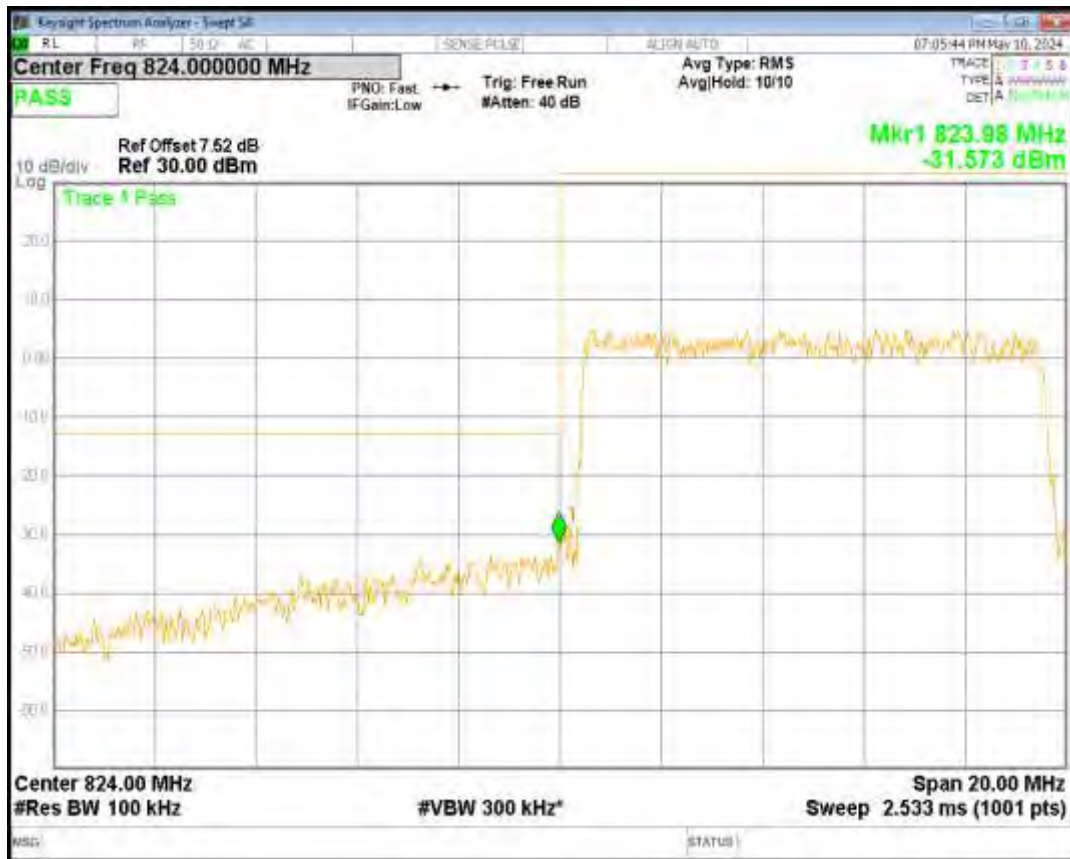
Band26(824-849) QPSK BW=15MHz Channel=26965 RB Size=75 Position=#0
