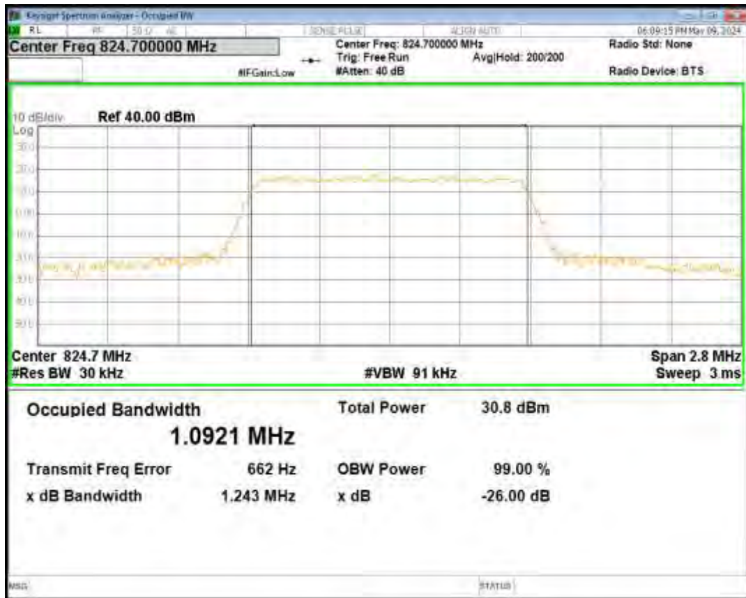
Band5 16QAM BW=5MHz Channel=20625 RB Size=25 Position=#0
