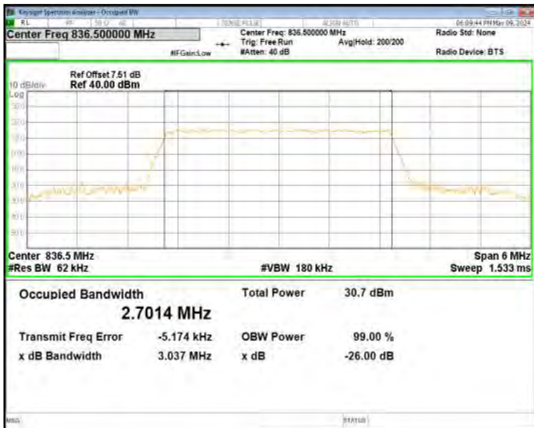
Band5 16QAM BW=3MHz Channel=20635 RB Size=15 Position=#0
