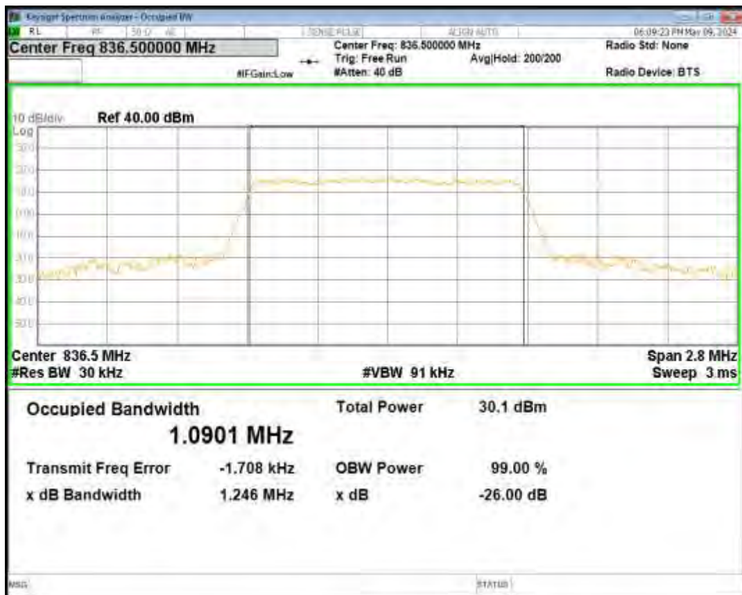
Band5 16QAM BW=1.4MHz Channel=20643 RB Size=6 Position=#0
