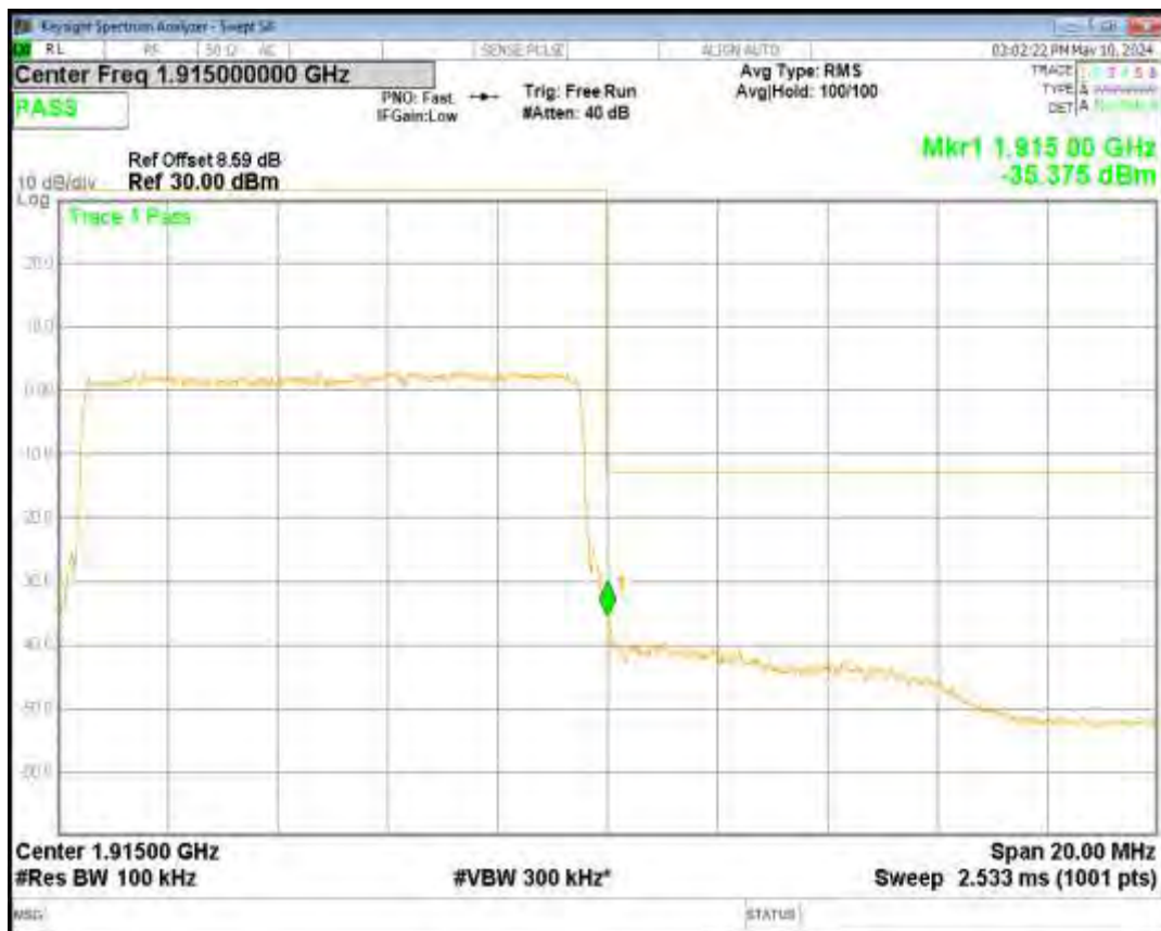
Band25 16QAM BW=15MHz Channel=26115 RB Size=75 Position=#0
