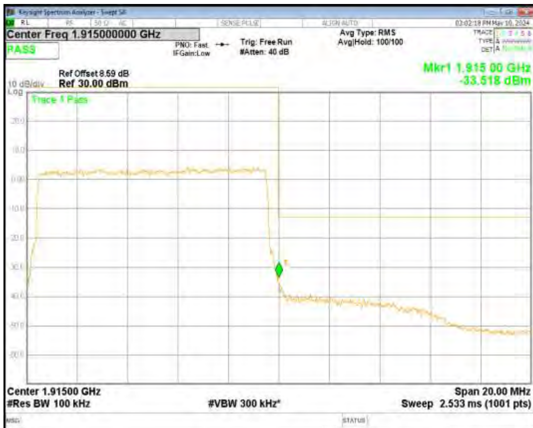
Band25 QPSK BW=5MHz Channel=26065 RB Size=25 Position=#0
