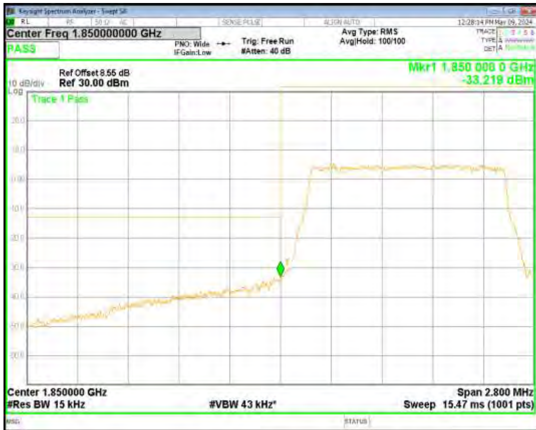
Band2 16QAM BW=1.4MHz Channel=19193 RB Size=6 Position=#0
