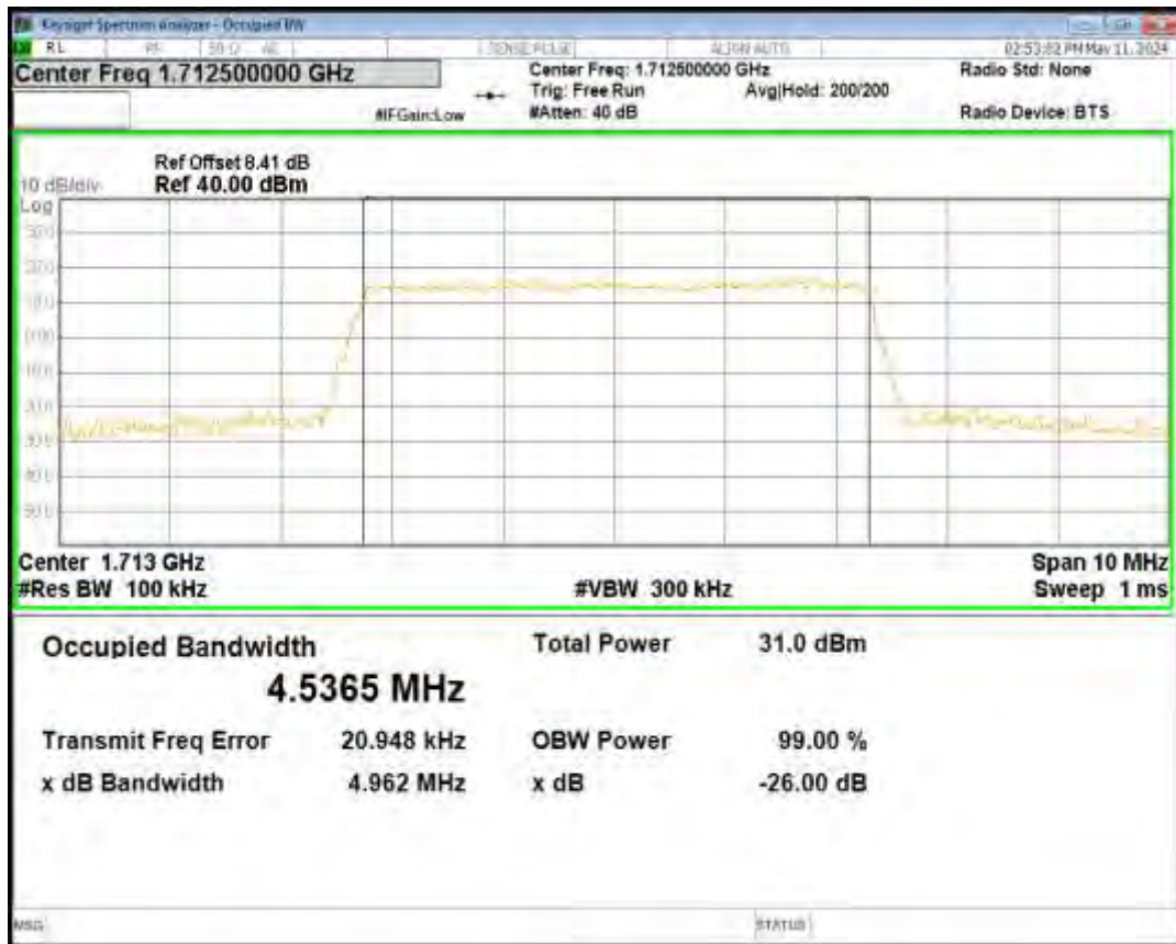
Band66 QPSK BW=5MHz Channel=132647 RB Size=25 Position=#0
