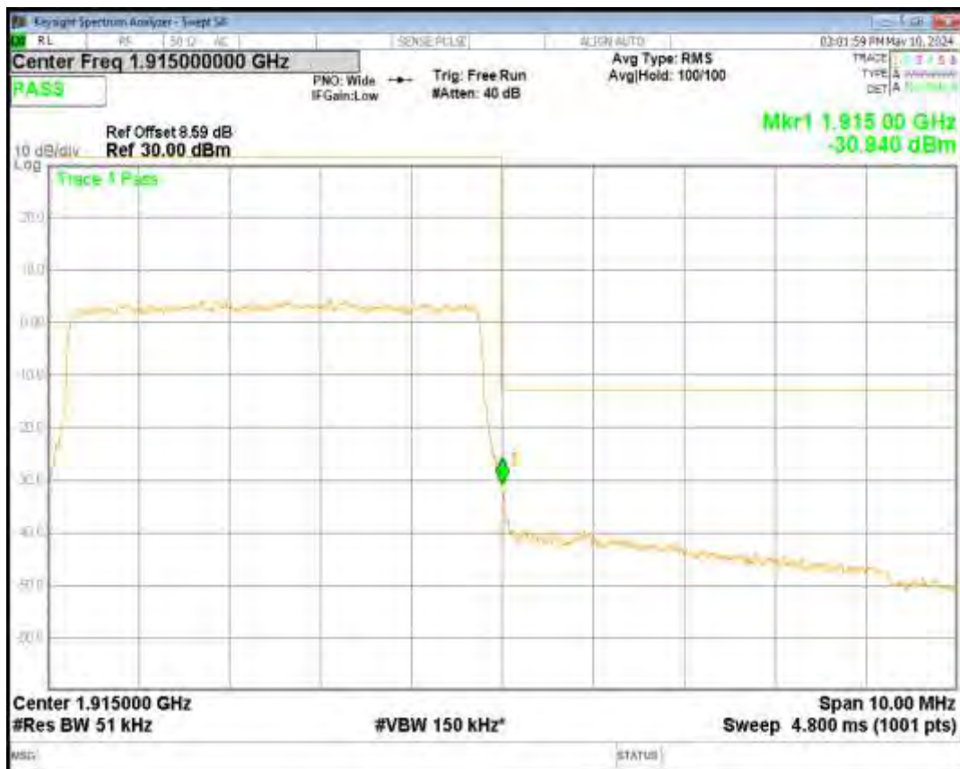
Band26(814-824) 16QAM BW=1.4MHz Channel=26697 RB Size=6 Position=#0
