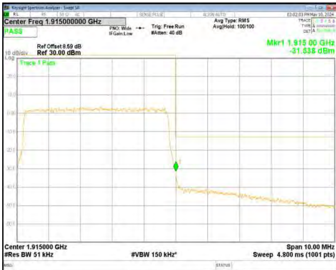
Band25 QPSK BW=10MHz Channel=26090 RB Size=50 Position=#0
