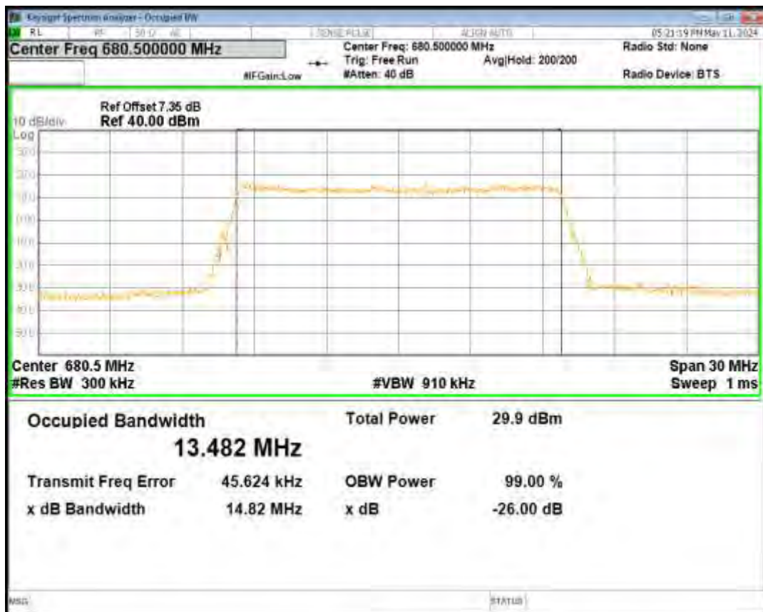
Band71 16QAM BW=5MHz Channel=133447 RB Size=25 Position=#0
