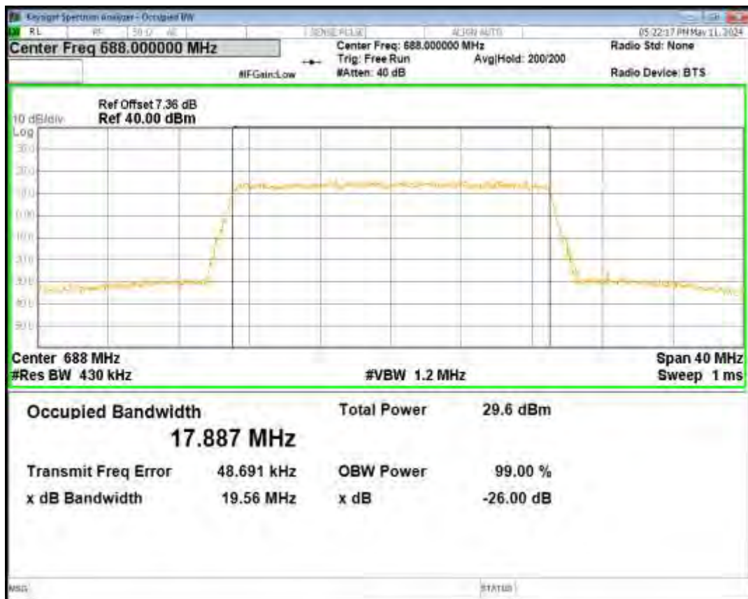
Band71 QPSK BW=20MHz Channel=133297 RB Size=100 Position=#0
