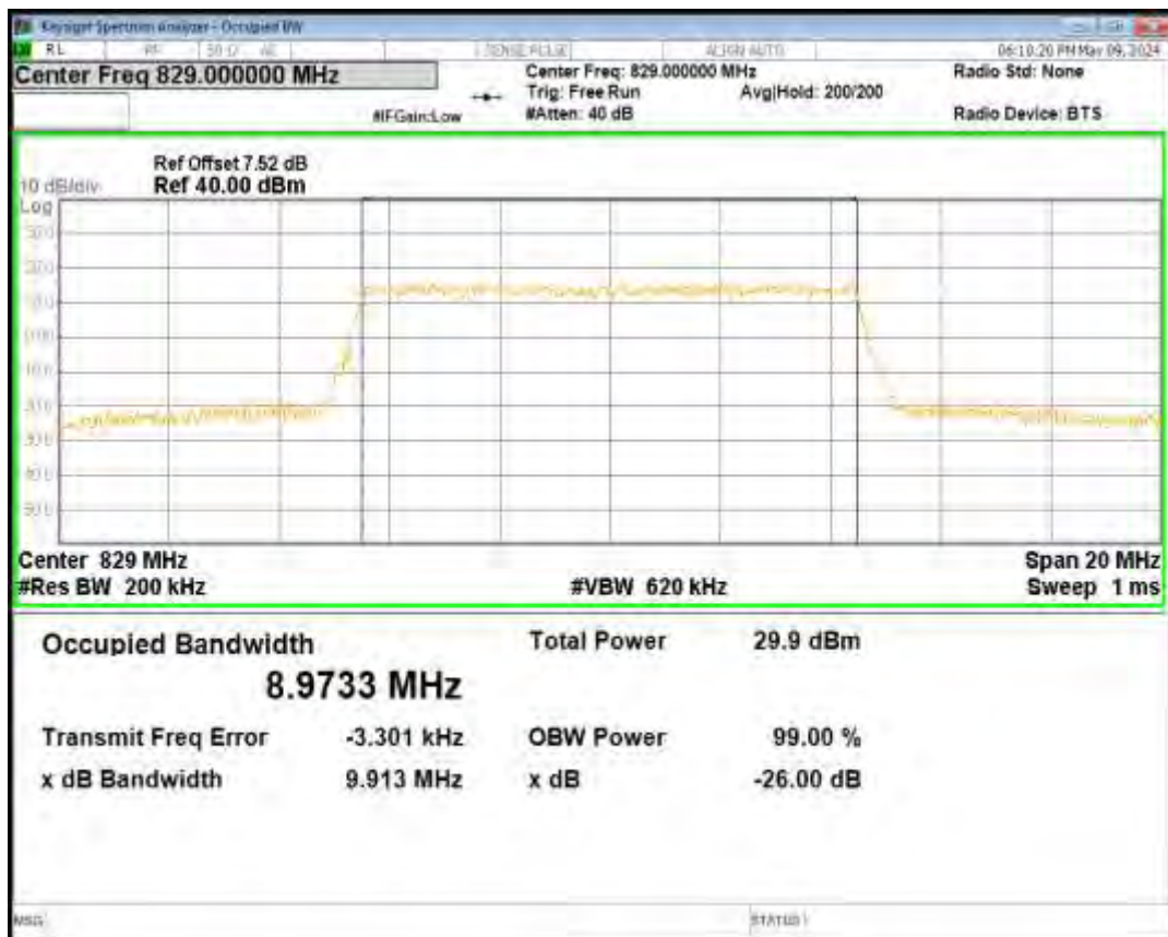
Band5 16QAM BW=10MHz Channel=20525 RB Size=50 Position=#0
