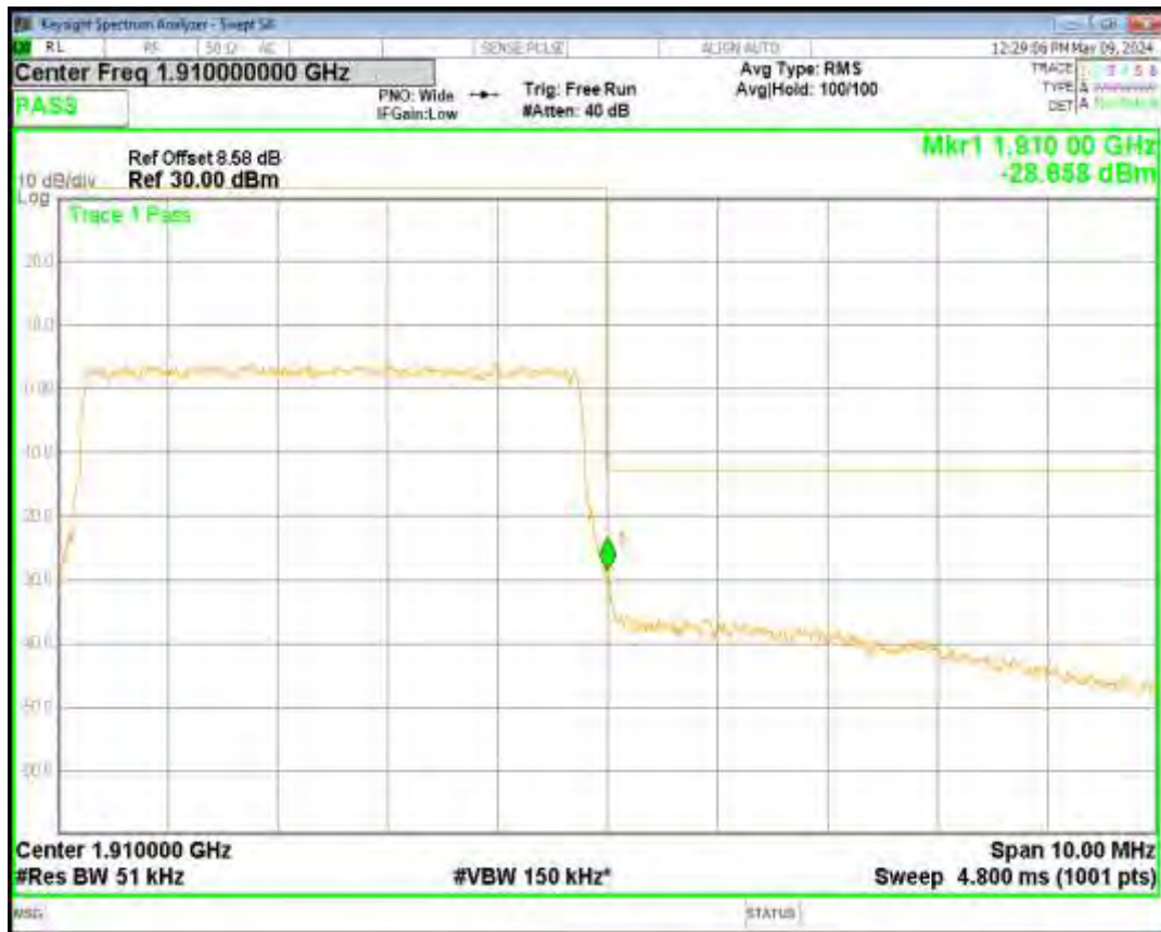
Band2 16QAM BW=3MHz Channel=18615 RB Size=15 Position=#0
