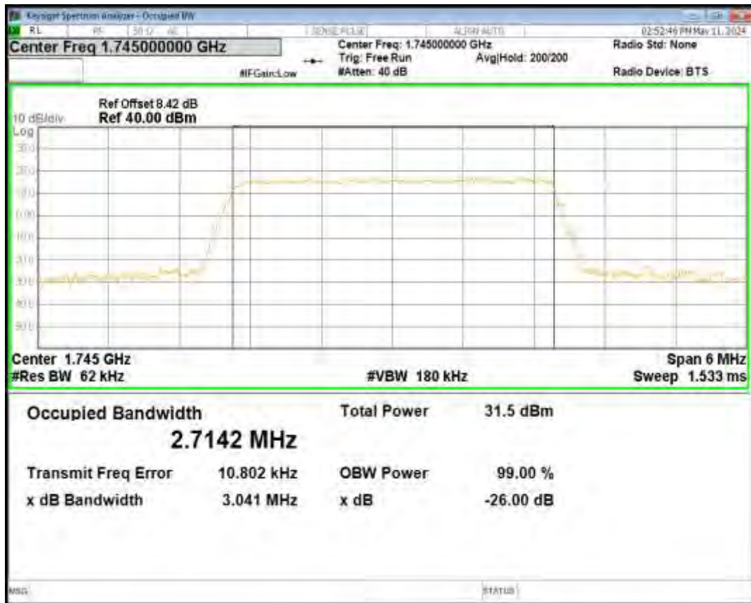
Band66 QPSK BW=3MHz Channel=132657 RB Size=15 Position=#0
