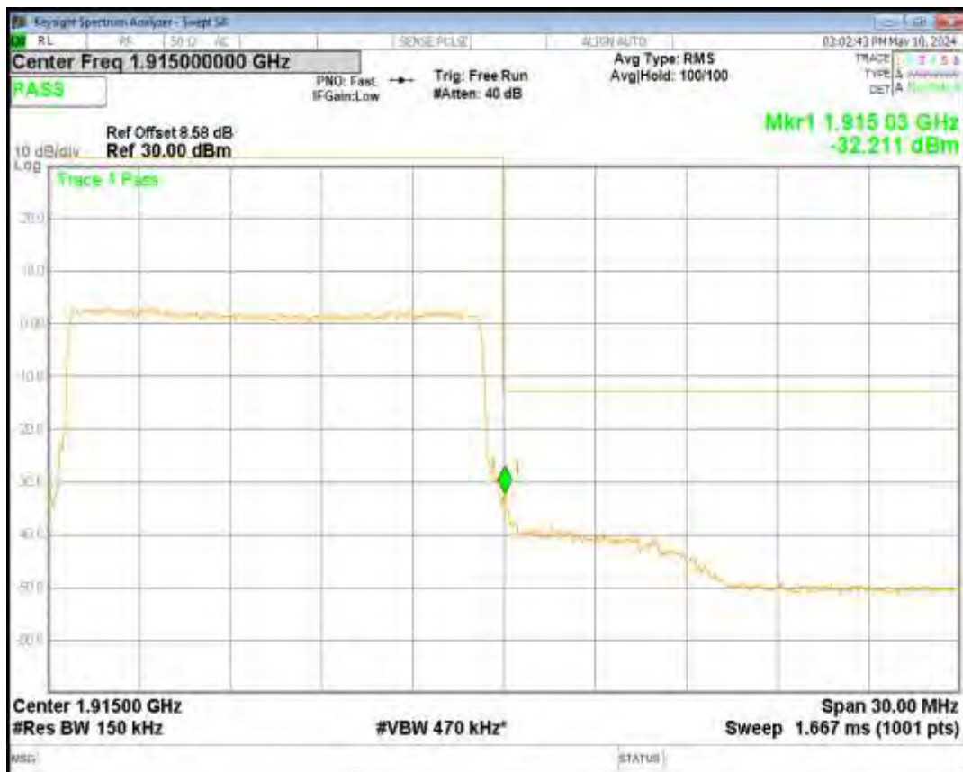
Band25 16QAM BW=20MHz Channel=26140 RB Size=100 Position=#0
