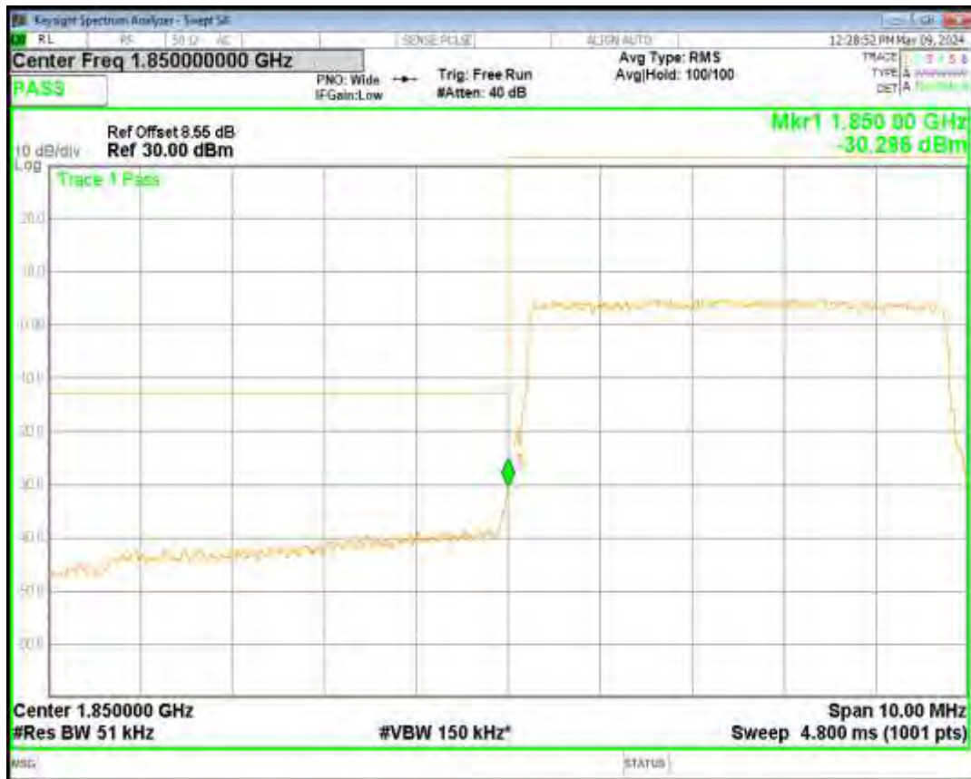
Band2 QPSK BW=15MHz Channel=18675 RB Size=75 Position=#0
