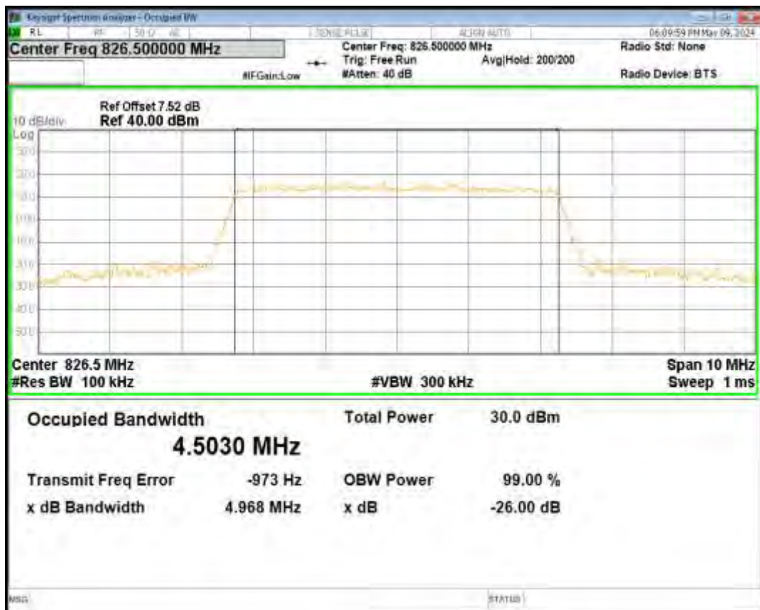
Band5 QPSK BW=1.4MHz Channel=20407 RB Size=6 Position=#0
