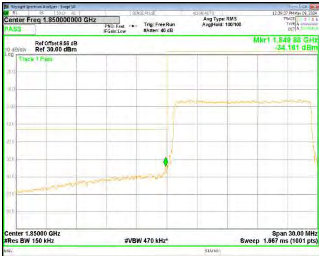
Band2 16QAM BW=15MHz Channel=19125 RB Size=75 Position=#0
