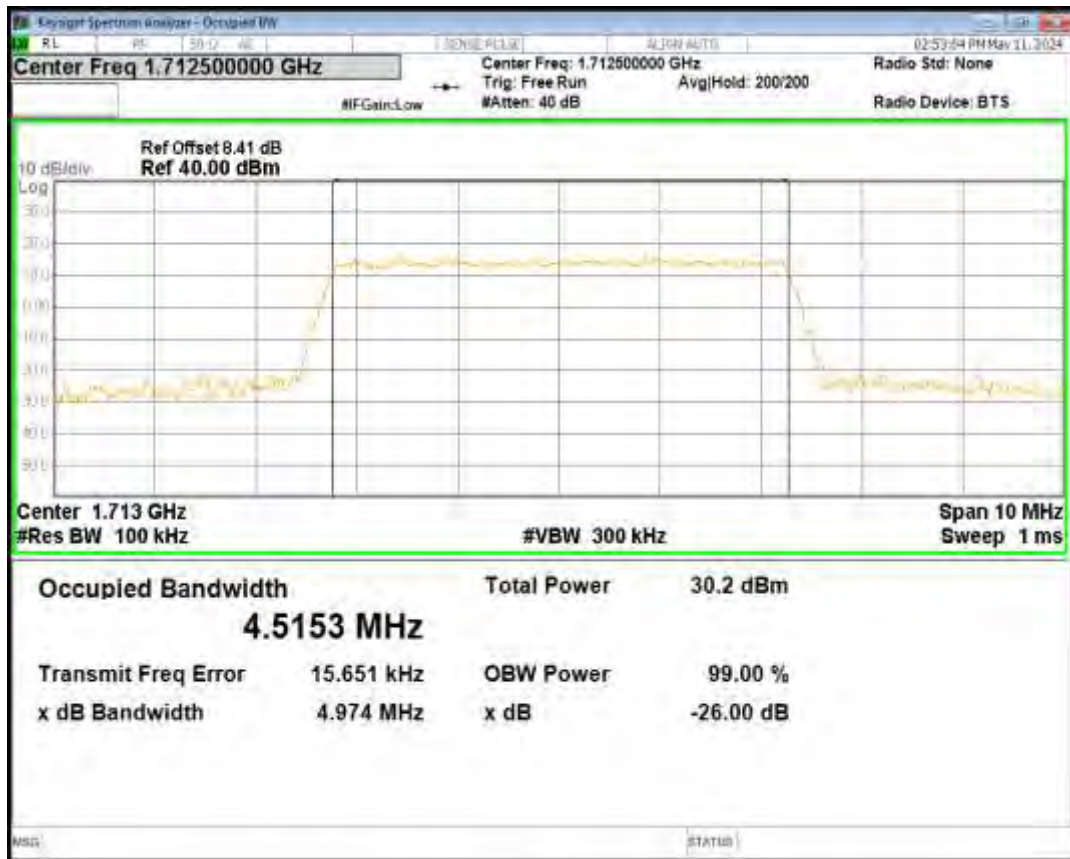
Band66 16QAM BW=3MHz Channel=132657 RB Size=15 Position=#0
