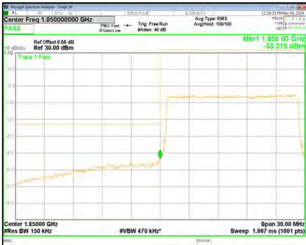
Band2 QPSK BW=15MHz Channel=19125 RB Size=75 Position=#0
