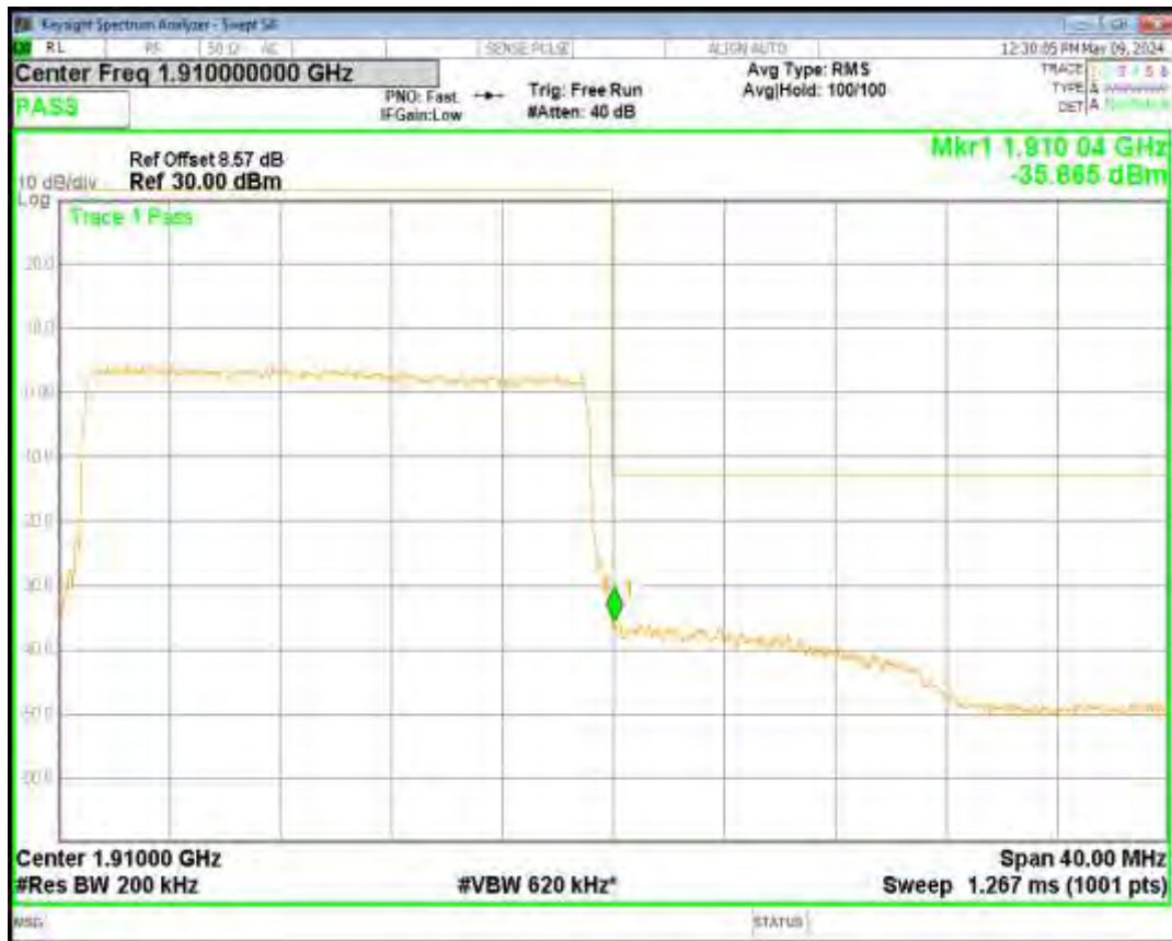
Band2 16QAM BW=3MHz Channel=19185 RB Size=15 Position=#0
