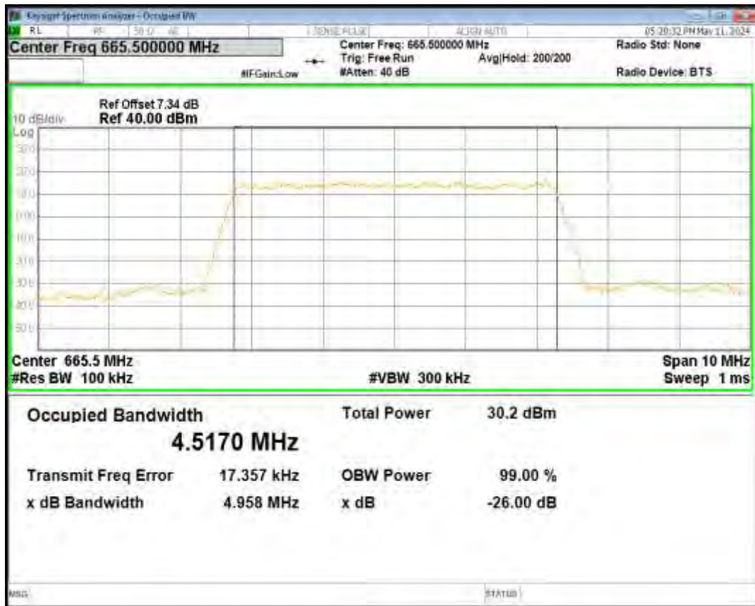
Band71 QPSK BW=20MHz Channel=133372 RB Size=100 Position=#0
