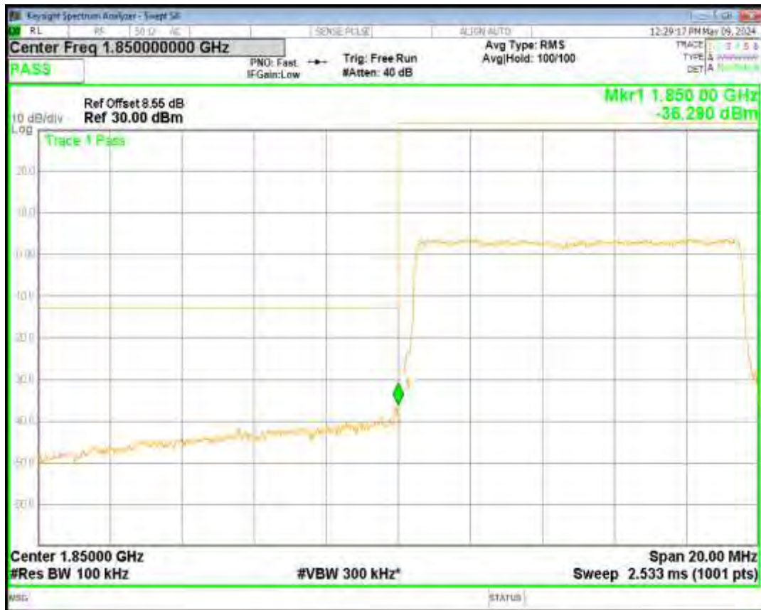
Band2 16QAM BW=10MHz Channel=19150 RB Size=50 Position=#0
