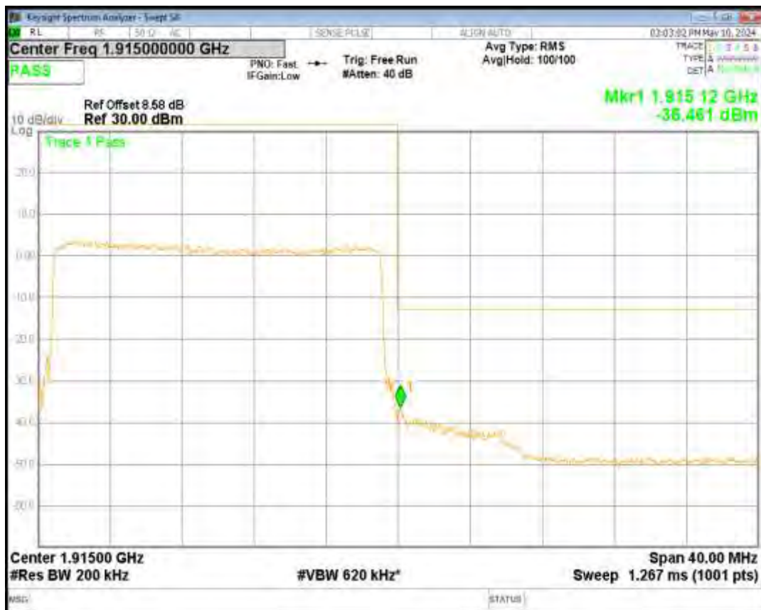
Band25 16QAM BW=3MHz Channel=26055 RB Size=15 Position=#0
