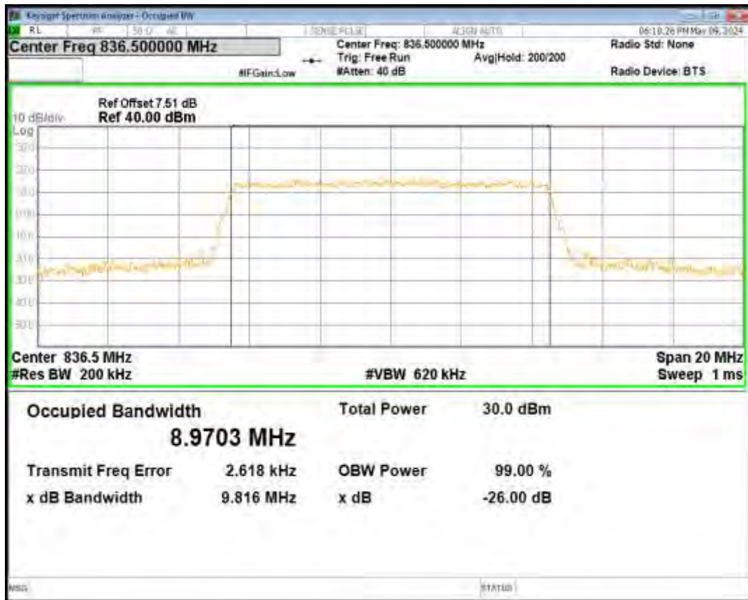
Band5 16QAM BW=10MHz Channel=20600 RB Size=50 Position=#0
