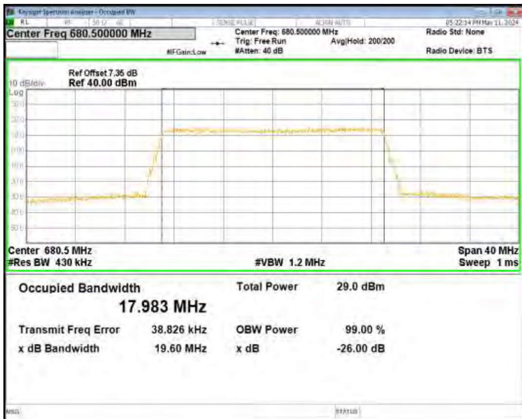
Band71 16QAM BW=20MHz Channel=133372 RB Size=100 Position=#0
