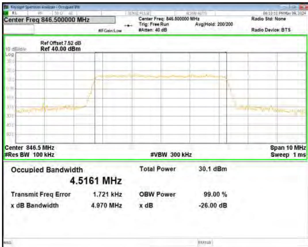
Band5 16QAM BW=5MHz Channel=20525 RB Size=25 Position=#0
