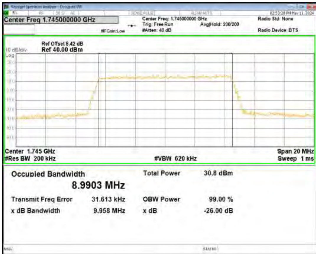
Band66 QPSK BW=5MHz Channel=132322 RB Size=25 Position=#0
