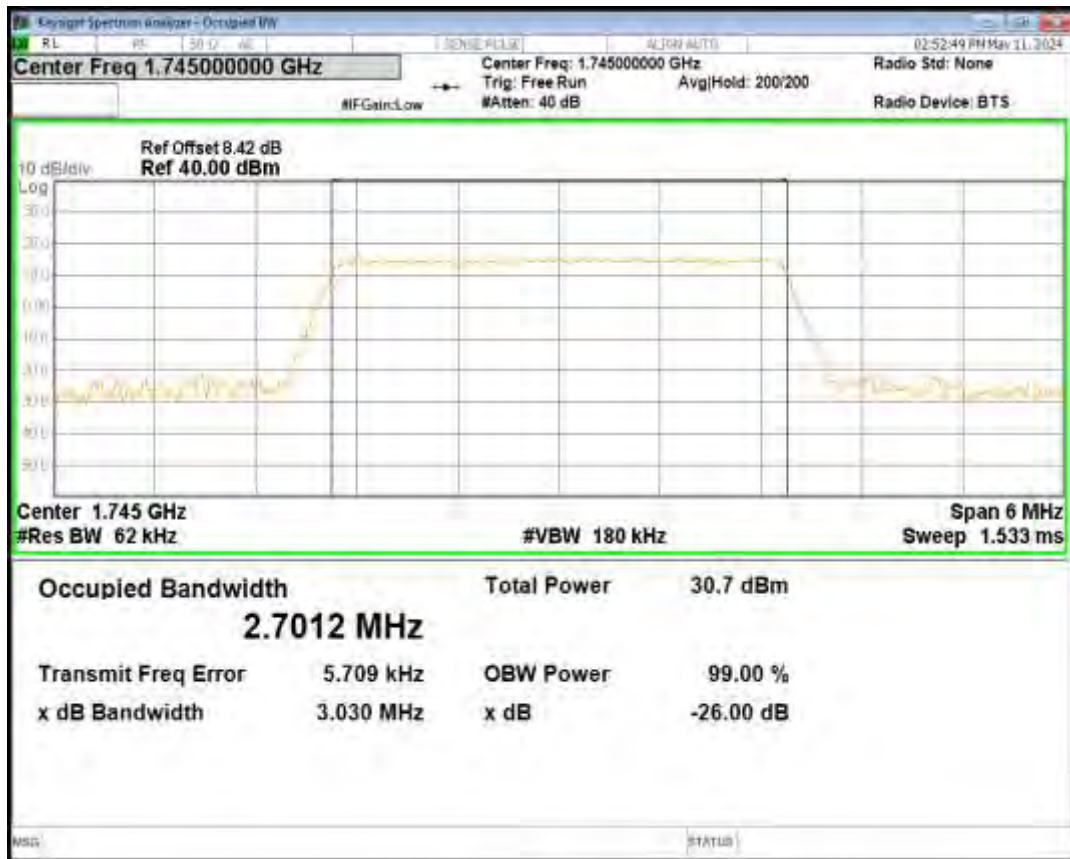
Band66 16QAM BW=3MHz Channel=131987 RB Size=15 Position=#0
