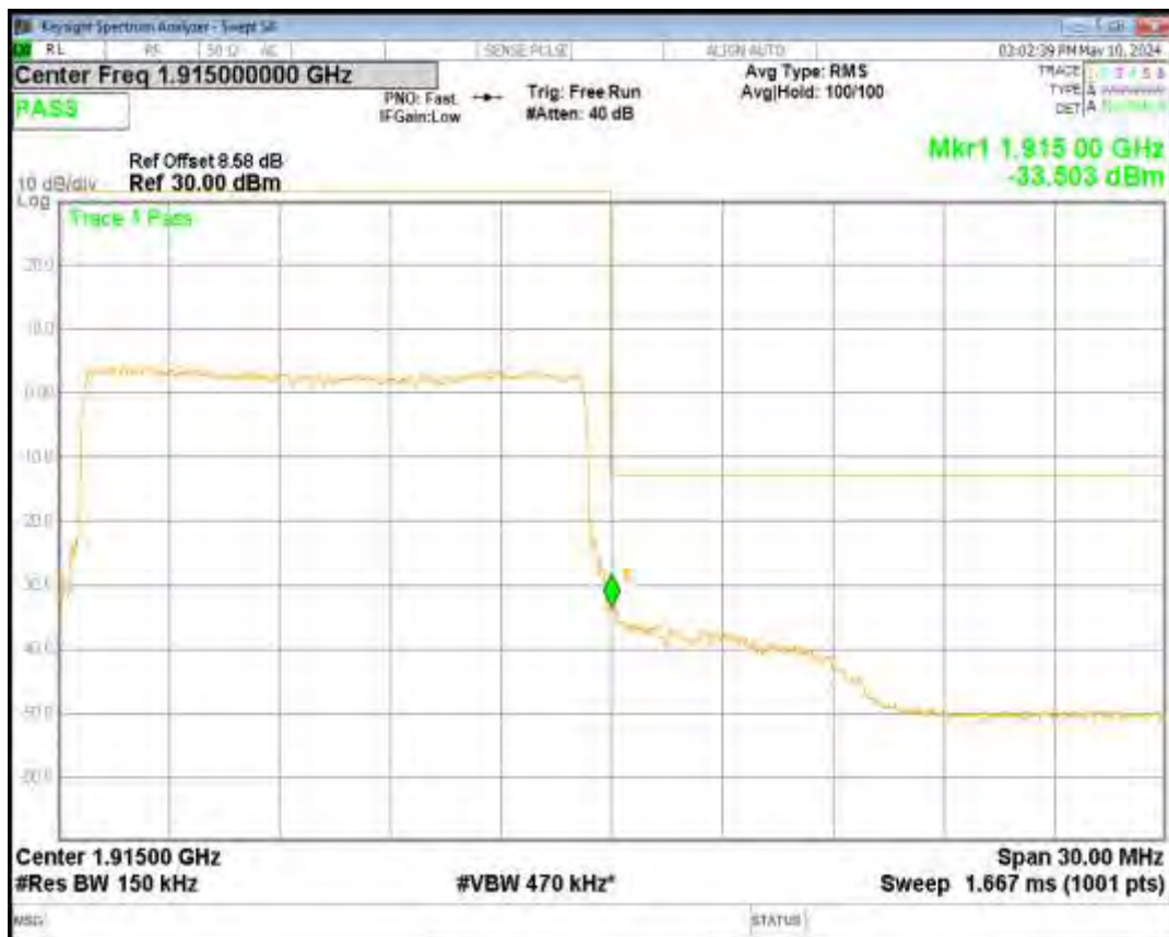
Band25 QPSK BW=15MHz Channel=26115 RB Size=75 Position=#0
