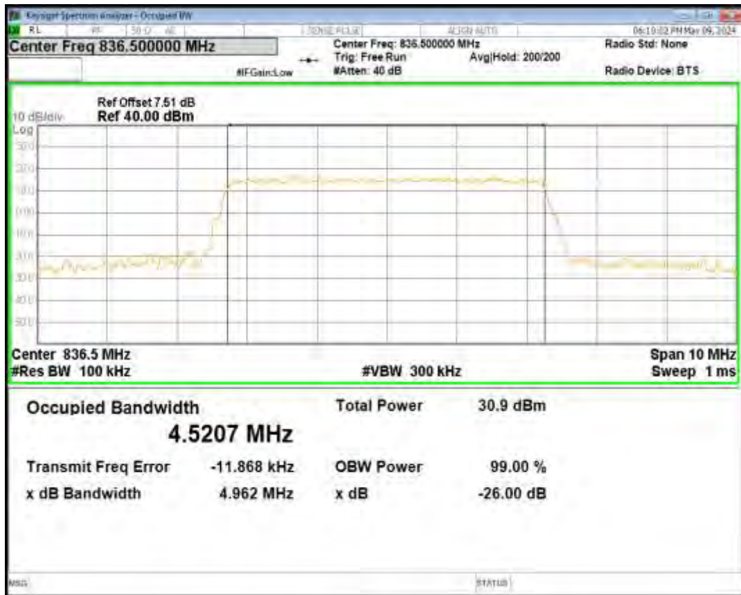
Band5 QPSK BW=5MHz Channel=20625 RB Size=25 Position=#0
