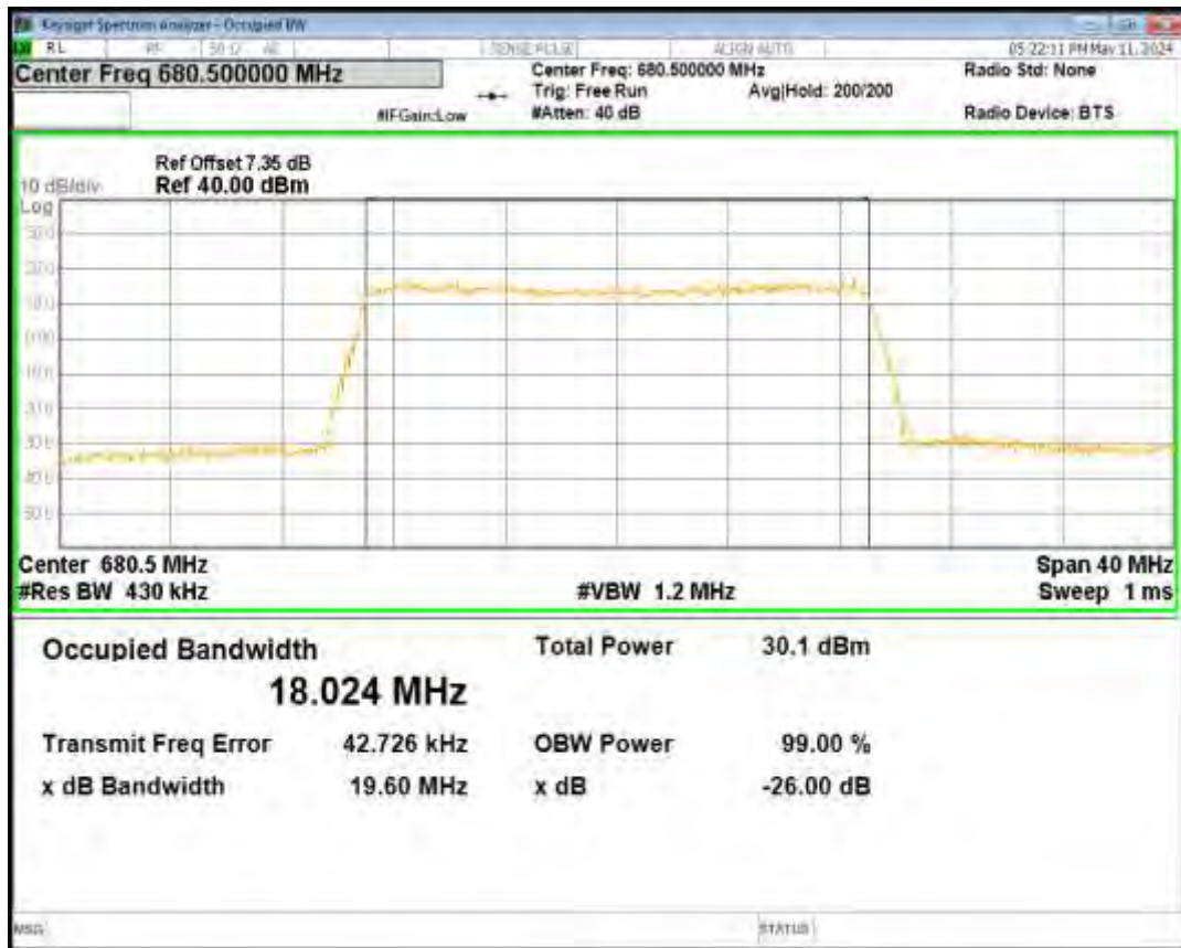
Band71 QPSK BW=20MHz Channel=133222 RB Size=100 Position=#0
