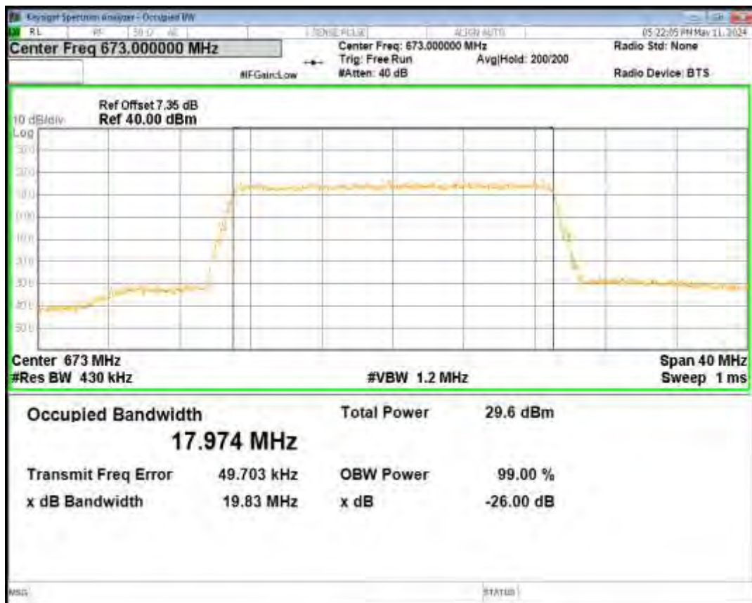
Band71 QPSK BW=15MHz Channel=133397 RB Size=75 Position=#0
