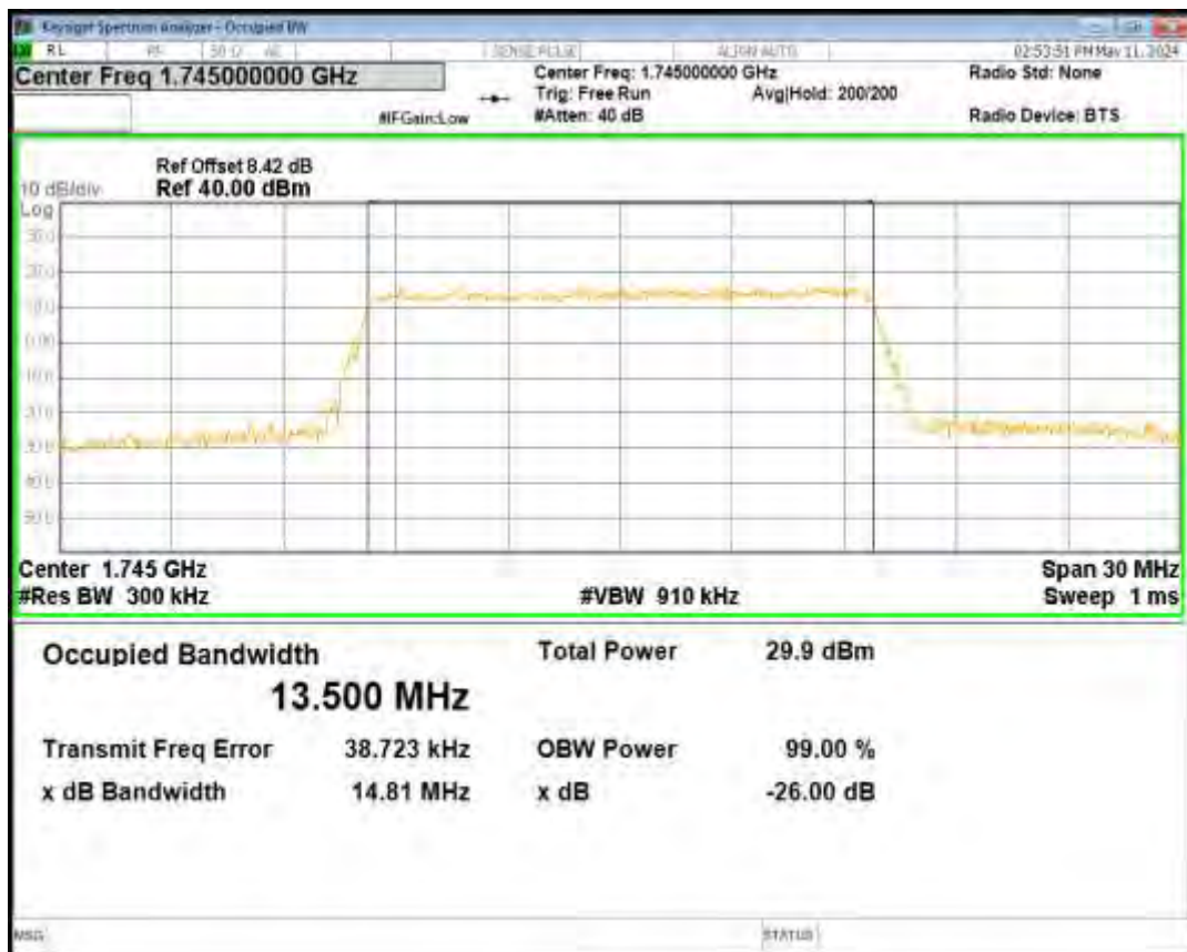
Band66 16QAM BW=15MHz Channel=132047 RB Size=75 Position=#0
