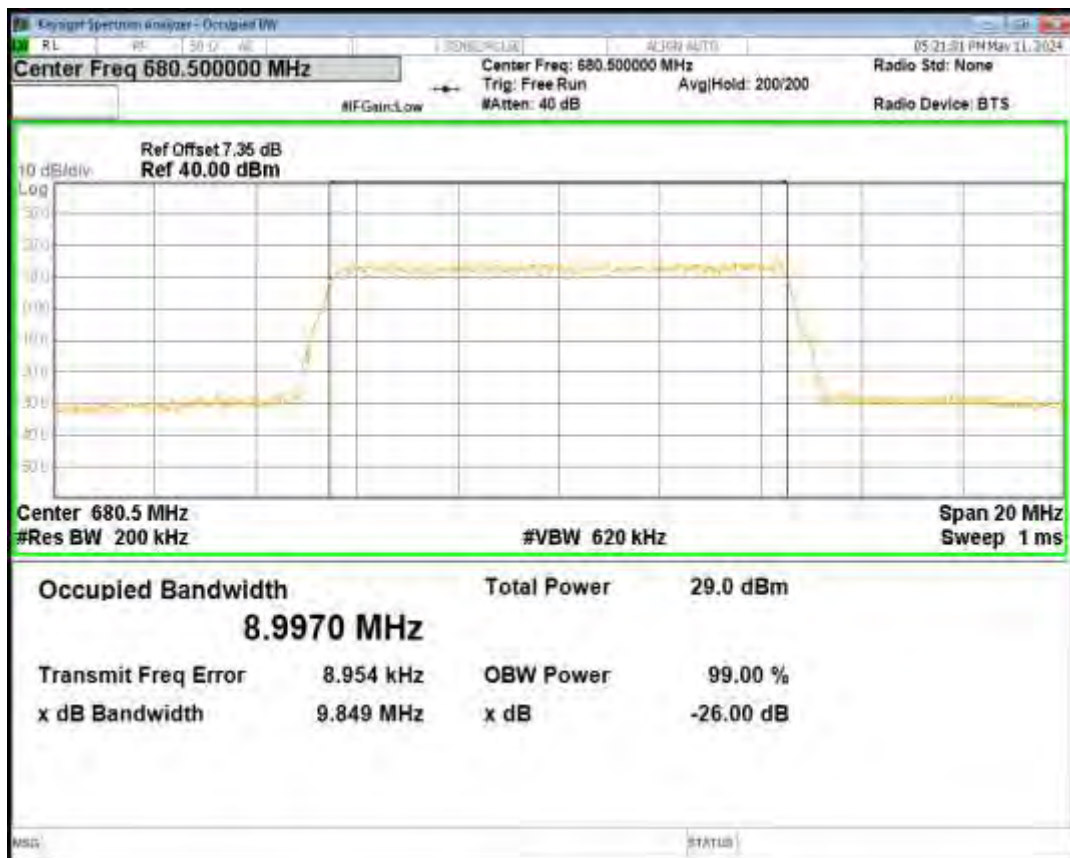
Band71 16QAM BW=10MHz Channel=133422 RB Size=50 Position=#0
