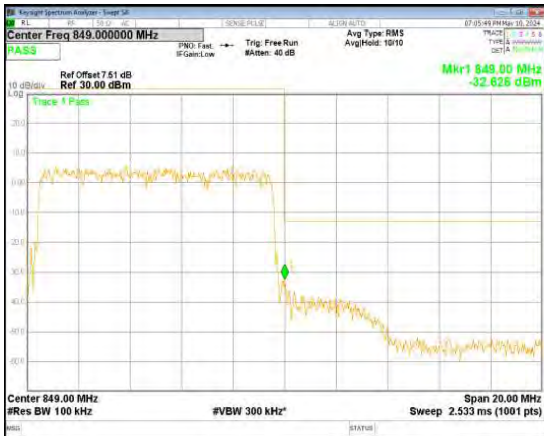
Band26(824-849) QPSK BW=10MHz Channel=26840 RB Size=50 Position=#0
