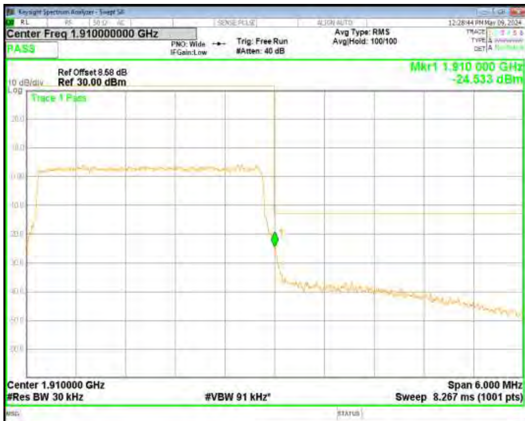
Band2 QPSK BW=10MHz Channel=18650 RB Size=50 Position=#0
