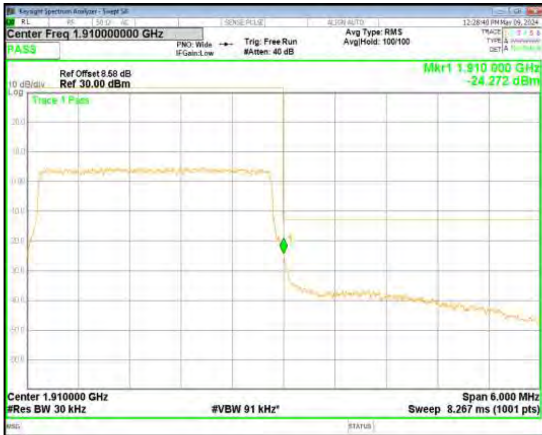
Band2 QPSK BW=5MHz Channel=19175 RB Size=25 Position=#0
