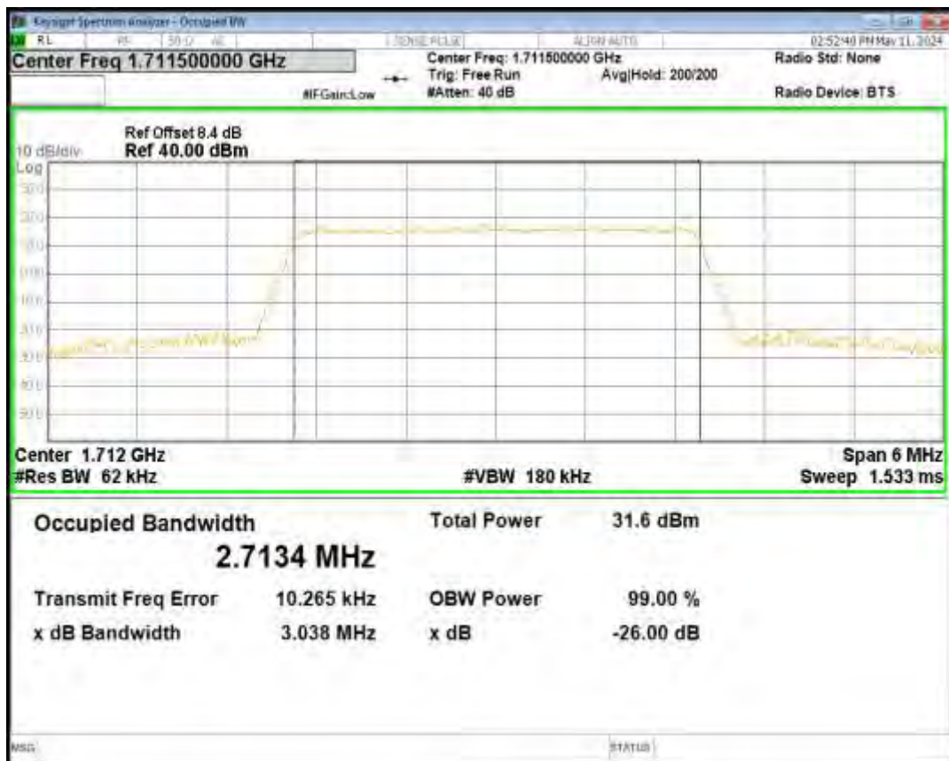
Band66 QPSK BW=3MHz Channel=132322 RB Size=15 Position=#0
