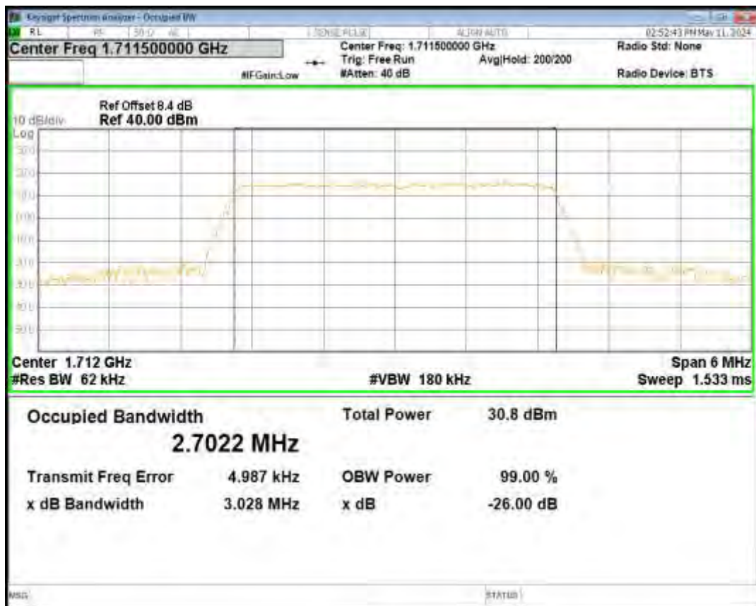
Band66 16QAM BW=20MHz Channel=132572 RB Size=100 Position=#0
