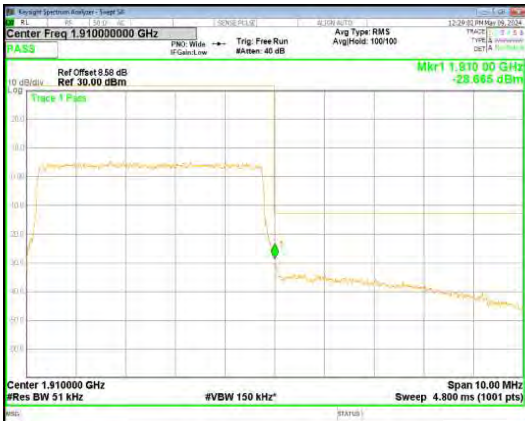
Band25 16QAM BW=1.4MHz Channel=26047 RB Size=6 Position=#0
