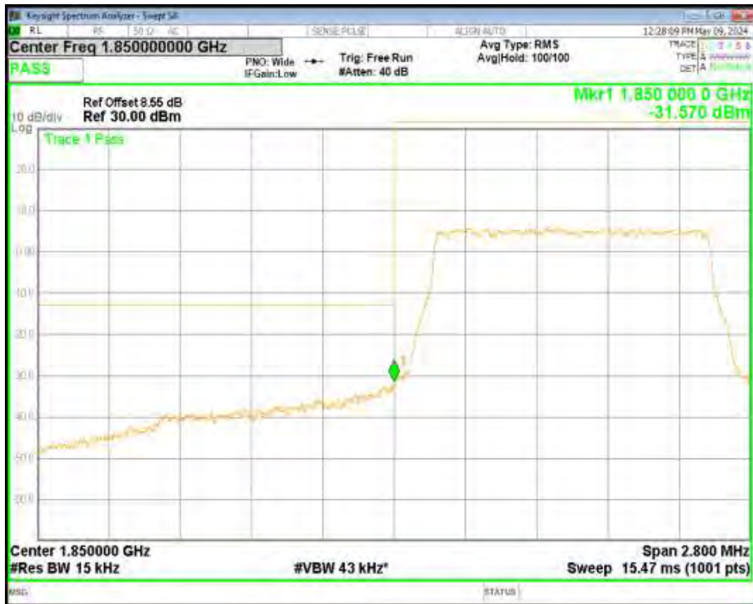
Band2 16QAM BW=5MHz Channel=18625 RB Size=25 Position=#0
