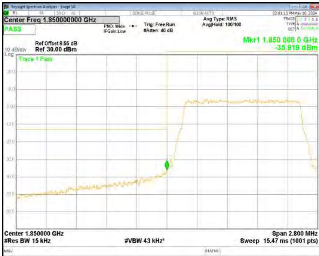
Band25 16QAM BW=1.4MHz Channel=26683 RB Size=6 Position=#0
