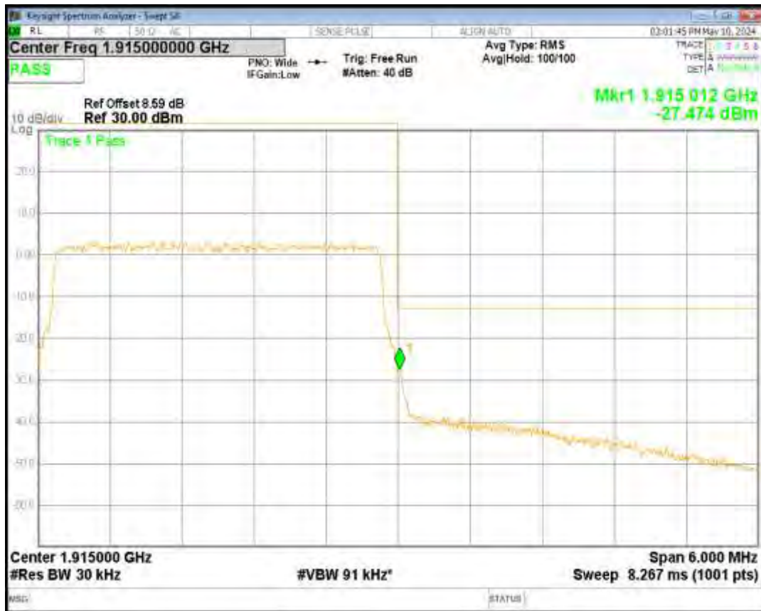
Band25 QPSK BW=10MHz Channel=26640 RB Size=50 Position=#0
