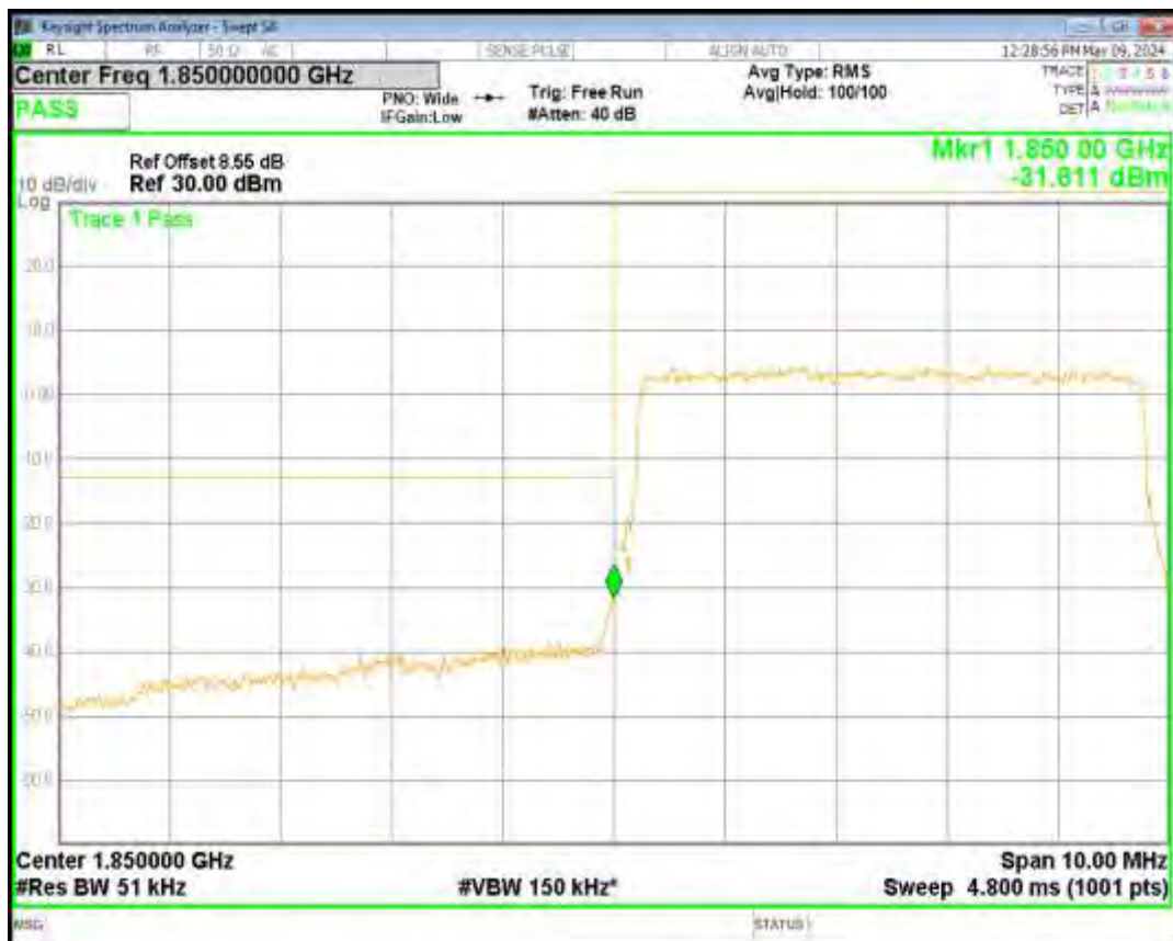
Band2 16QAM BW=5MHz Channel=19175 RB Size=25 Position=#0
