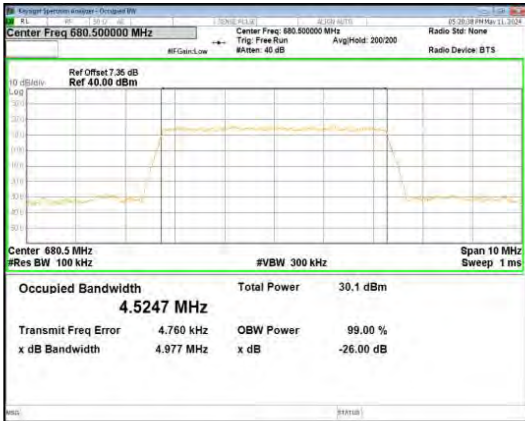
Band71 16QAM BW=5MHz Channel=133297 RB Size=25 Position=#0
