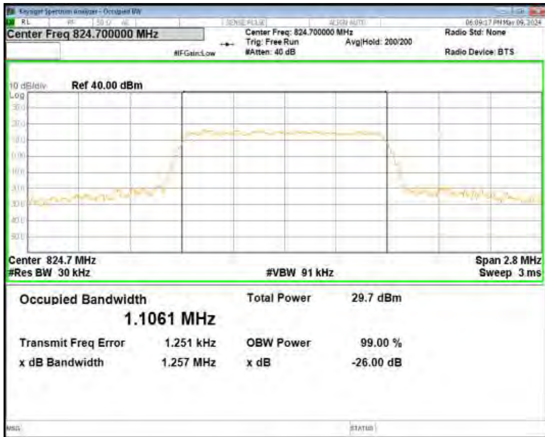
Band5 16QAM BW=1.4MHz Channel=20525 RB Size=6 Position=#0
