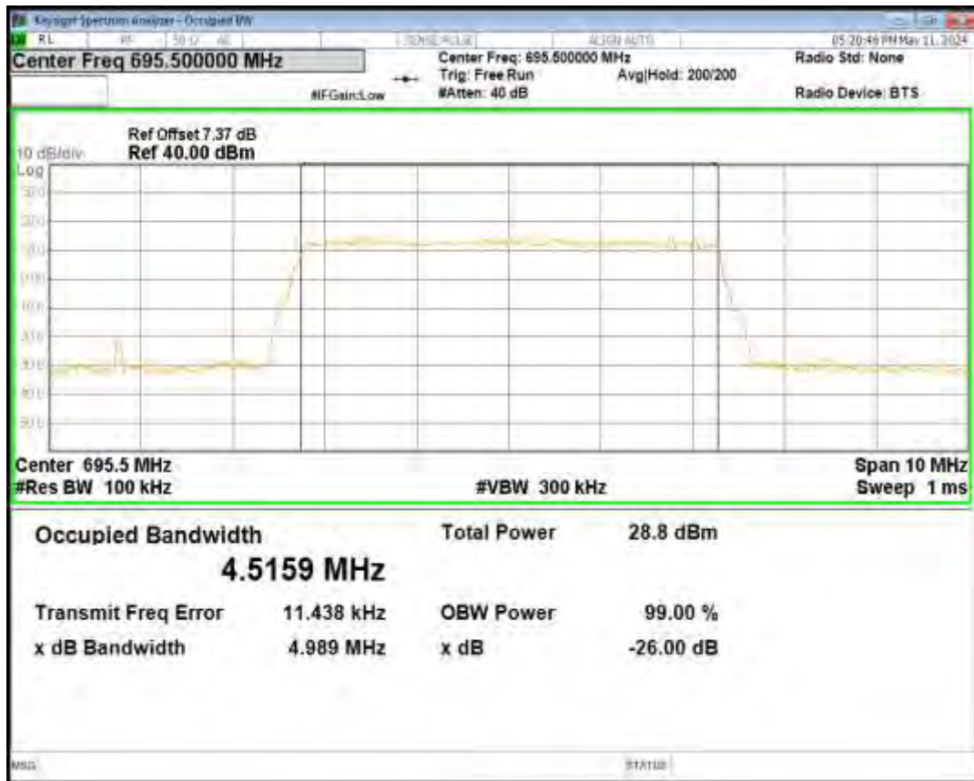
Band71 QPSK BW=10MHz Channel=133422 RB Size=50 Position=#0
