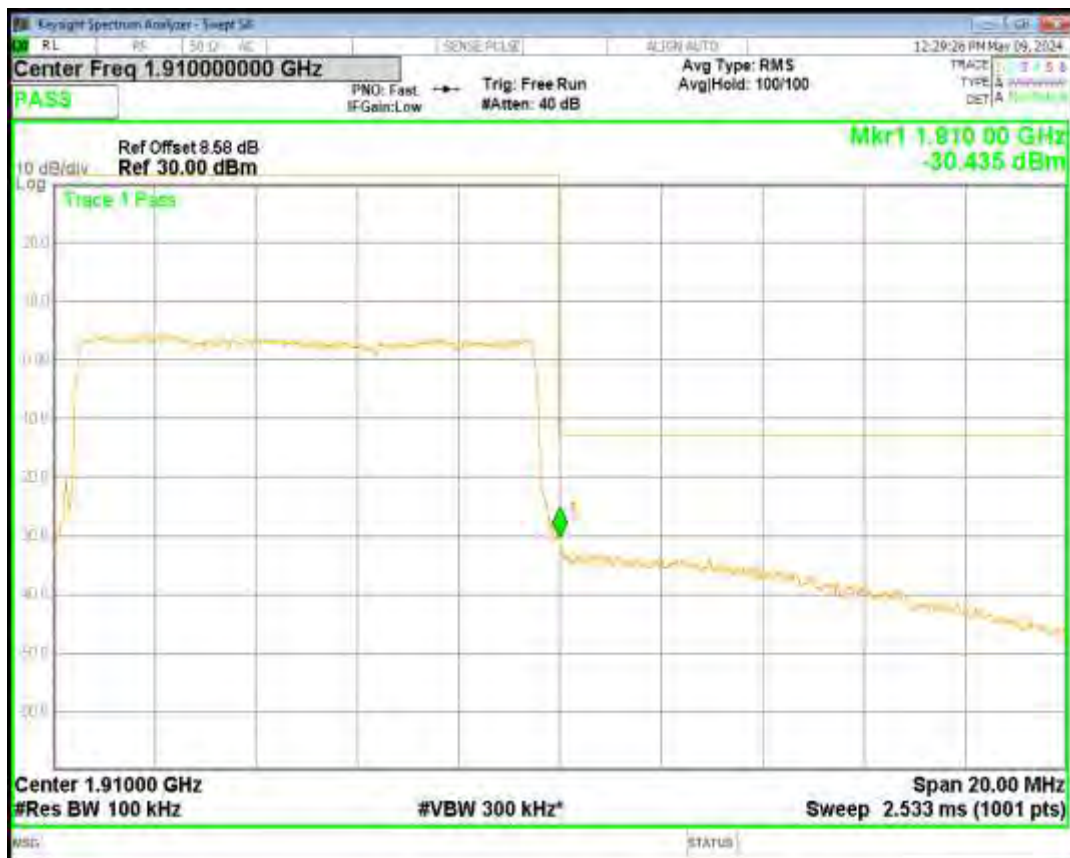
Band2 16QAM BW=15MHz Channel=18675 RB Size=75 Position=#0
