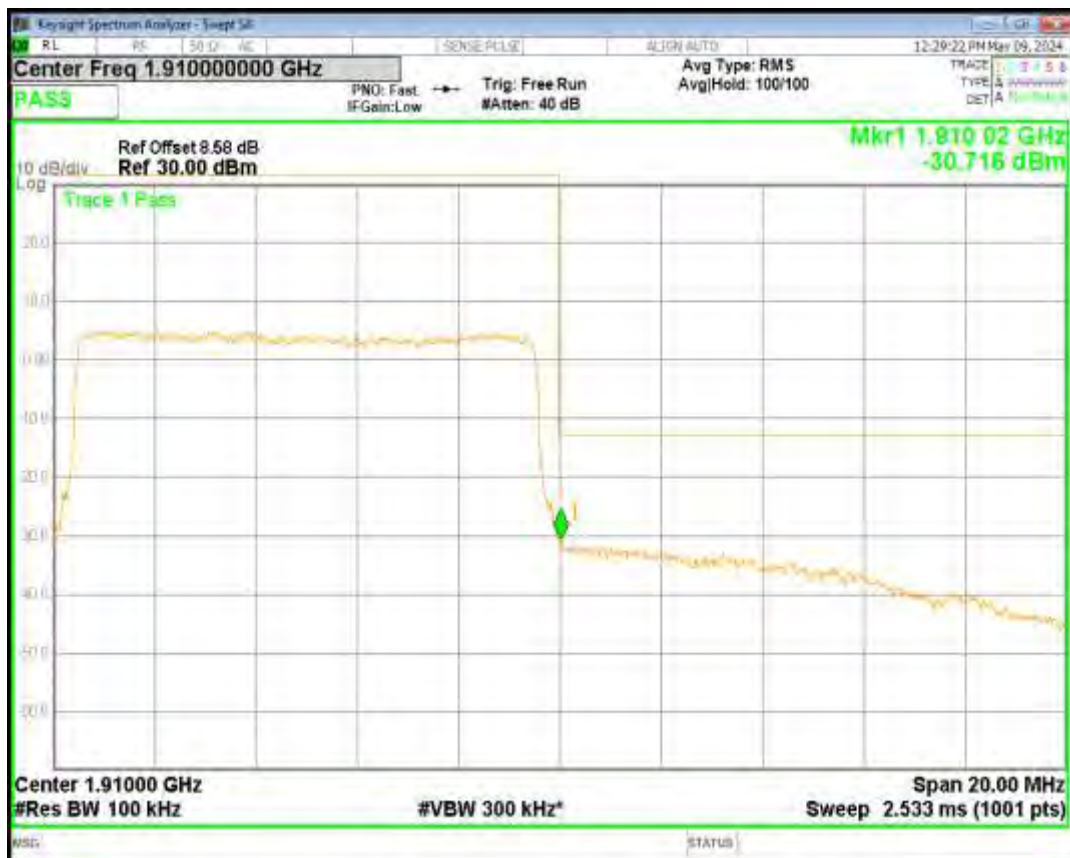
Band2 QPSK BW=5MHz Channel=18625 RB Size=25 Position=#0
