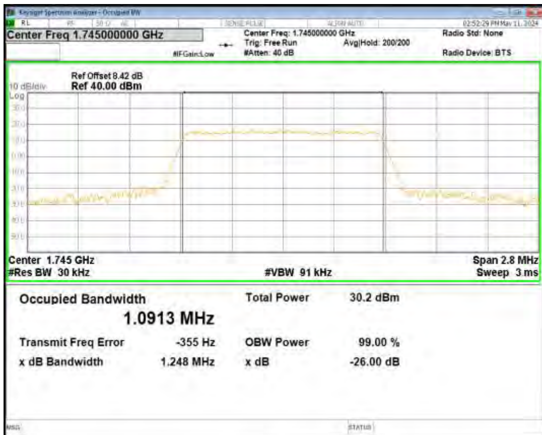
Band66 16QAM BW=1.4MHz Channel=132665 RB Size=6 Position=#0
