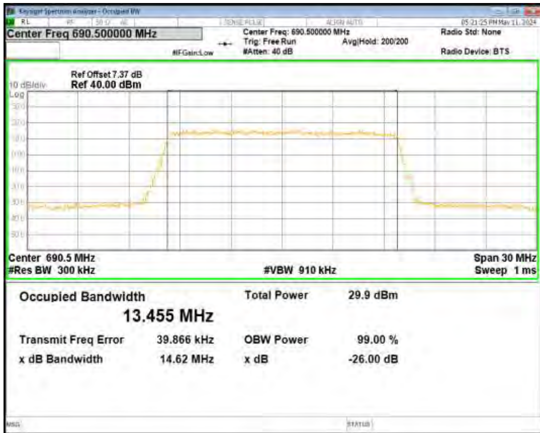
Band71 QPSK BW=15MHz Channel=133297 RB Size=75 Position=#0
