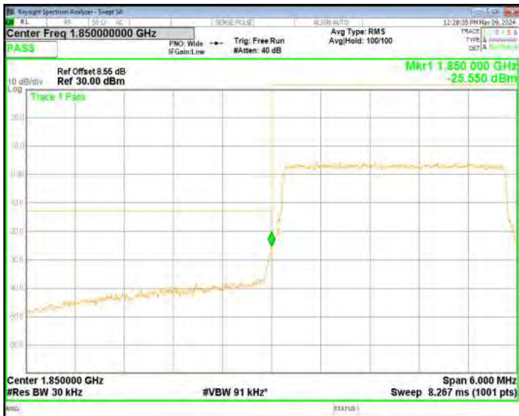
Band2 16QAM BW=20MHz Channel=19100 RB Size=100 Position=#0
