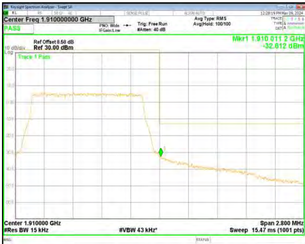
Band2 QPSK BW=1.4MHz Channel=18607 RB Size=6 Position=#0
