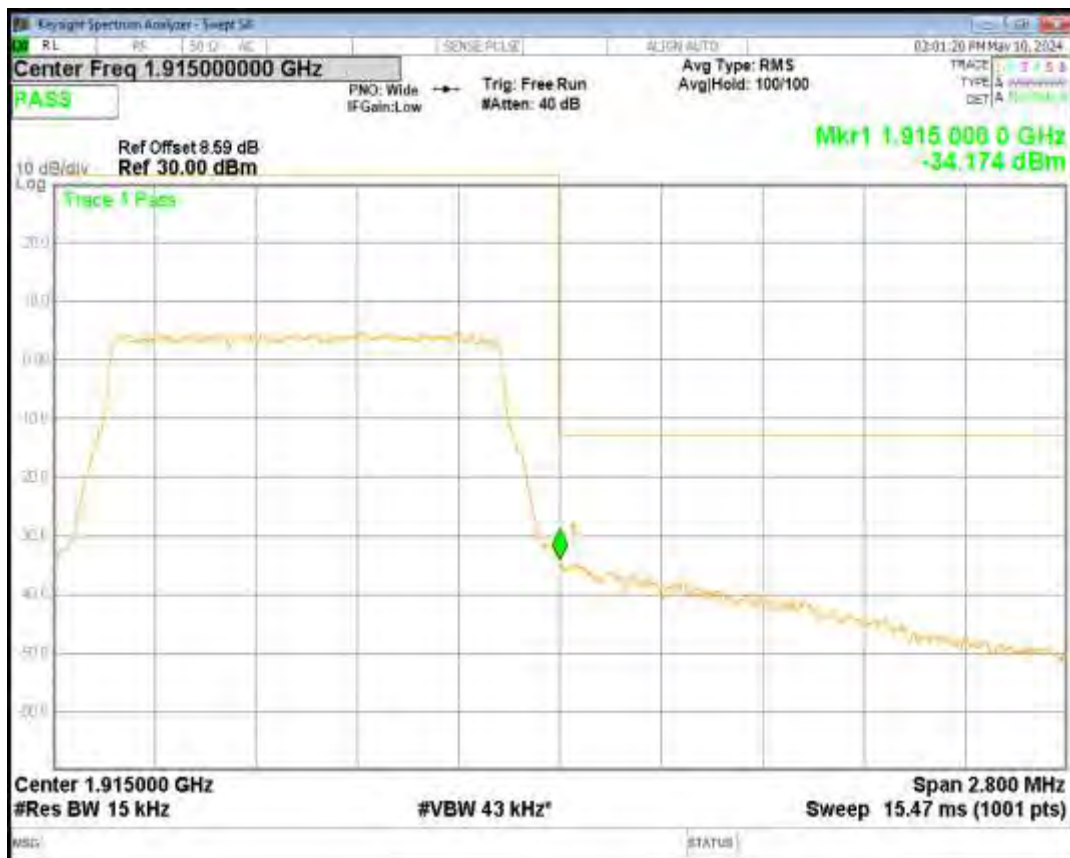
Band25 QPSK BW=1.4MHz Channel=26047 RB Size=6 Position=#0
