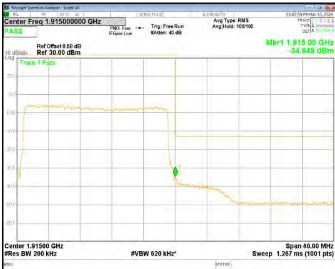
Band25 QPSK BW=20MHz Channel=26140 RB Size=100 Position=#0
