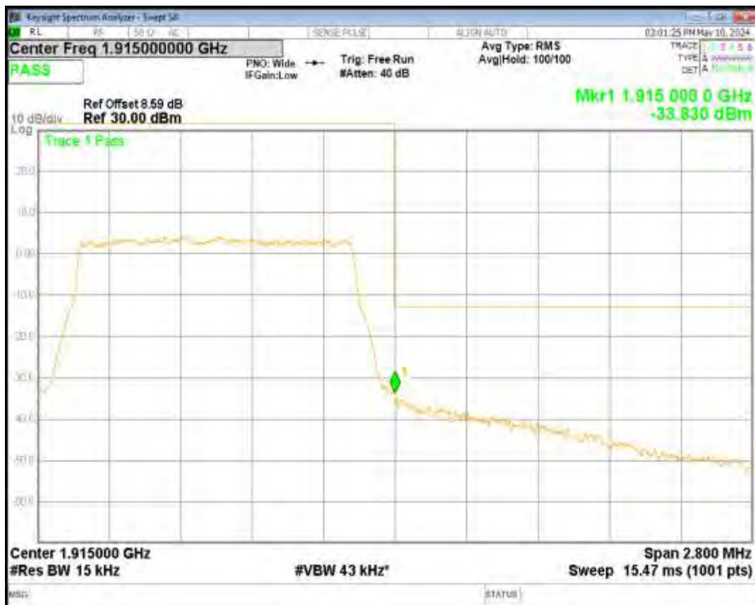
Band25 16QAM BW=10MHz Channel=26090 RB Size=50 Position=#0
