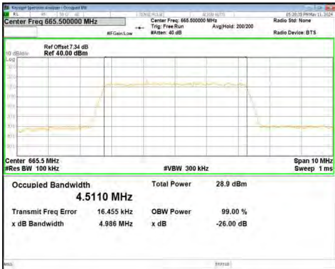
Band71 QPSK BW=5MHz Channel=133147 RB Size=25 Position=#0
