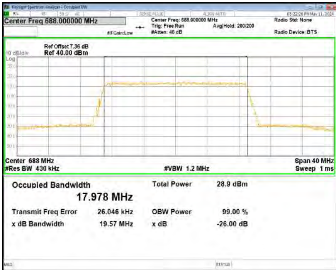
Band71 16QAM BW=5MHz Channel=133147 RB Size=25 Position=#0
