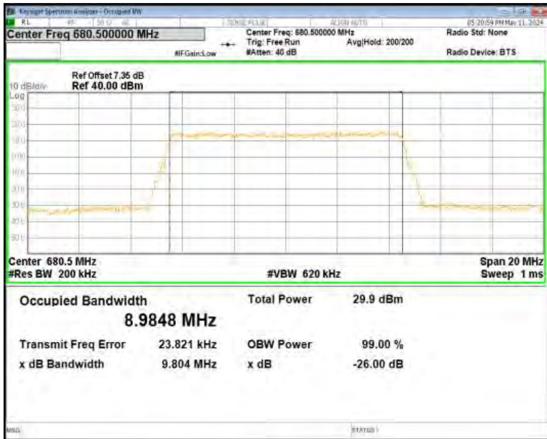
Band71 QPSK BW=10MHz Channel=133172 RB Size=50 Position=#0
