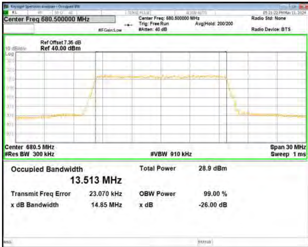
Band71 16QAM BW=15MHz Channel=133397 RB Size=75 Position=#0
