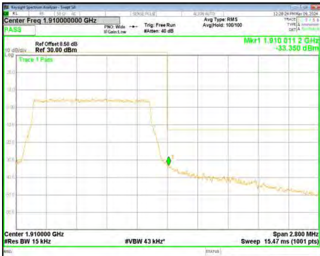
Band2 16QAM BW=10MHz Channel=18650 RB Size=50 Position=#0
