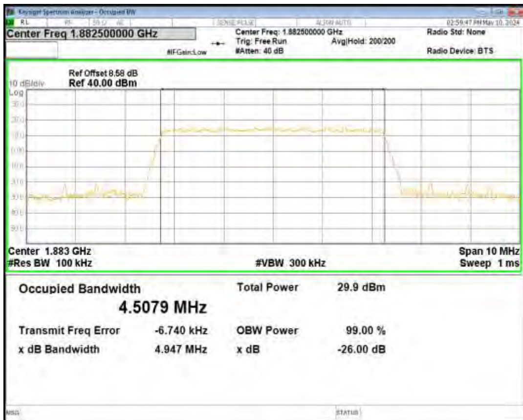
Band25 QPSK BW=15MHz Channel=26365 RB Size=75 Position=#0
