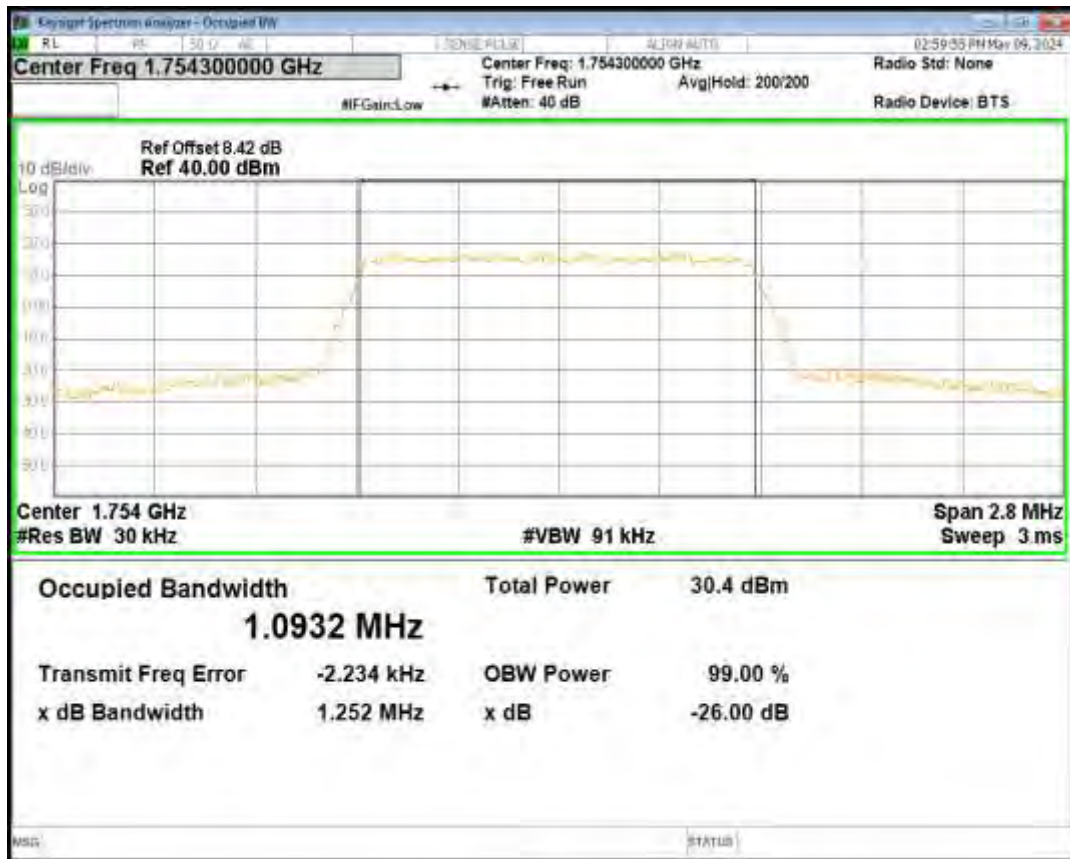
Band4 QPSK BW=10MHz Channel=20000 RB Size=50 Position=#0
