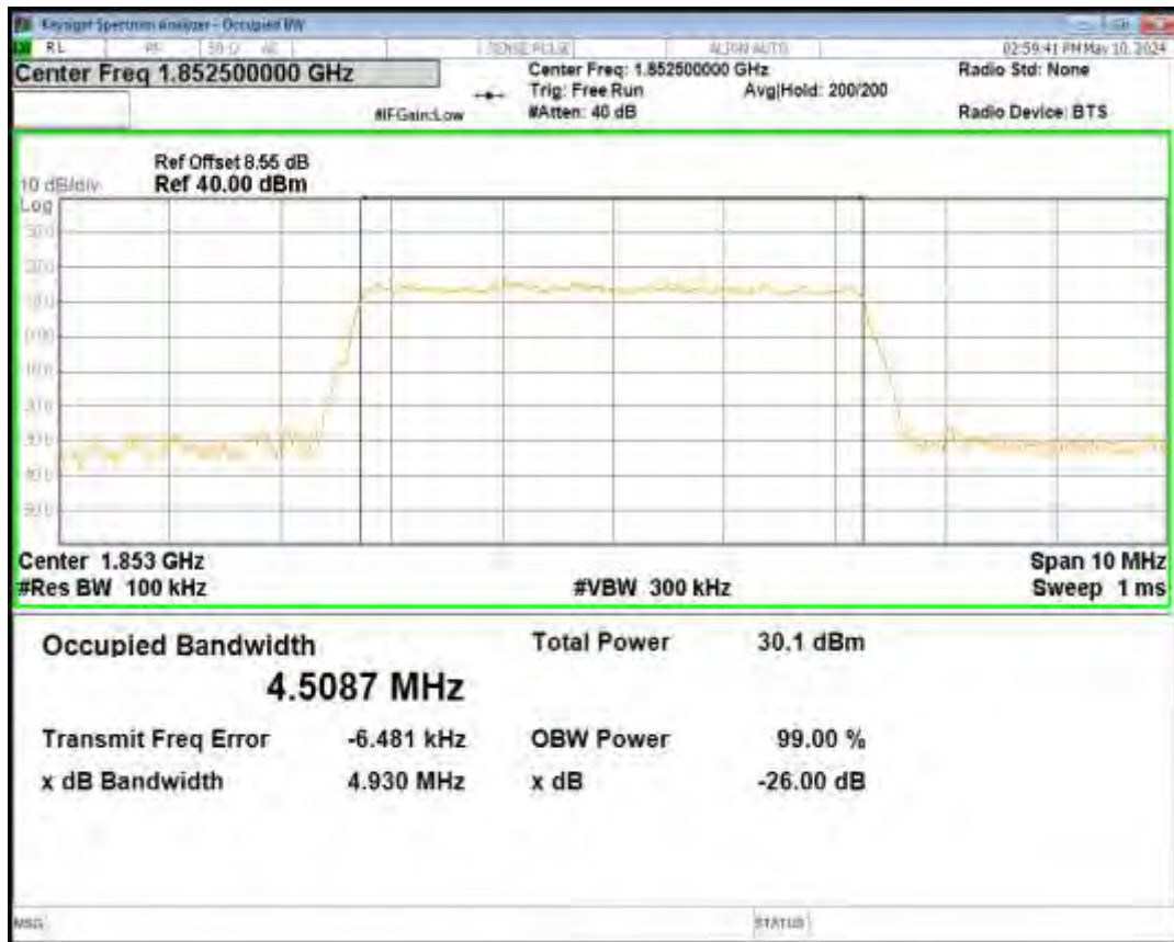
Band25 QPSK BW=5MHz Channel=26665 RB Size=25 Position=#0
