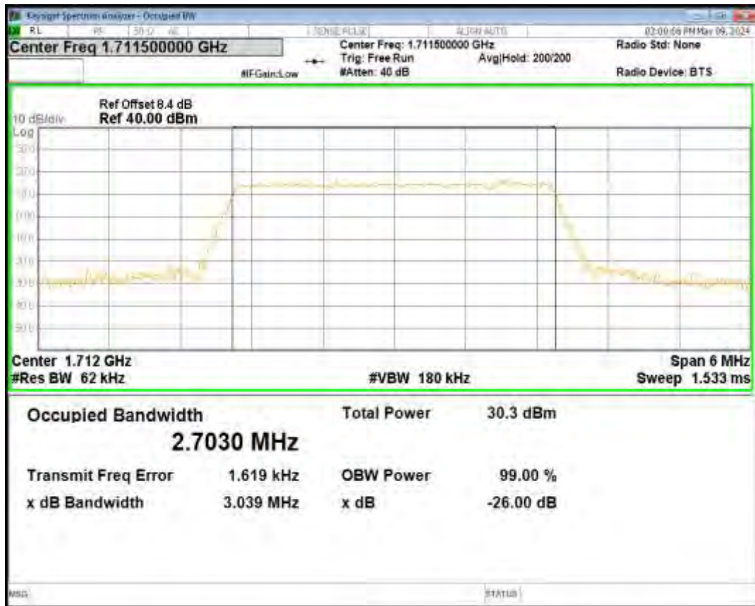
Band4 16QAM BW=3MHz Channel=20175 RB Size=15 Position=#0
