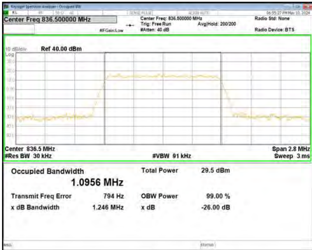
Band26(824-849) QPSK BW=1.4MHz Channel=26797 RB Size=6 Position=#0
