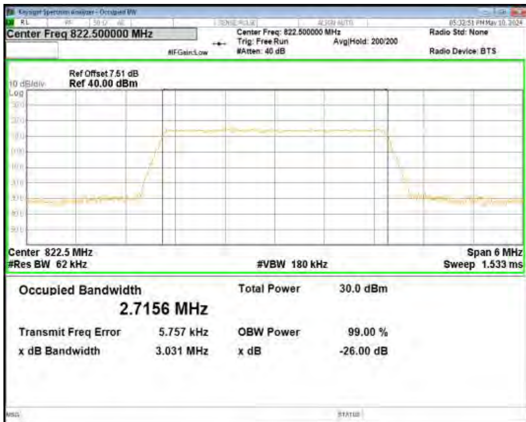
Band26(814-824) QPSK BW=5MHz Channel=26715 RB Size=25 Position=#0
