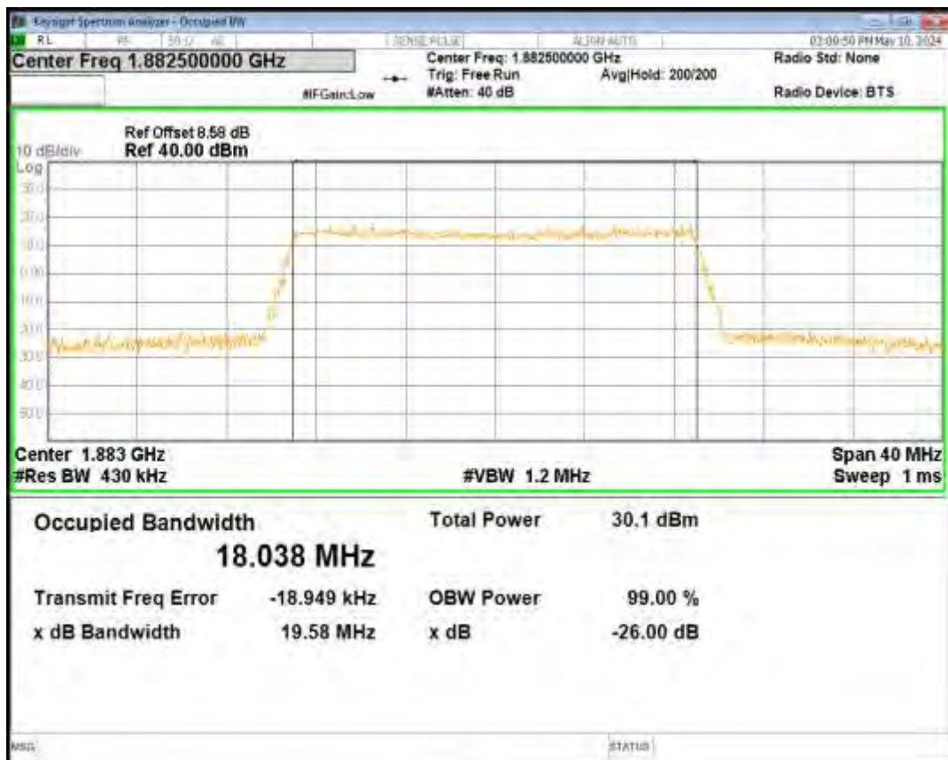
Band25 QPSK BW=20MHz Channel=26590 RB Size=100 Position=#0
