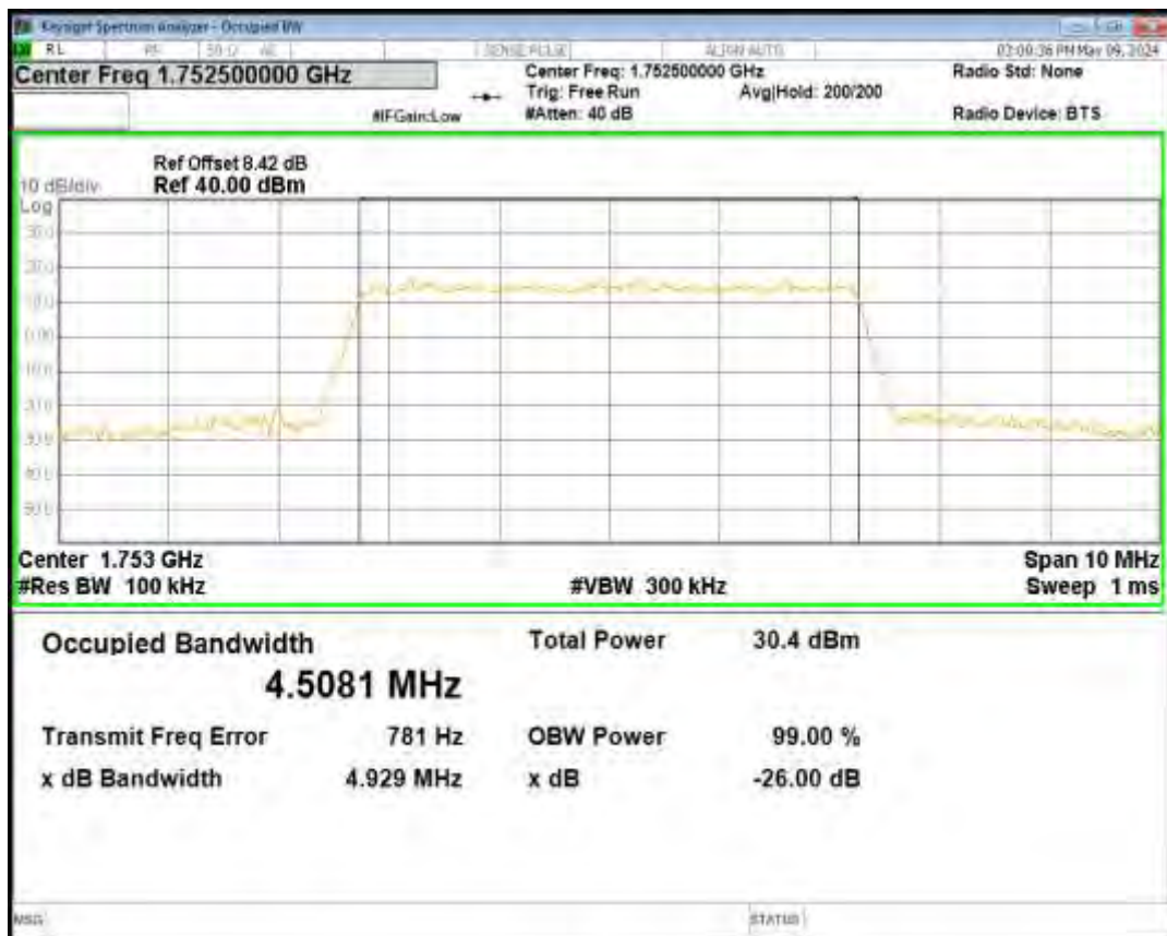
Band41 16QAM BW=10MHz Channel=39700 RB Size=50 Position=#0
