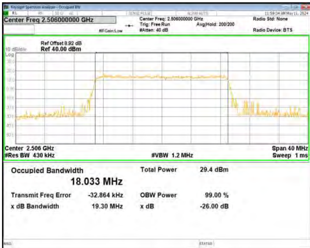
Band41 QPSK BW=15MHz Channel=41515 RB Size=75 Position=#0
