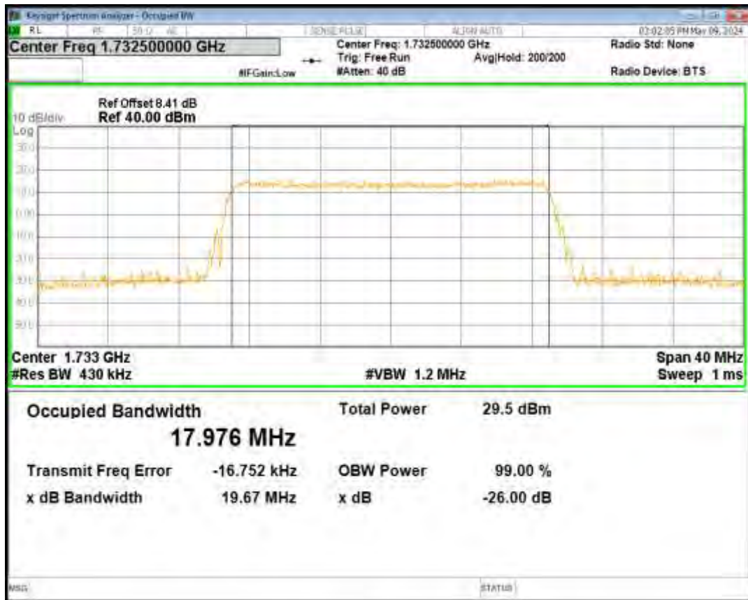
Band4 16QAM BW=20MHz Channel=20300 RB Size=100 Position=#0
