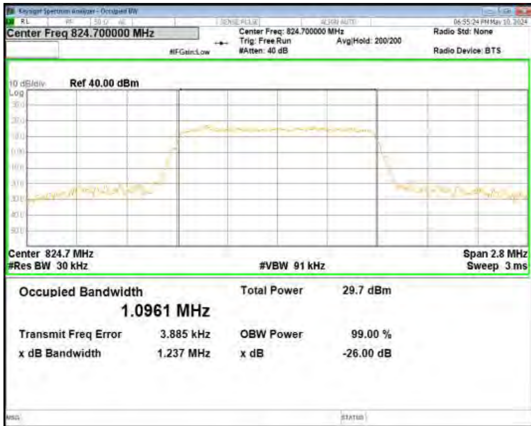
Band26(824-849) 16QAM BW=3MHz Channel=26915 RB Size=15 Position=#0
