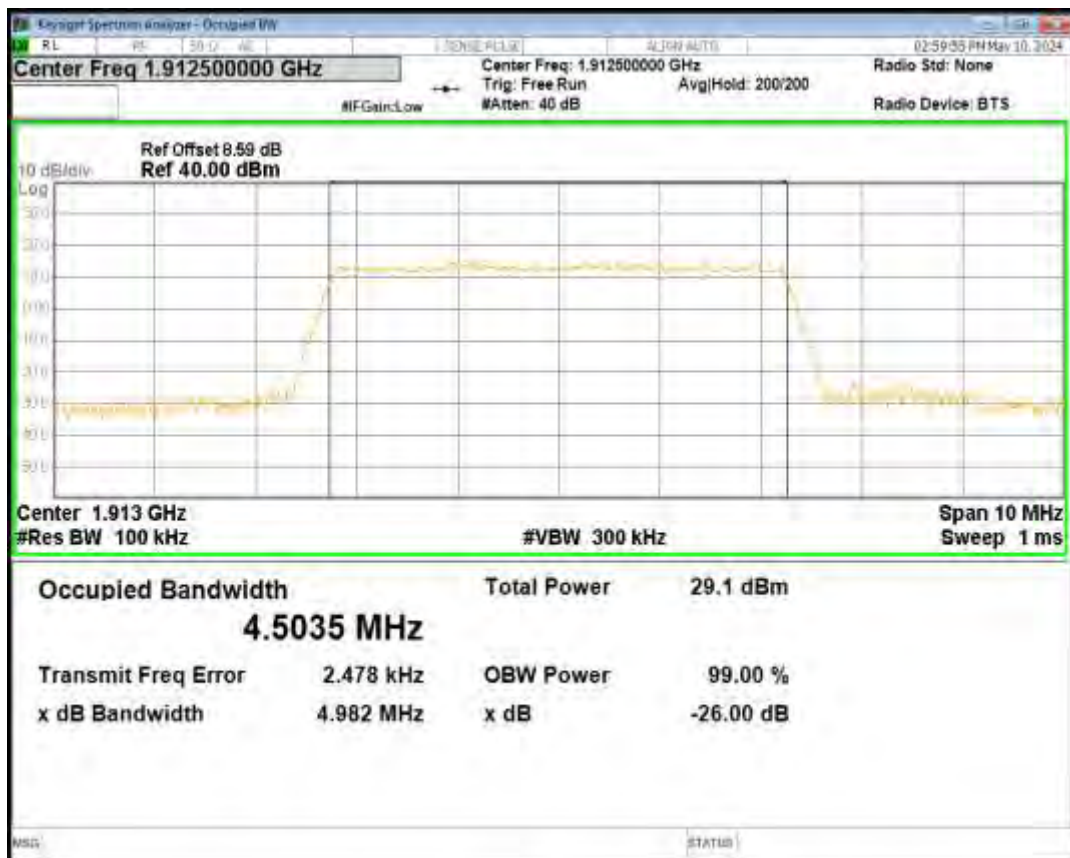
Band25 16QAM BW=5MHz Channel=26365 RB Size=25 Position=#0
