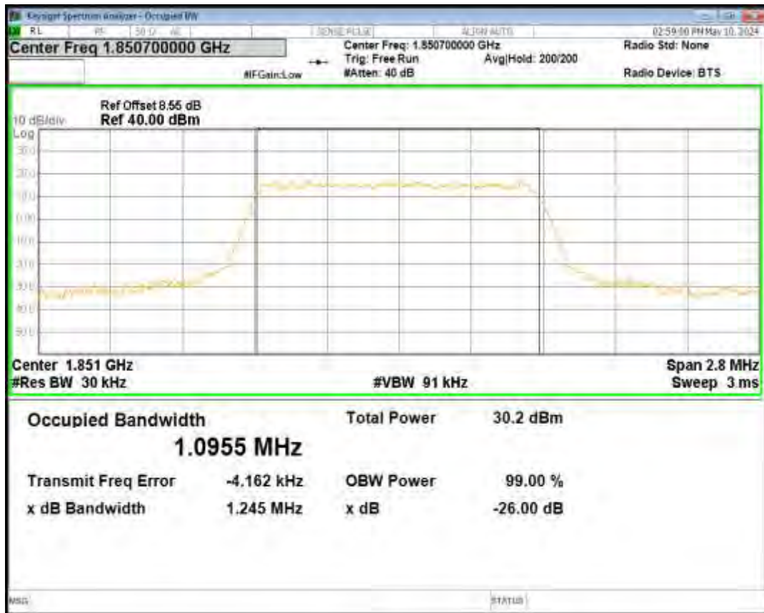
Band25 QPSK BW=5MHz Channel=26365 RB Size=25 Position=#0
