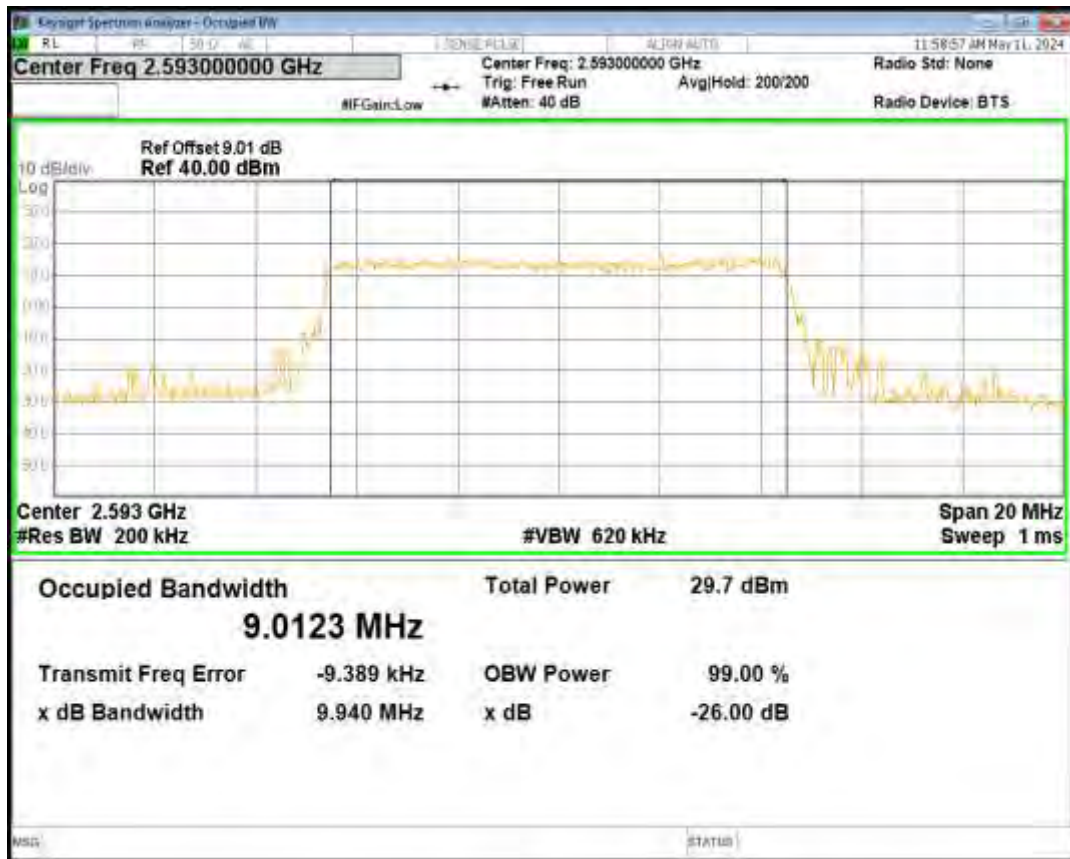
Band41 QPSK BW=10MHz Channel=39700 RB Size=50 Position=#0
