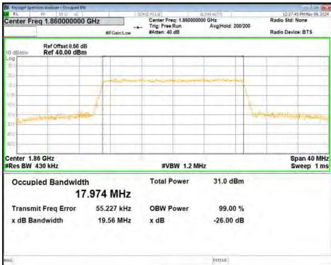
Band2 QPSK BW=20MHz Channel=18900 RB Size=100 Position=#0
