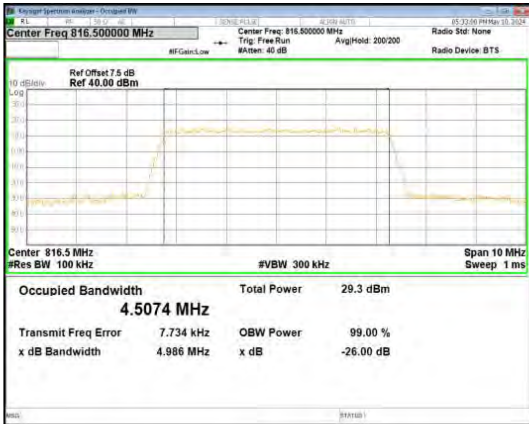
Band26(814-824) QPSK BW=5MHz Channel=26765 RB Size=25 Position=#0
