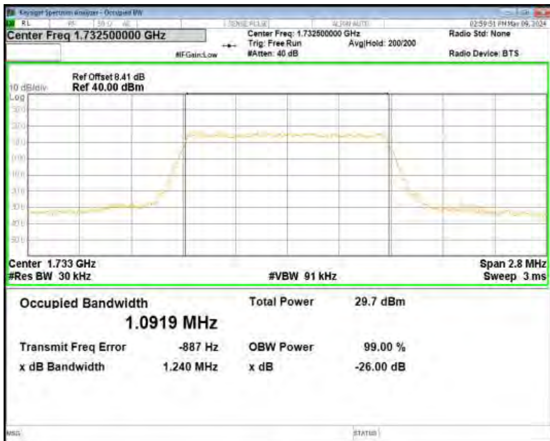
Band4 16QAM BW=1.4MHz Channel=20393 RB Size=6 Position=#0
