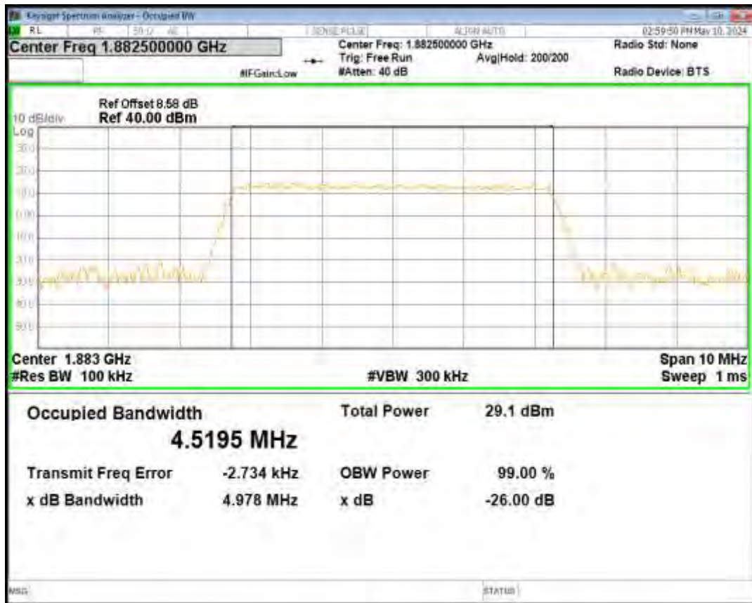
Band25 16QAM BW=5MHz Channel=26065 RB Size=25 Position=#0
