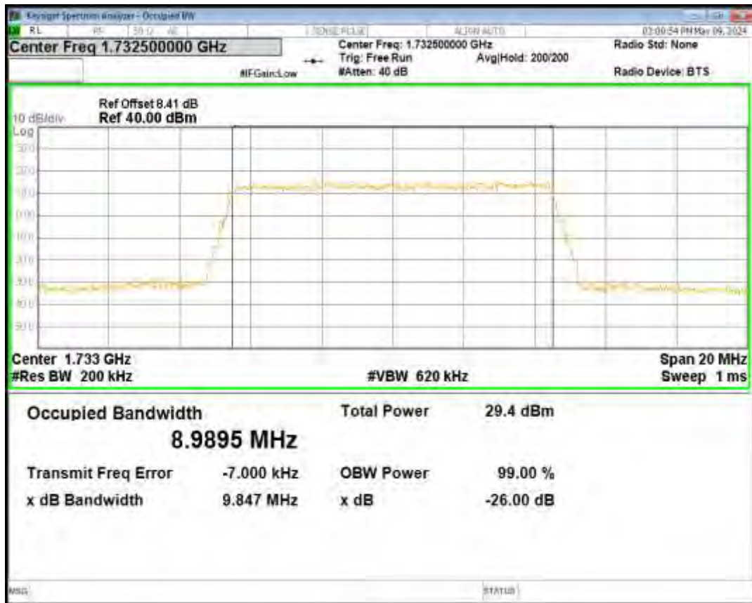
Band4 16QAM BW=10MHz Channel=20350 RB Size=50 Position=#0
