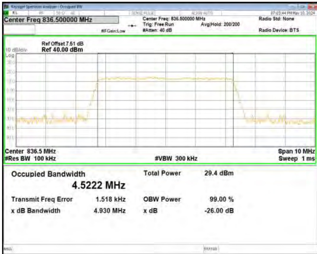
Band26(824-849) QPSK BW=3MHz Channel=26805 RB Size=15 Position=#0
