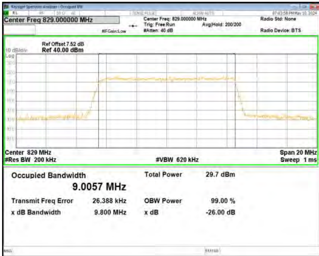
Band26(824-849) 16QAM BW=5MHz Channel=27015 RB Size=25 Position=#0
