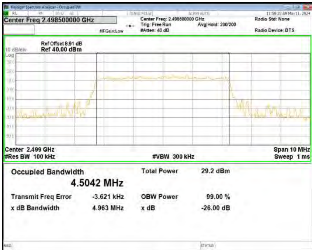
Band41 QPSK BW=5MHz Channel=39675 RB Size=25 Position=#0
