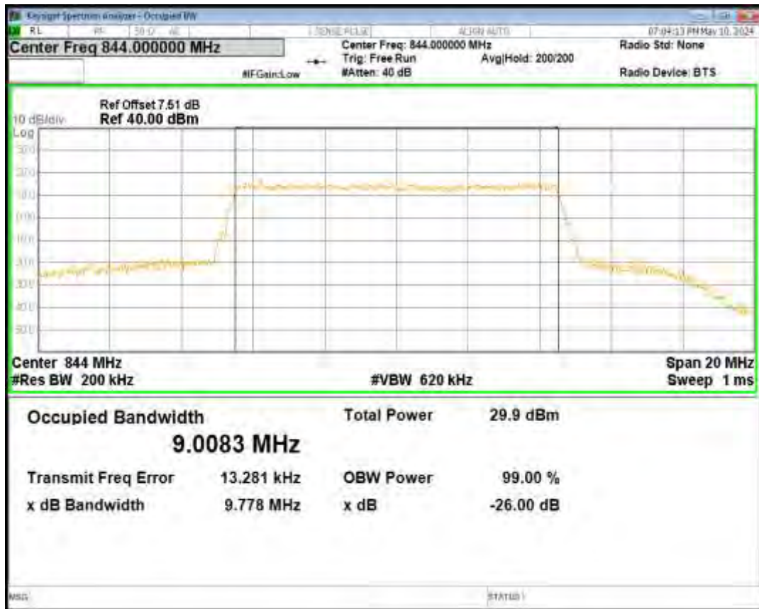
Band26(824-849) QPSK BW=10MHz Channel=26915 RB Size=50 Position=#0
