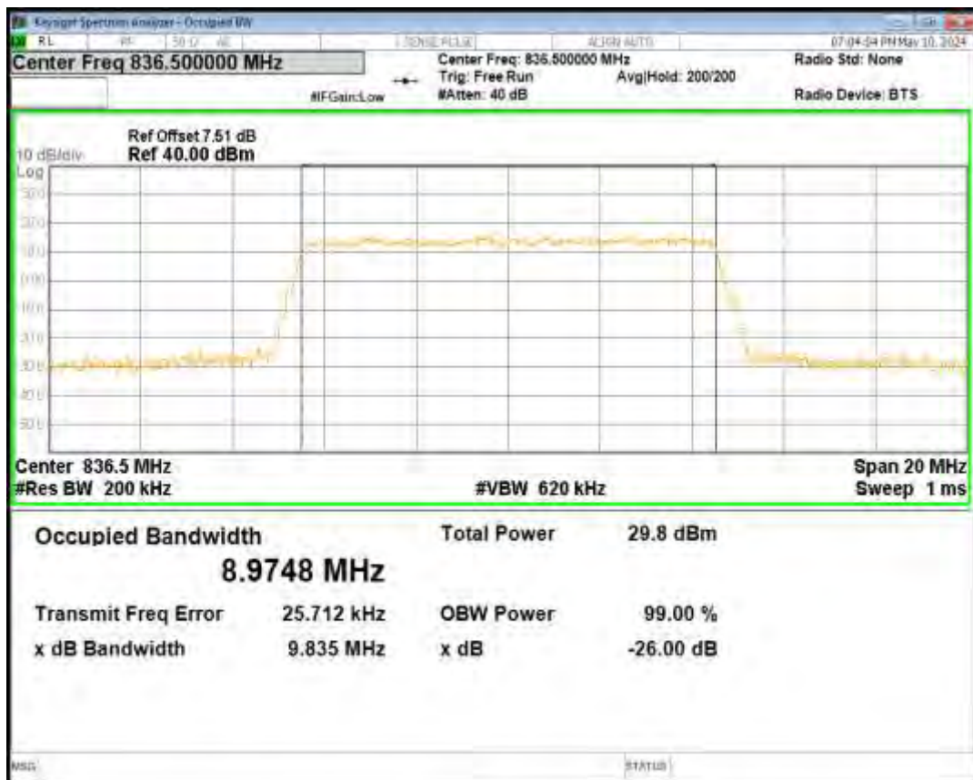
Band26(824-849) QPSK BW=15MHz Channel=26965 RB Size=75 Position=#0
