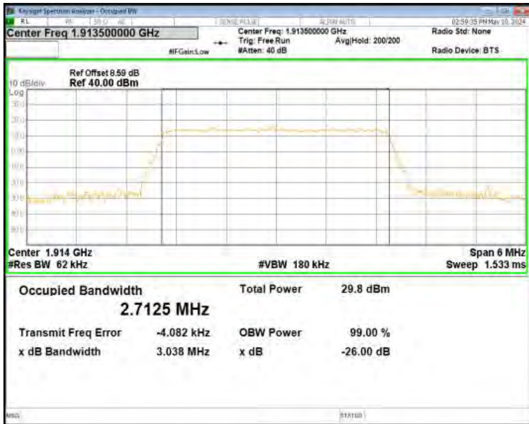
Band25 16QAM BW=3MHz Channel=26365 RB Size=15 Position=#0
