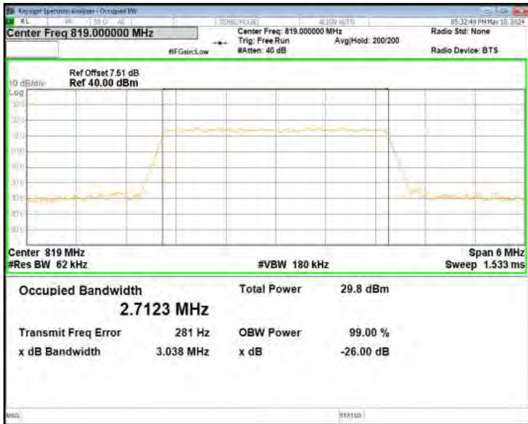
Band26(814-824) QPSK BW=3MHz Channel=26775 RB Size=15 Position=#0
