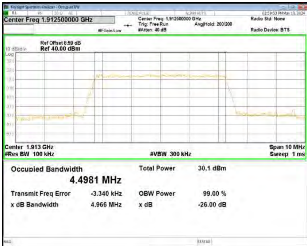
Band26(814-824) 16QAM BW=1.4MHz Channel=26697 RB Size=6 Position=#0
