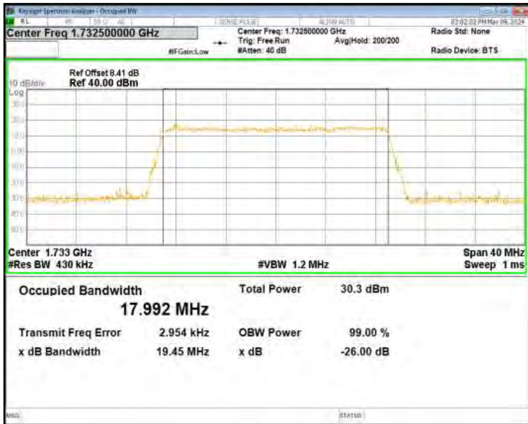
Band4 QPSK BW=5MHz Channel=20375 RB Size=25 Position=#0
