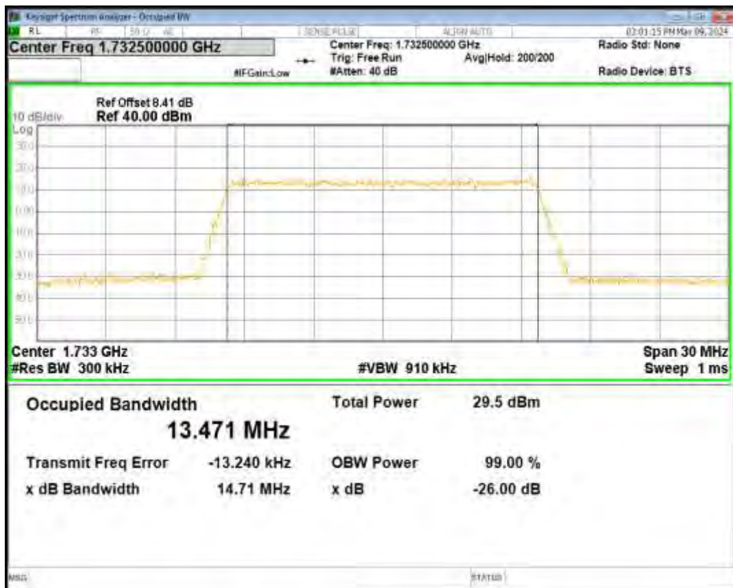
Band4 16QAM BW=15MHz Channel=20325 RB Size=75 Position=#0
