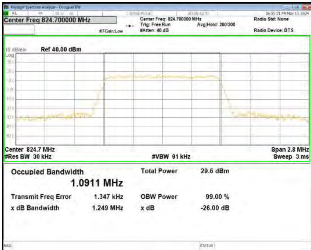
Band26(824-849) 16QAM BW=5MHz Channel=26915 RB Size=25 Position=#0
