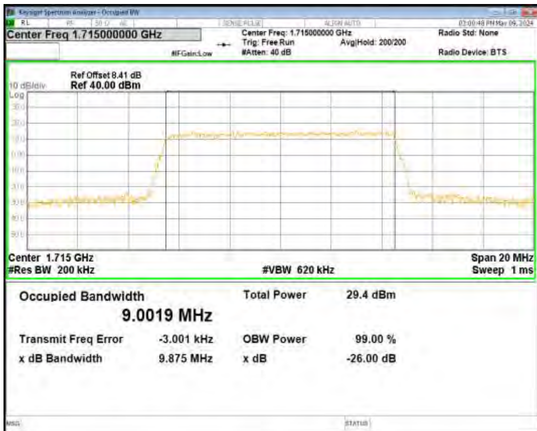
Band4 16QAM BW=10MHz Channel=20175 RB Size=50 Position=#0
