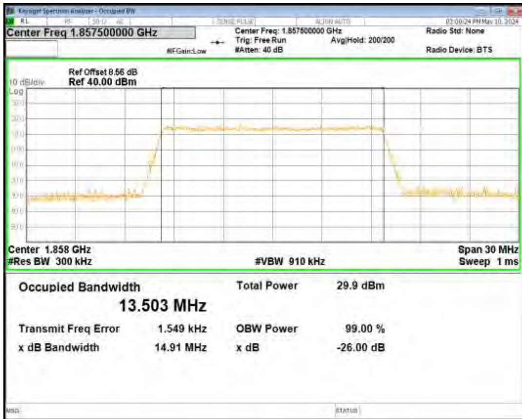
Band25 QPSK BW=10MHz Channel=26640 RB Size=50 Position=#0
