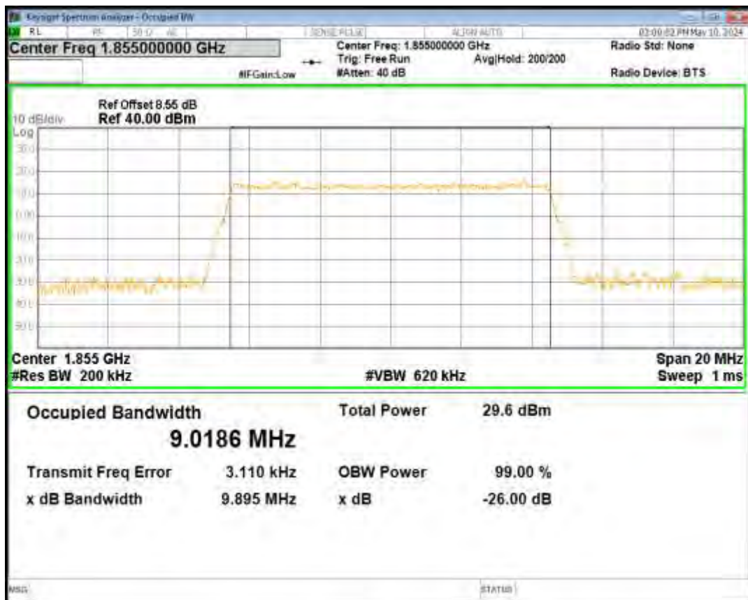
Band25 QPSK BW=1.4MHz Channel=26365 RB Size=6 Position=#0
