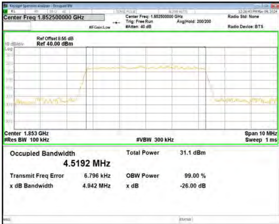
Band2 QPSK BW=5MHz Channel=19175 RB Size=25 Position=#0
