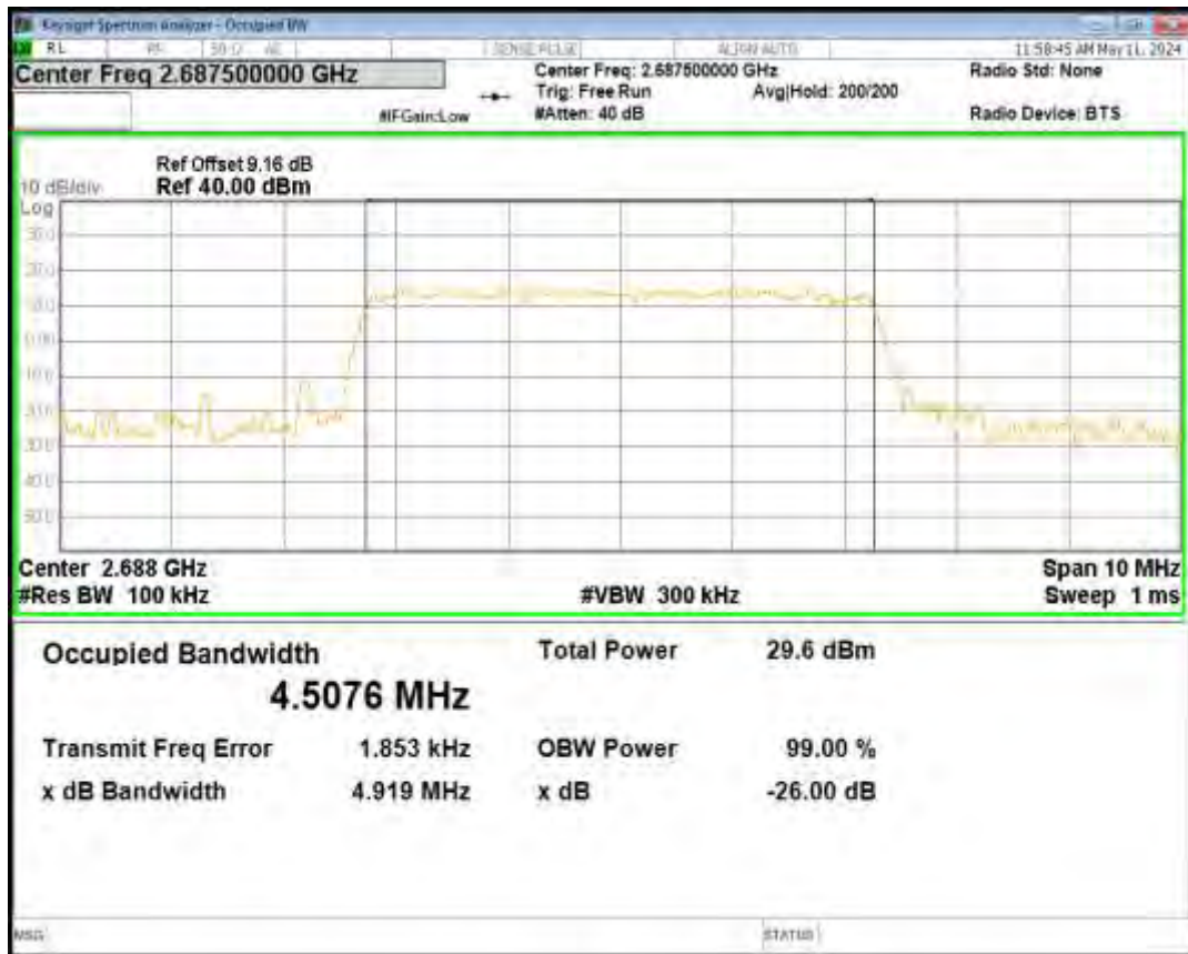
Band41 QPSK BW=10MHz Channel=41540 RB Size=50 Position=#0
