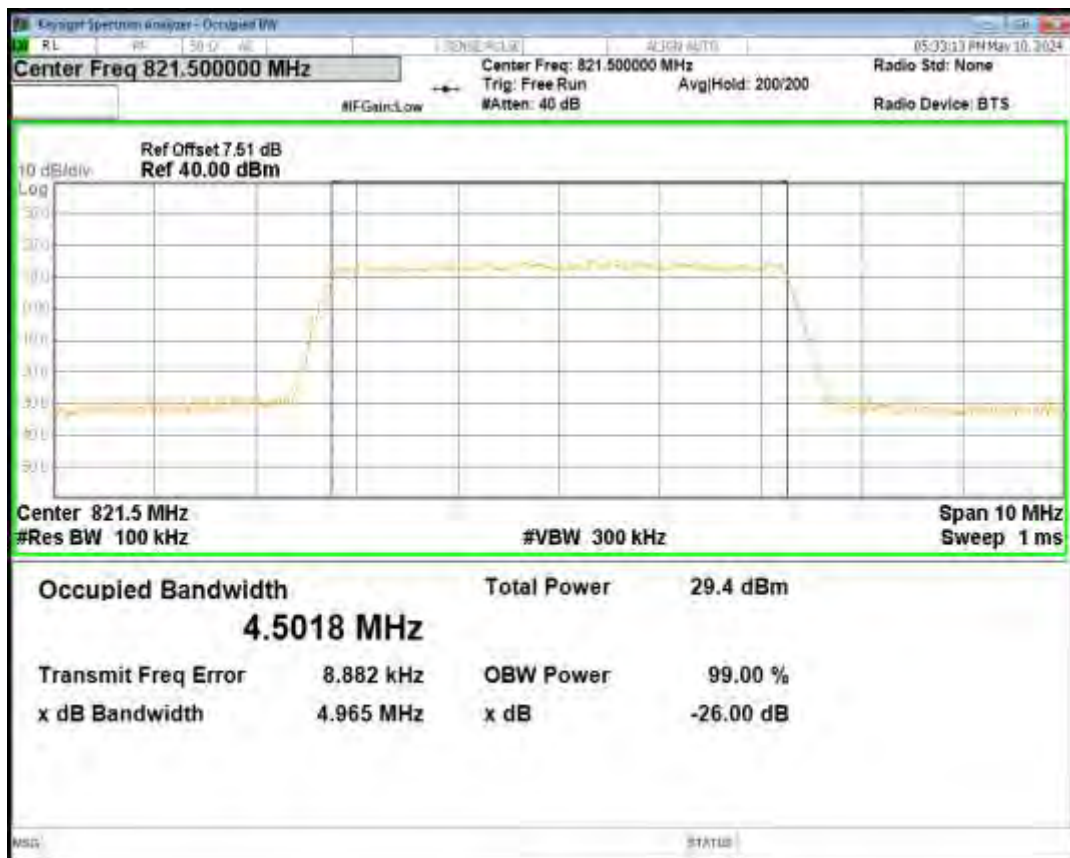
Band26(824-849) 16QAM BW=1.4MHz Channel=26797 RB Size=6 Position=#0
