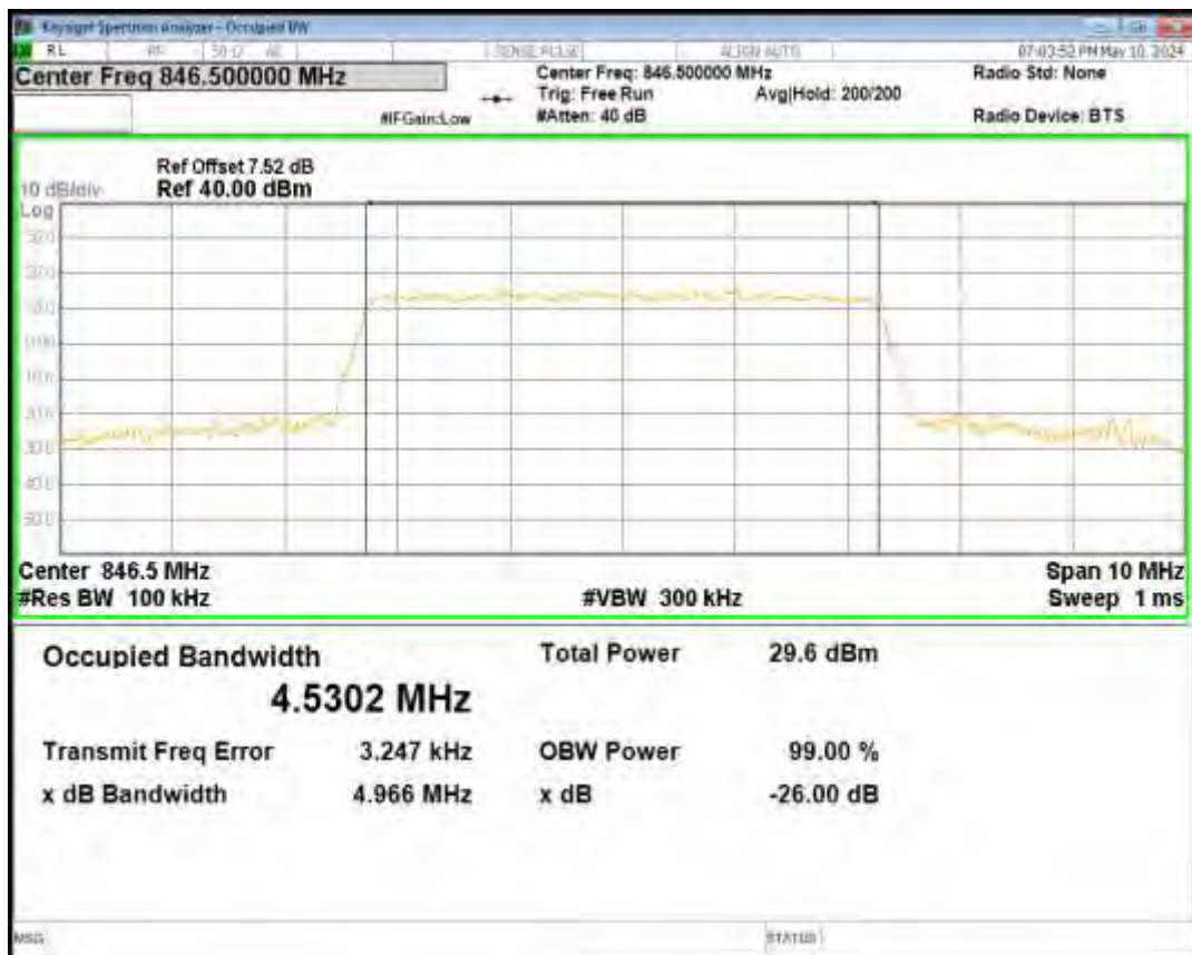
Band26(824-849) QPSK BW=1.4MHz Channel=26915 RB Size=6 Position=#0
