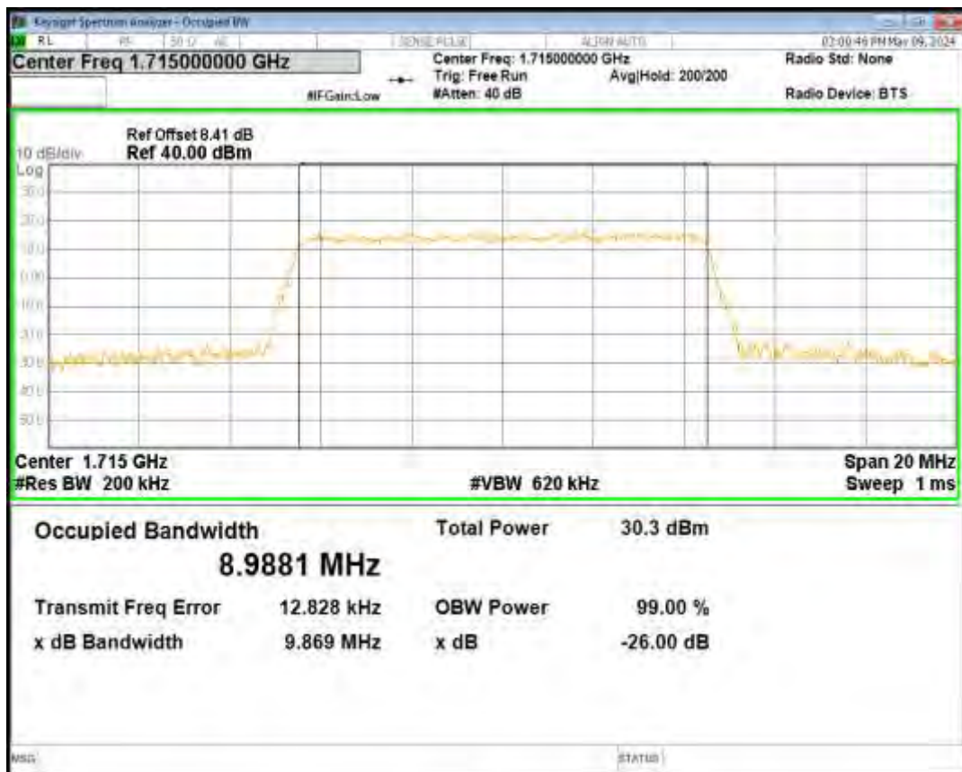
Band4 QPSK BW=10MHz Channel=20175 RB Size=50 Position=#0
