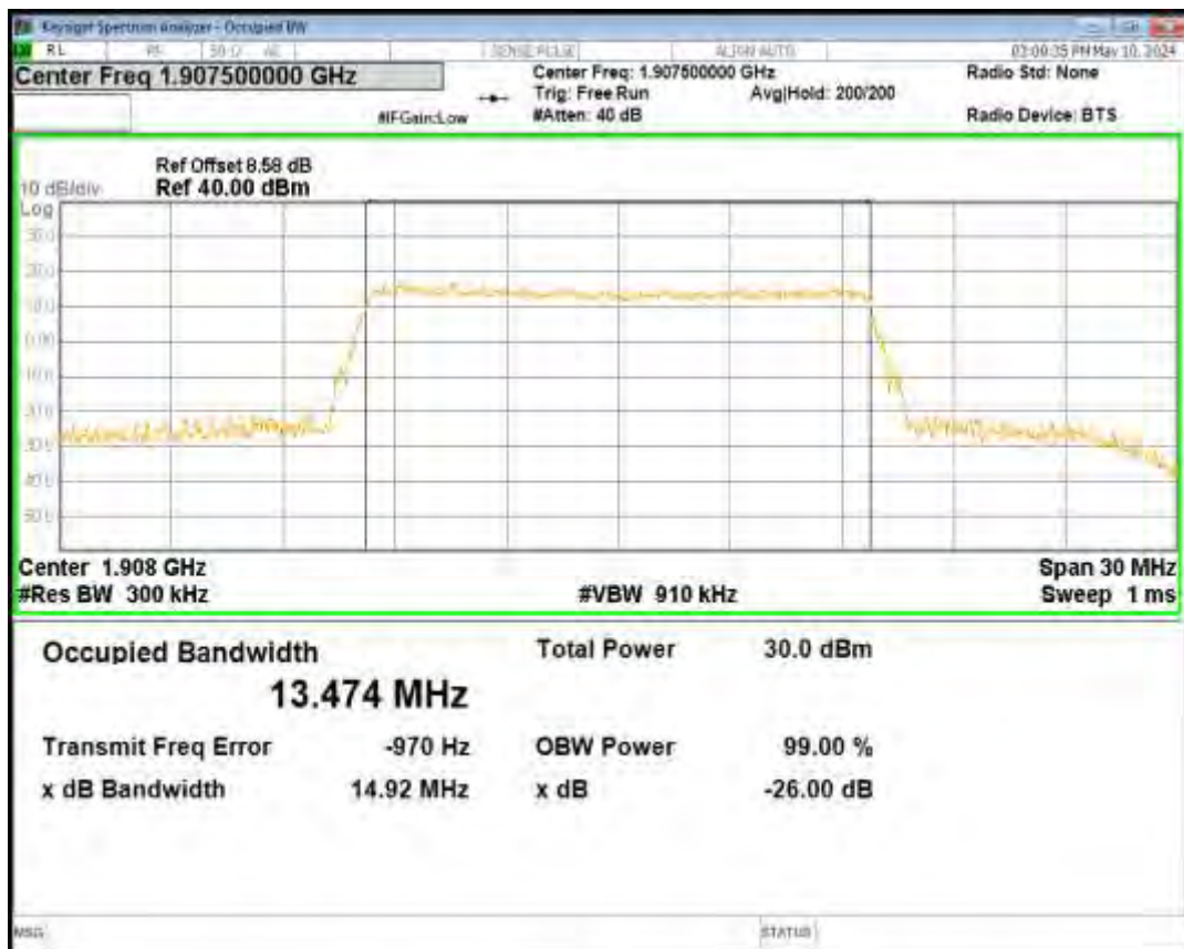
Band25 QPSK BW=20MHz Channel=26140 RB Size=100 Position=#0
