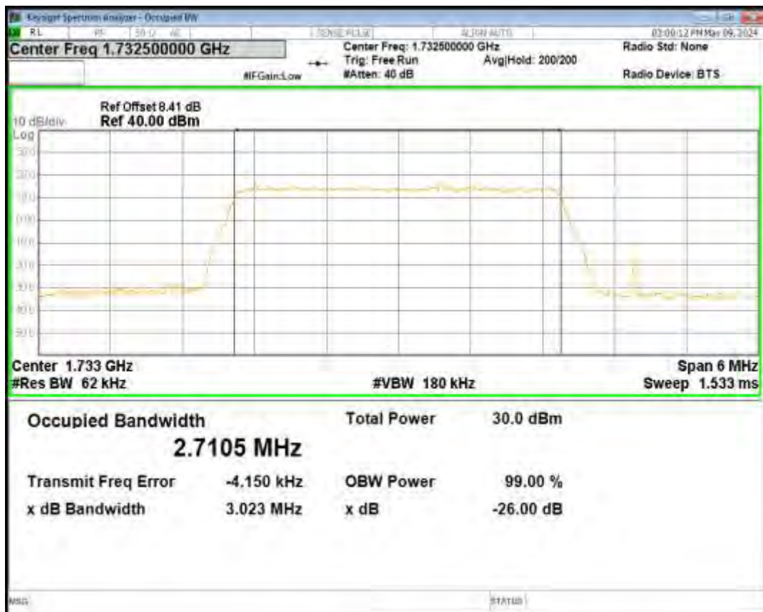
Band4 16QAM BW=3MHz Channel=20385 RB Size=15 Position=#0
