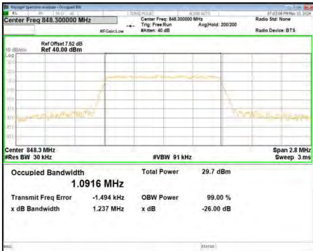
Band26(824-849) QPSK BW=5MHz Channel=26915 RB Size=25 Position=#0
