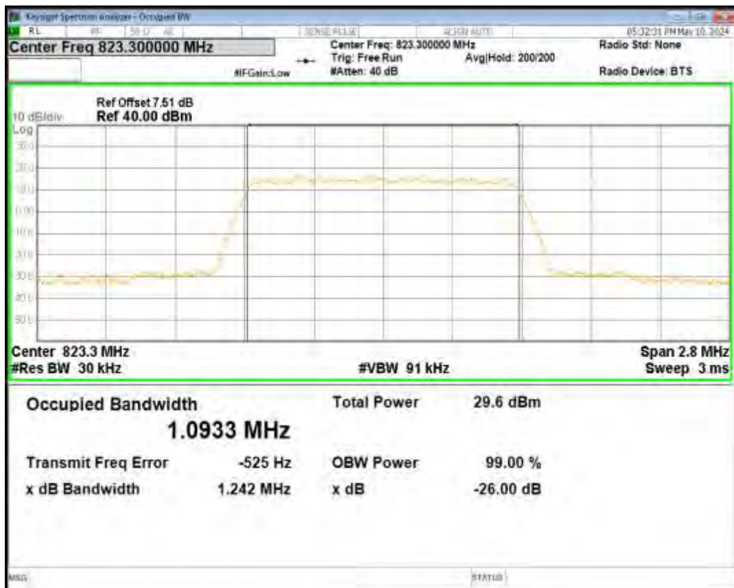
Band26(814-824) QPSK BW=10MHz Channel=26740 RB Size=50 Position=#0
