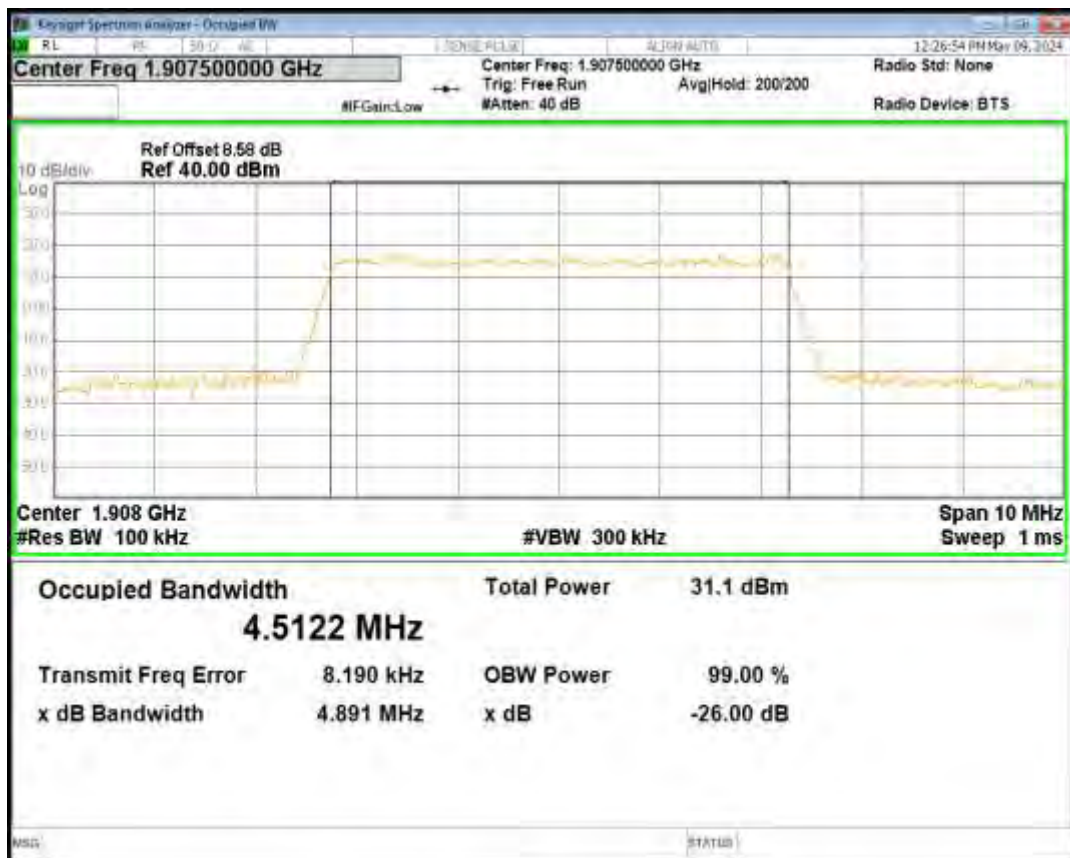
Band25 16QAM BW=1.4MHz Channel=26047 RB Size=6 Position=#0
