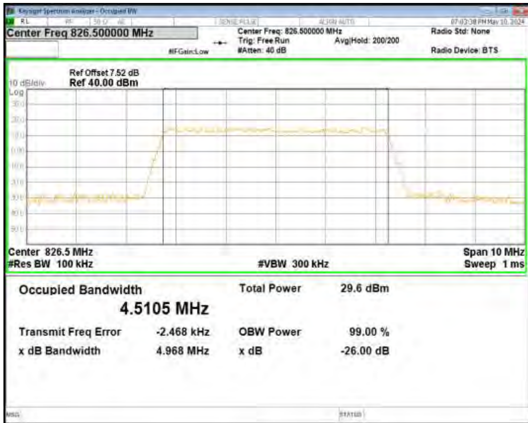
Band26(824-849) QPSK BW=5MHz Channel=27015 RB Size=25 Position=#0
