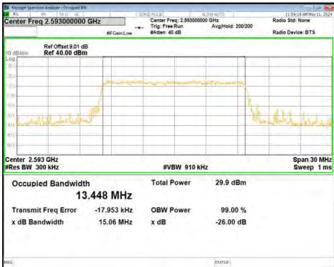
Band41 16QAM BW=5MHz Channel=41565 RB Size=25 Position=#0
