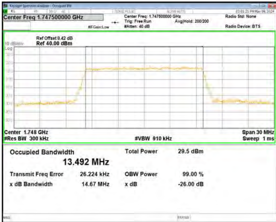
Band4 16QAM BW=20MHz Channel=20050 RB Size=100 Position=#0
