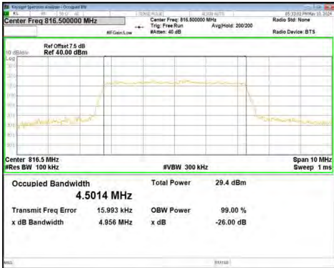
Band26(814-824) 16QAM BW=3MHz Channel=26775 RB Size=15 Position=#0
