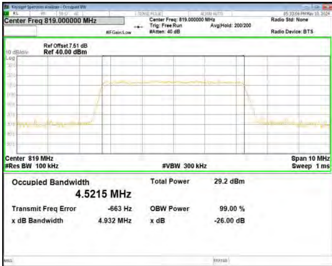
Band26(814-824) QPSK BW=1.4MHz Channel=26783 RB Size=6 Position=#0
