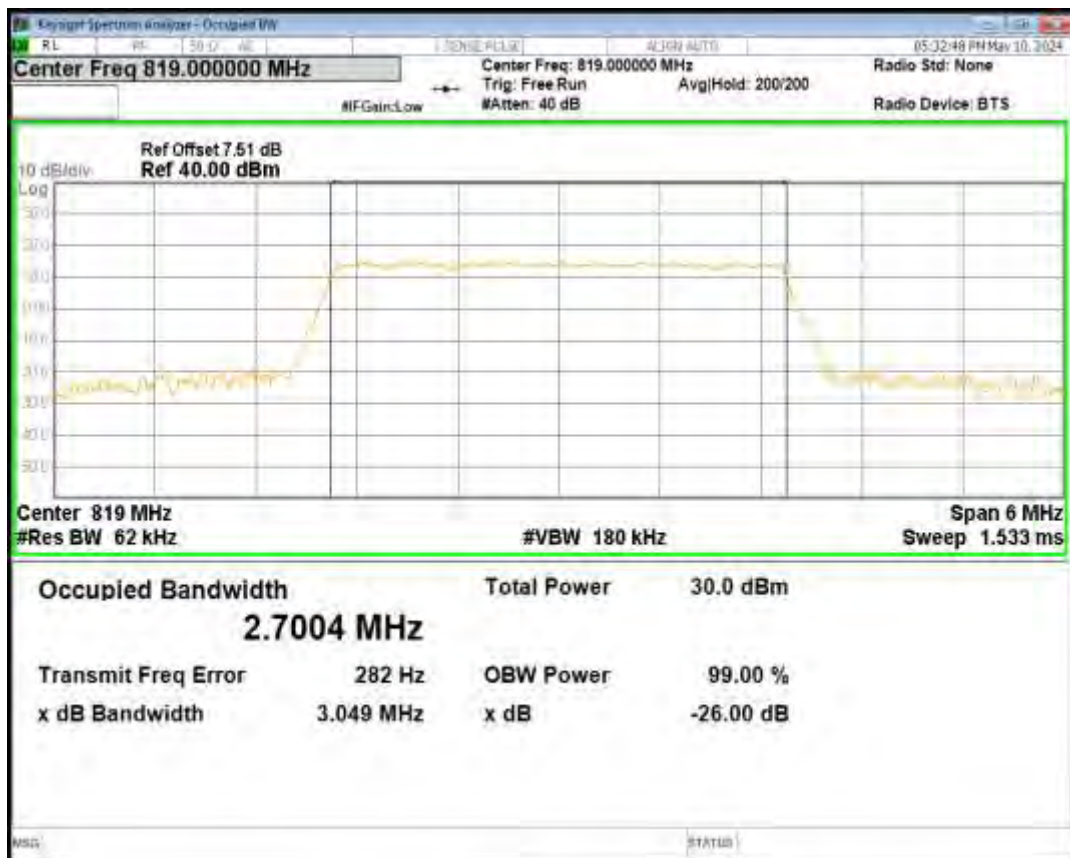
Band26(814-824) QPSK BW=5MHz Channel=26740 RB Size=25 Position=#0
