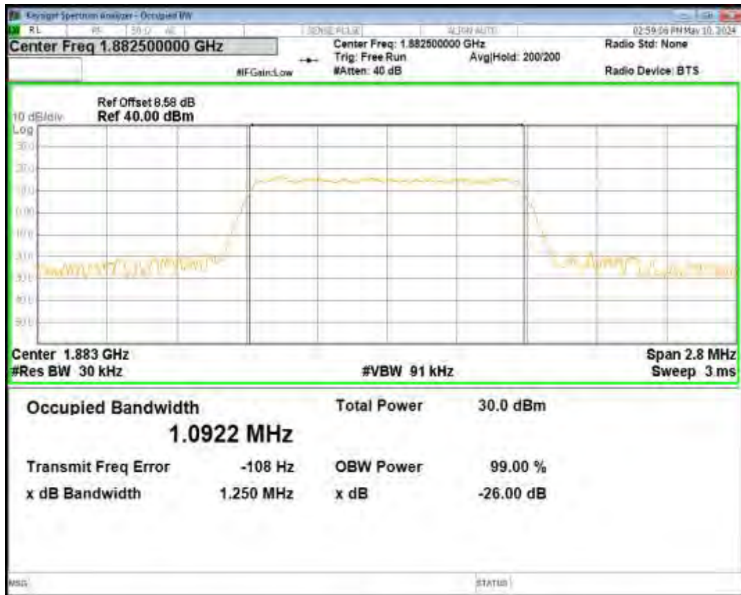
Band25 16QAM BW=5MHz Channel=26665 RB Size=25 Position=#0
