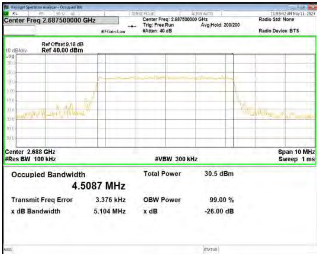
Band5 16QAM BW=1.4MHz Channel=20407 RB Size=6 Position=#0
