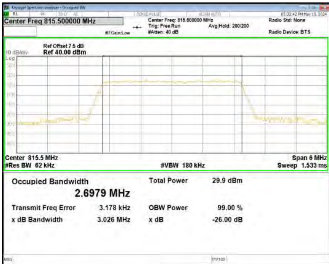
Band26(814-824) 16QAM BW=10MHz Channel=26740 RB Size=50 Position=#0
