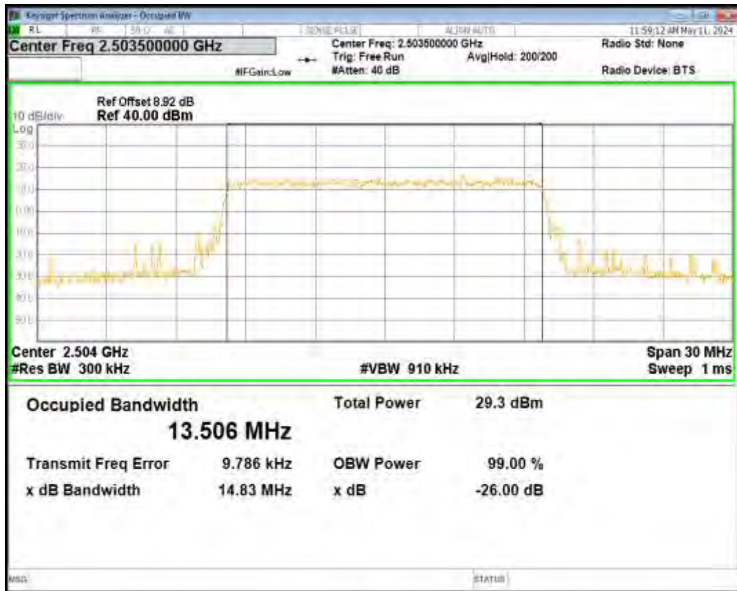
Band41 QPSK BW=5MHz Channel=41565 RB Size=25 Position=#0
