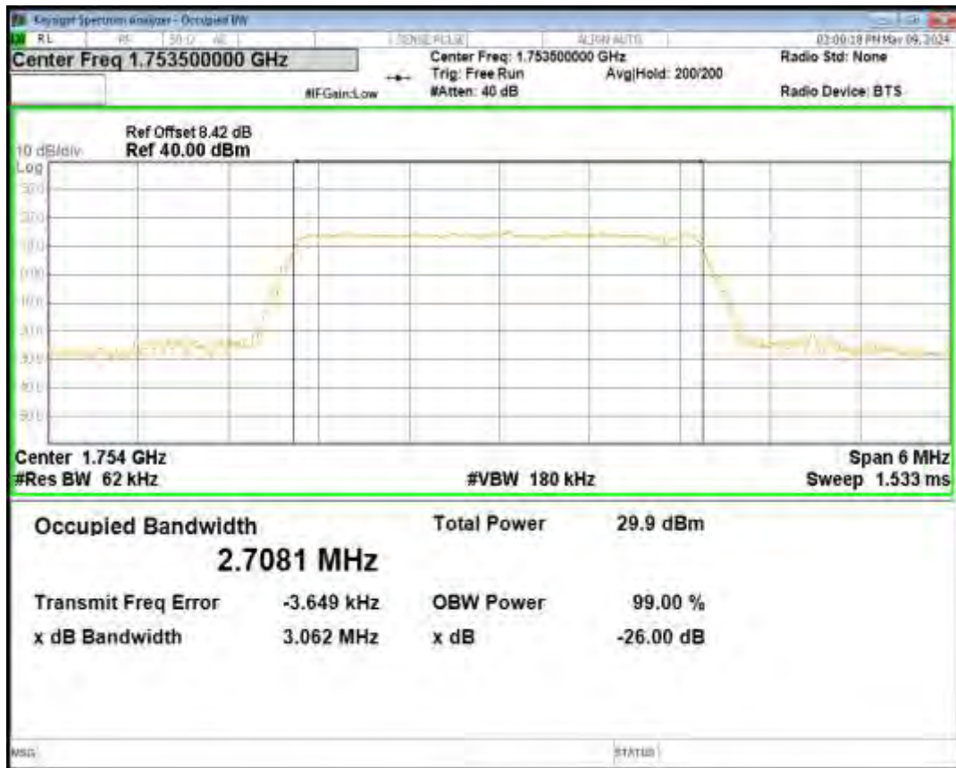
Band4 16QAM BW=5MHz Channel=20175 RB Size=25 Position=#0
