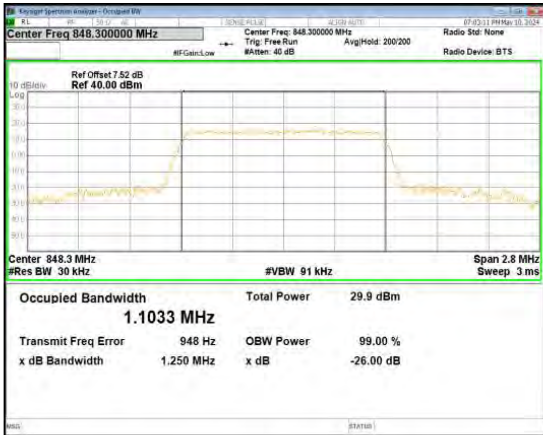
Band26(824-849) 16QAM BW=1.4MHz Channel=26915 RB Size=6 Position=#0
