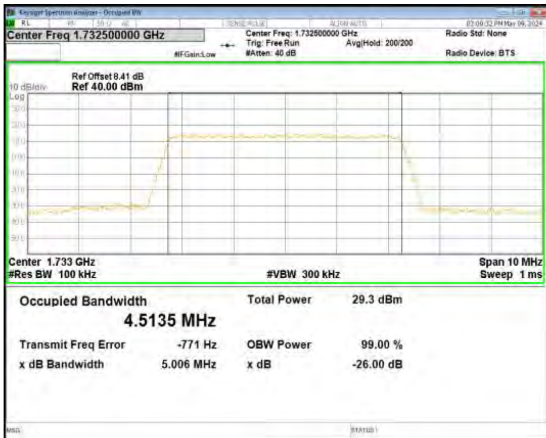
Band4 16QAM BW=5MHz Channel=20375 RB Size=25 Position=#0
