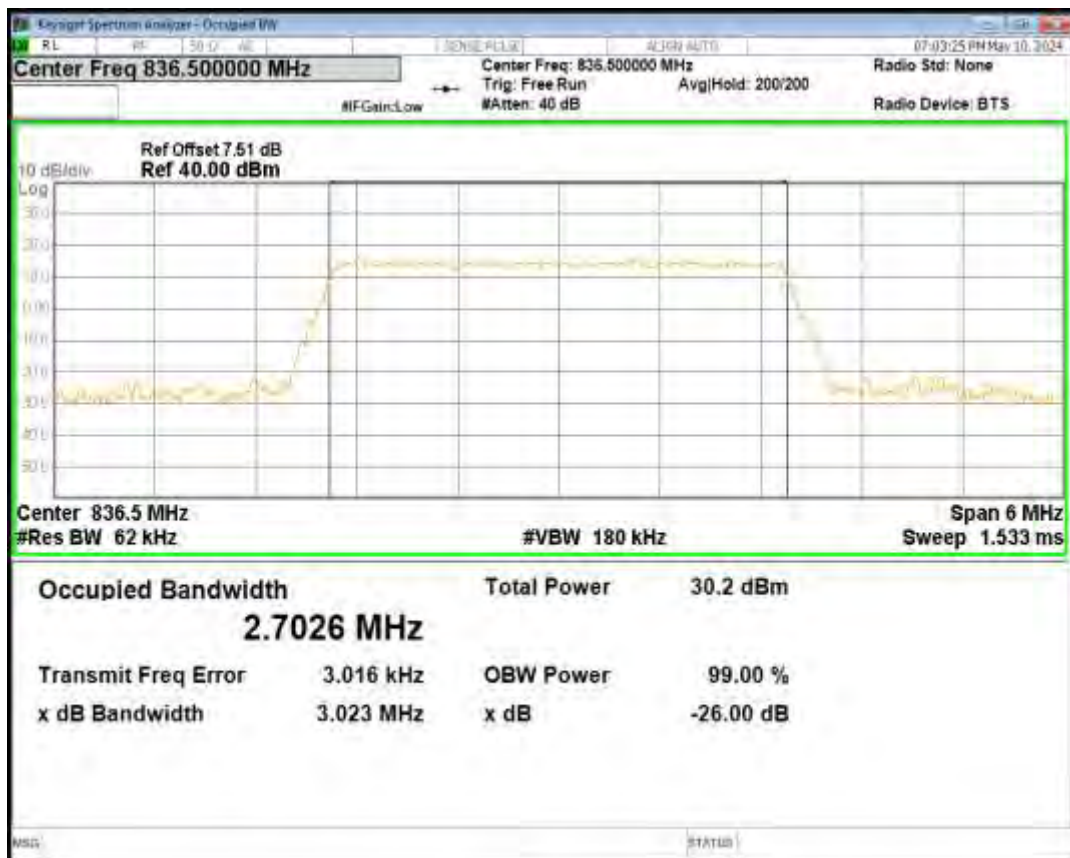
Band26(824-849) 16QAM BW=3MHz Channel=26805 RB Size=15 Position=#0
