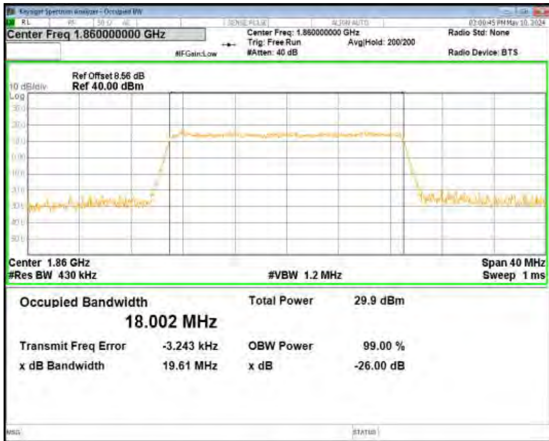
Band25 QPSK BW=20MHz Channel=26365 RB Size=100 Position=#0
