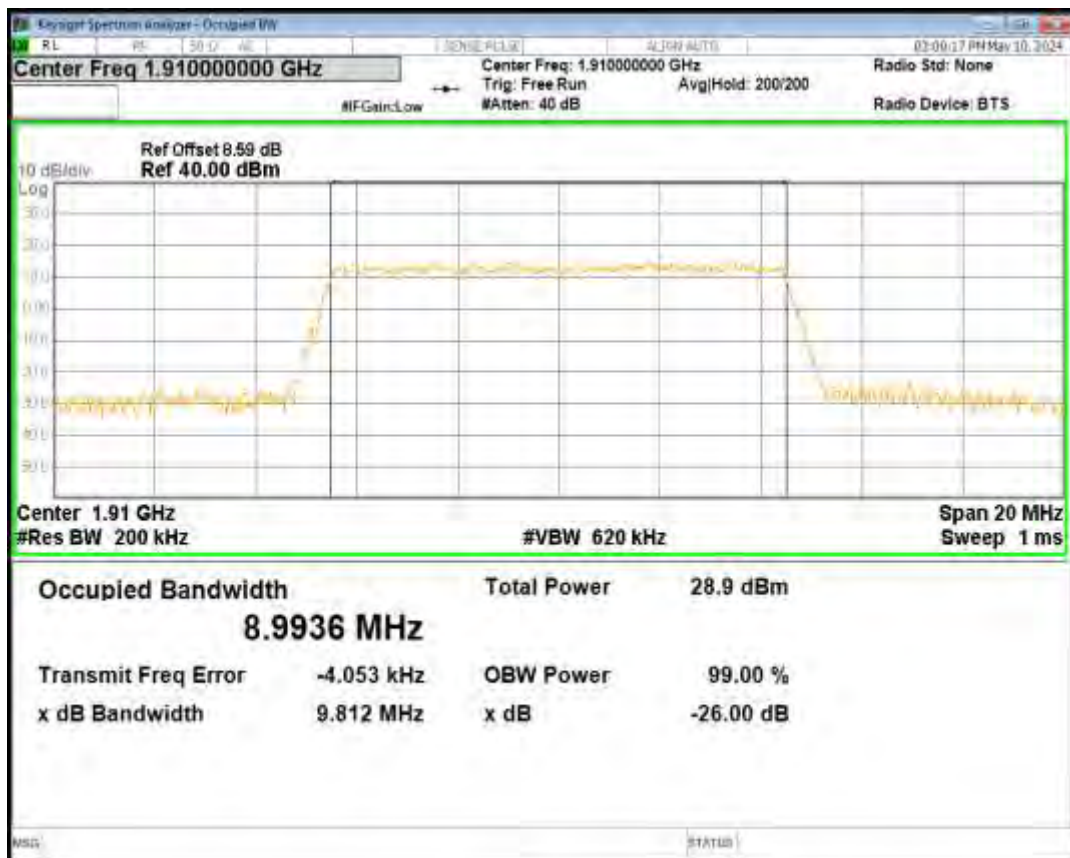
Band25 16QAM BW=10MHz Channel=26365 RB Size=50 Position=#0
