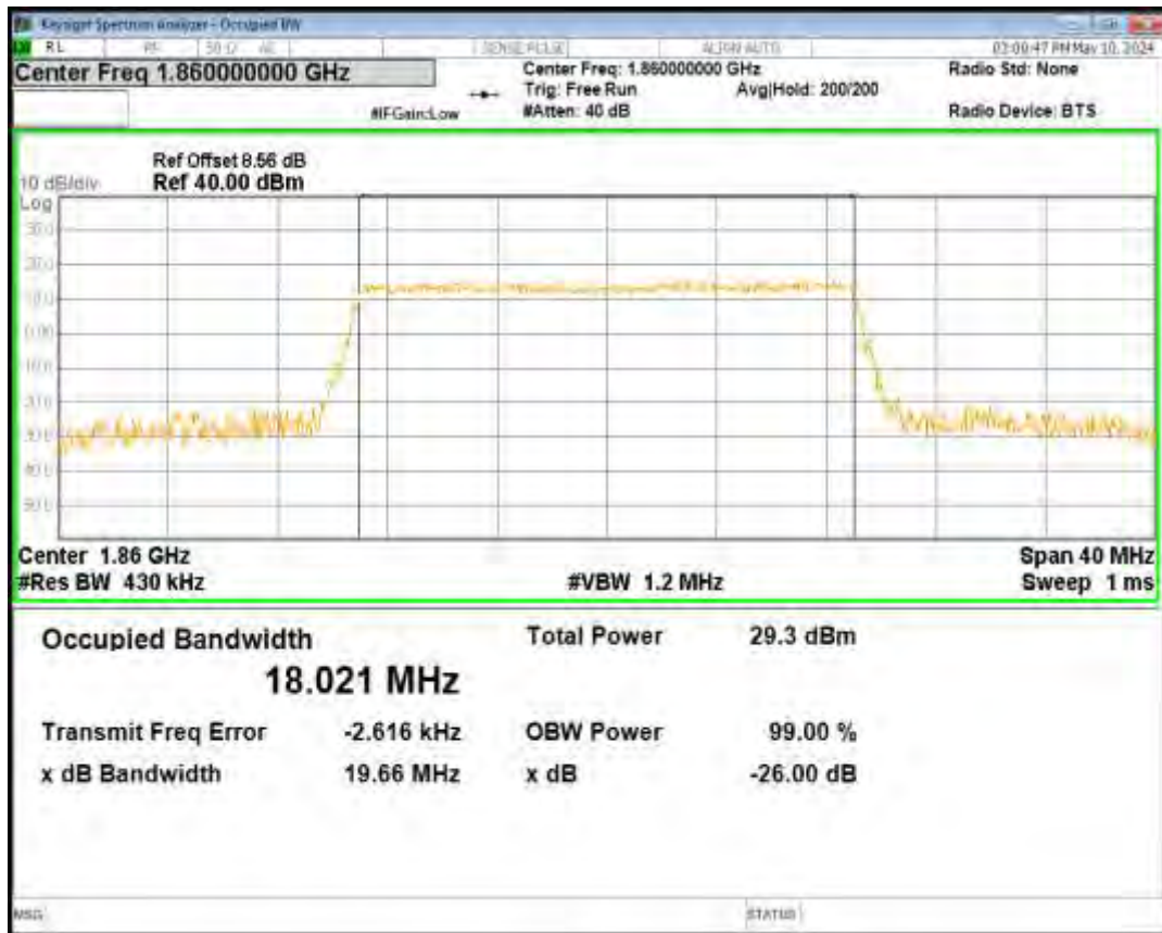
Band25 16QAM BW=10MHz Channel=26640 RB Size=50 Position=#0
