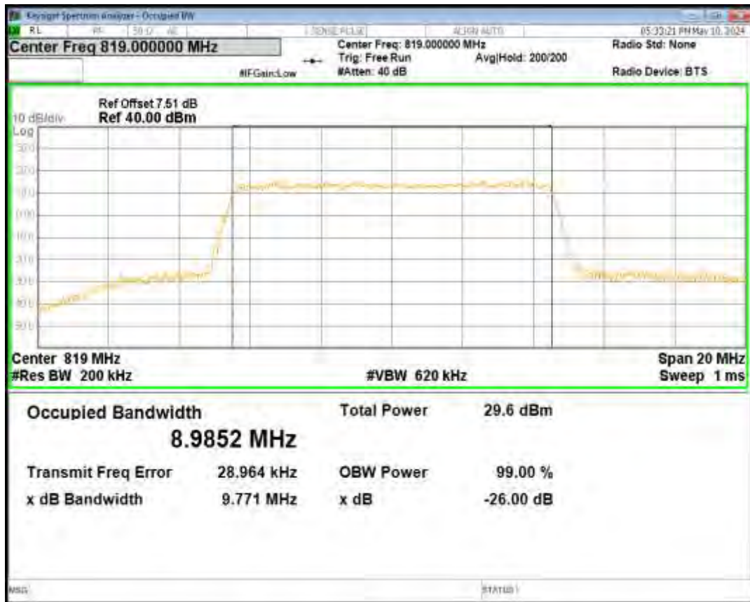
Band26(814-824) QPSK BW=3MHz Channel=26705 RB Size=15 Position=#0
