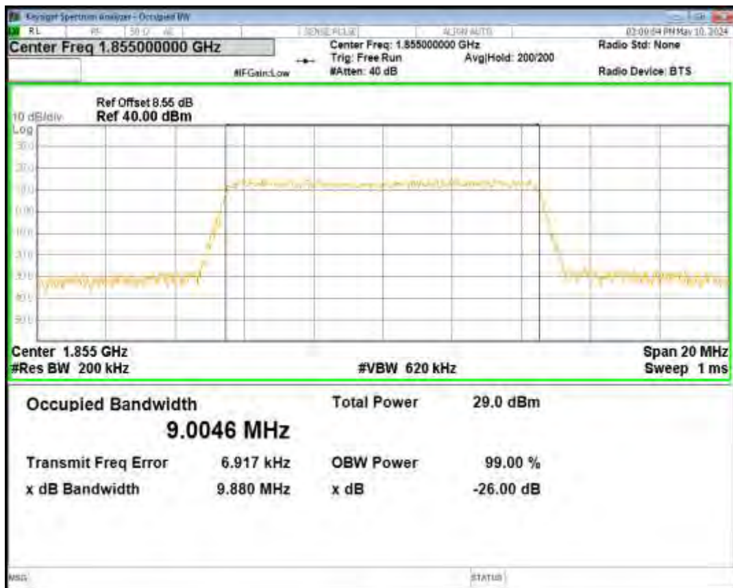
Band25 16QAM BW=1.4MHz Channel=26683 RB Size=6 Position=#0
