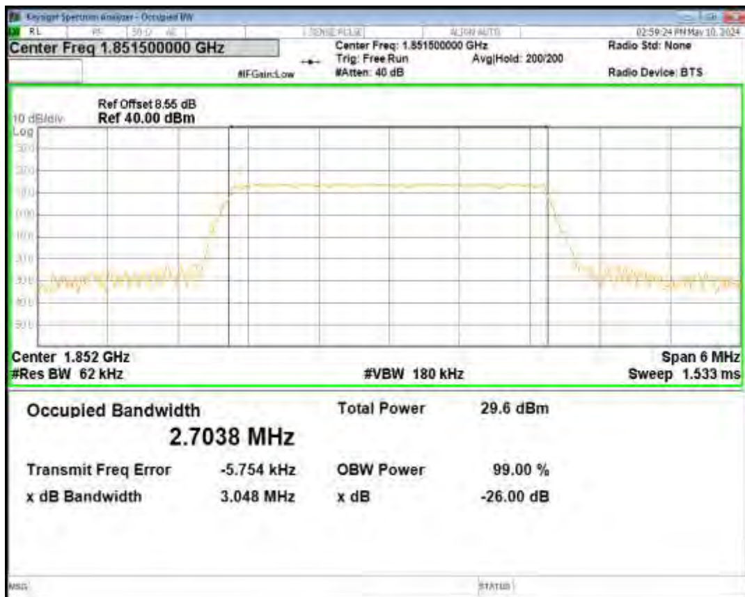
Band25 16QAM BW=20MHz Channel=26590 RB Size=100 Position=#0
