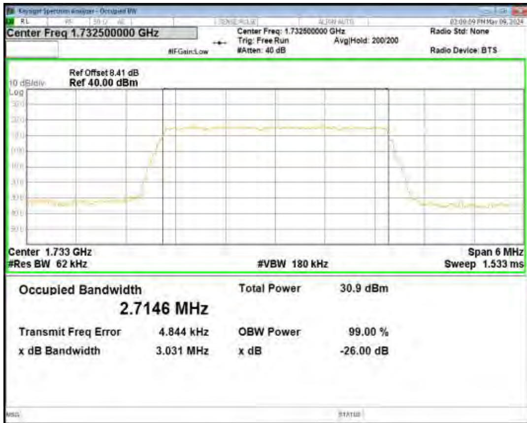
Band4 QPSK BW=3MHz Channel=19965 RB Size=15 Position=#0
