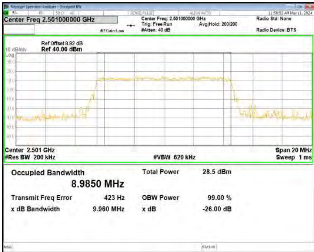
Band41 16QAM BW=10MHz Channel=40620 RB Size=50 Position=#0
