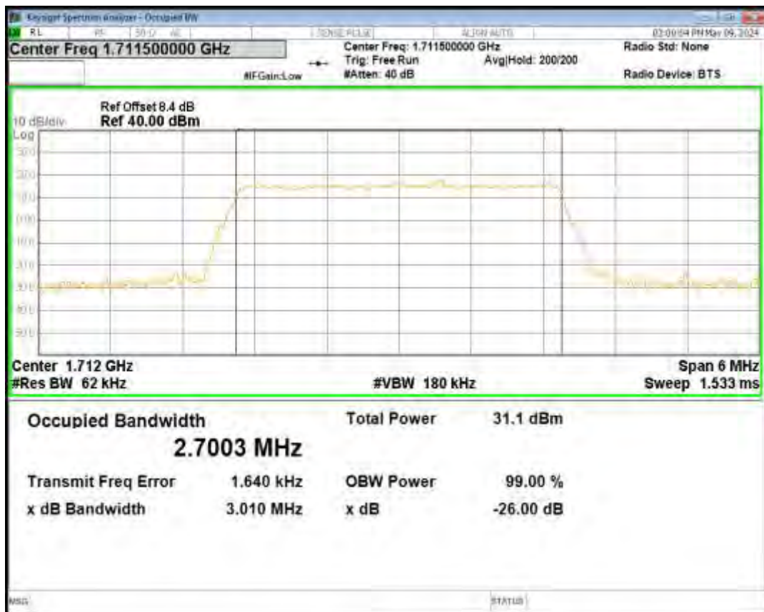
Band4 QPSK BW=20MHz Channel=20300 RB Size=100 Position=#0
