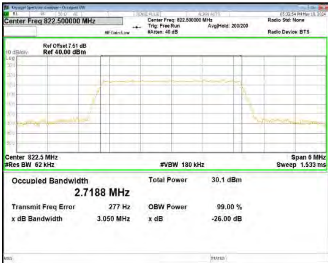
Band26(814-824) 16QAM BW=5MHz Channel=26765 RB Size=25 Position=#0
