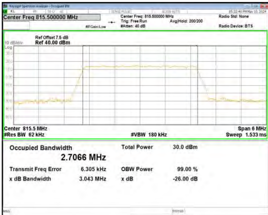
Band26(814-824) QPSK BW=3MHz Channel=26740 RB Size=15 Position=#0
