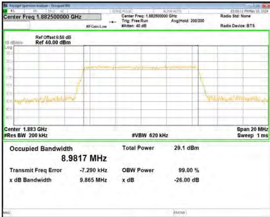
Band25 16QAM BW=10MHz Channel=26090 RB Size=50 Position=#0
