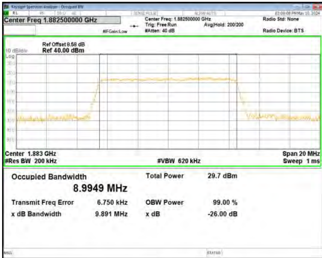
Band25 QPSK BW=10MHz Channel=26090 RB Size=50 Position=#0
