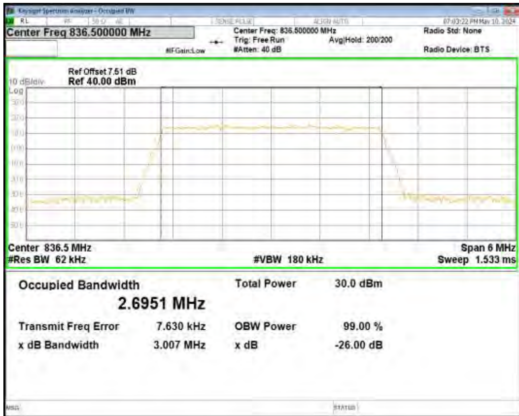
Band26(824-849) QPSK BW=3MHz Channel=27025 RB Size=15 Position=#0
