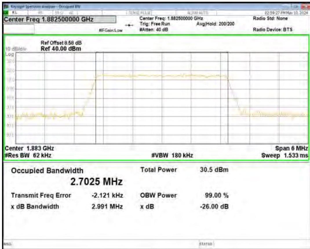
Band25 QPSK BW=3MHz Channel=26675 RB Size=15 Position=#0
