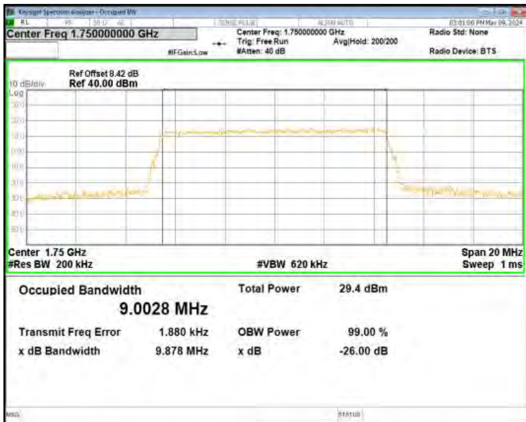
Band4 16QAM BW=15MHz Channel=20025 RB Size=75 Position=#0
