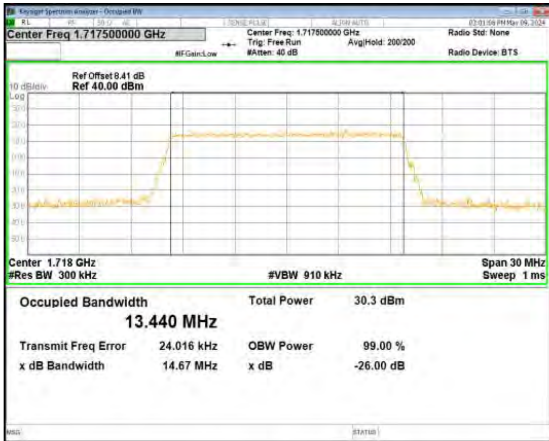
Band4 QPSK BW=10MHz Channel=20350 RB Size=50 Position=#0
