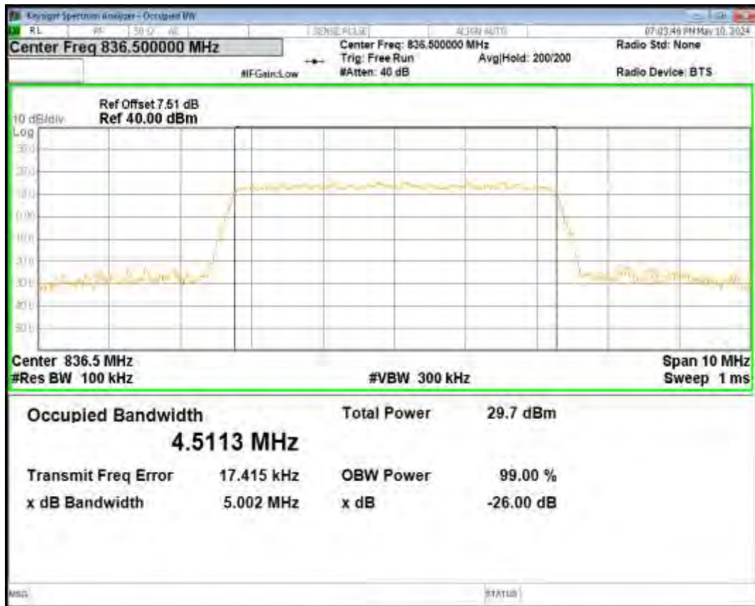
Band26(824-849) 16QAM BW=5MHz Channel=26815 RB Size=25 Position=#0
