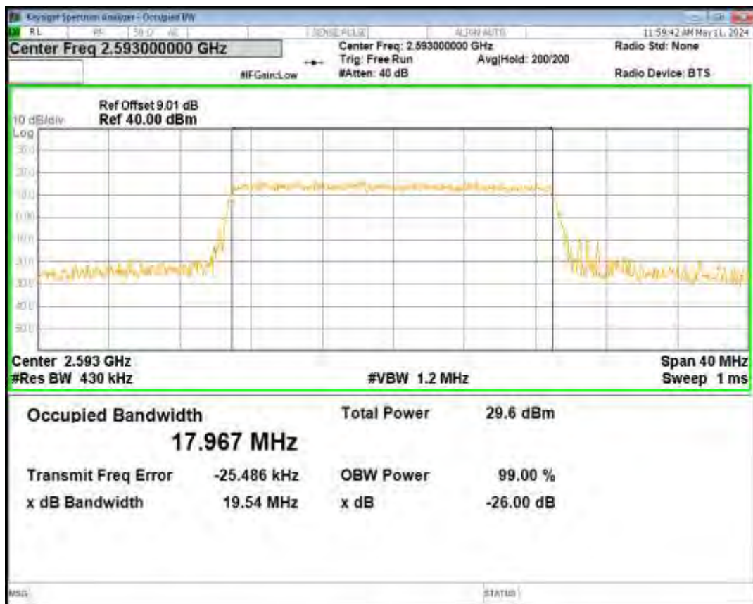
Band41 16QAM BW=20MHz Channel=41490 RB Size=100 Position=#0
