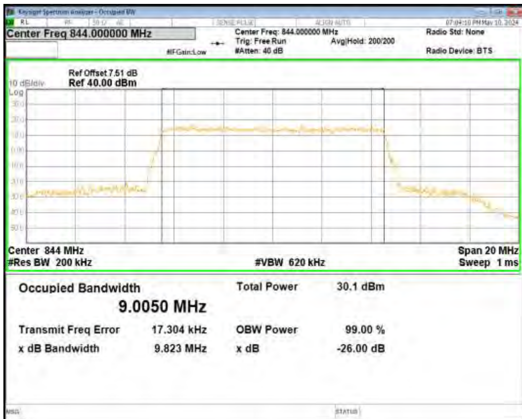
Band26(824-849) QPSK BW=10MHz Channel=26840 RB Size=50 Position=#0
