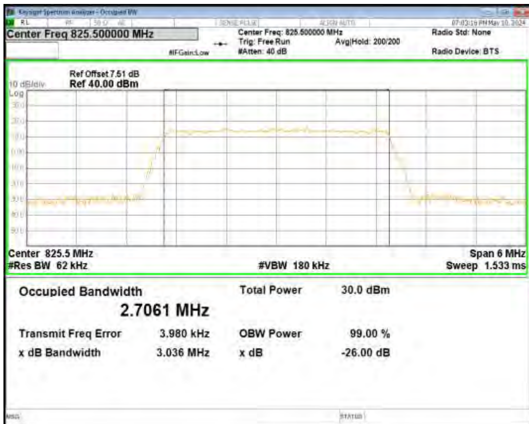
Band26(824-849) QPSK BW=3MHz Channel=26915 RB Size=15 Position=#0
