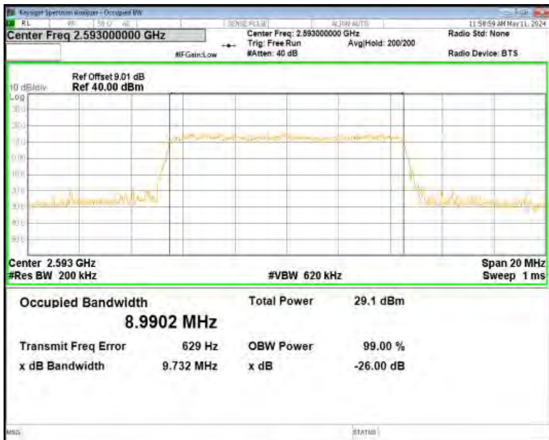
Band41 16QAM BW=10MHz Channel=41540 RB Size=50 Position=#0
