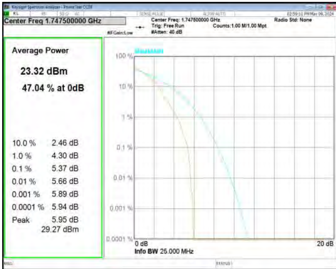
Band4 QPSK BW=15MHz Channel=20175 RB Size=1 Position=#0
