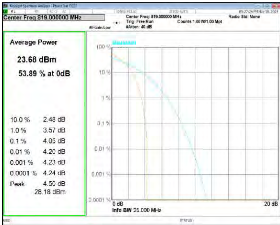
Band26(814-824) QPSK BW=1.4MHz Channel=26697 RB Size=1 Position=#0
