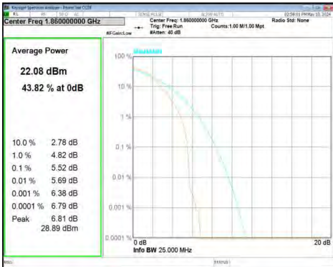
Band25 16QAM BW=20MHz Channel=26365 RB Size=1 Position=#0
