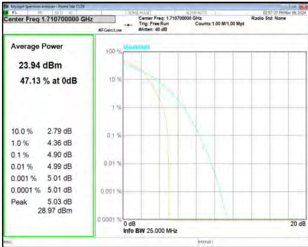
Band4 16QAM BW=1.4MHz Channel=20175 RB Size=1 Position=#0
