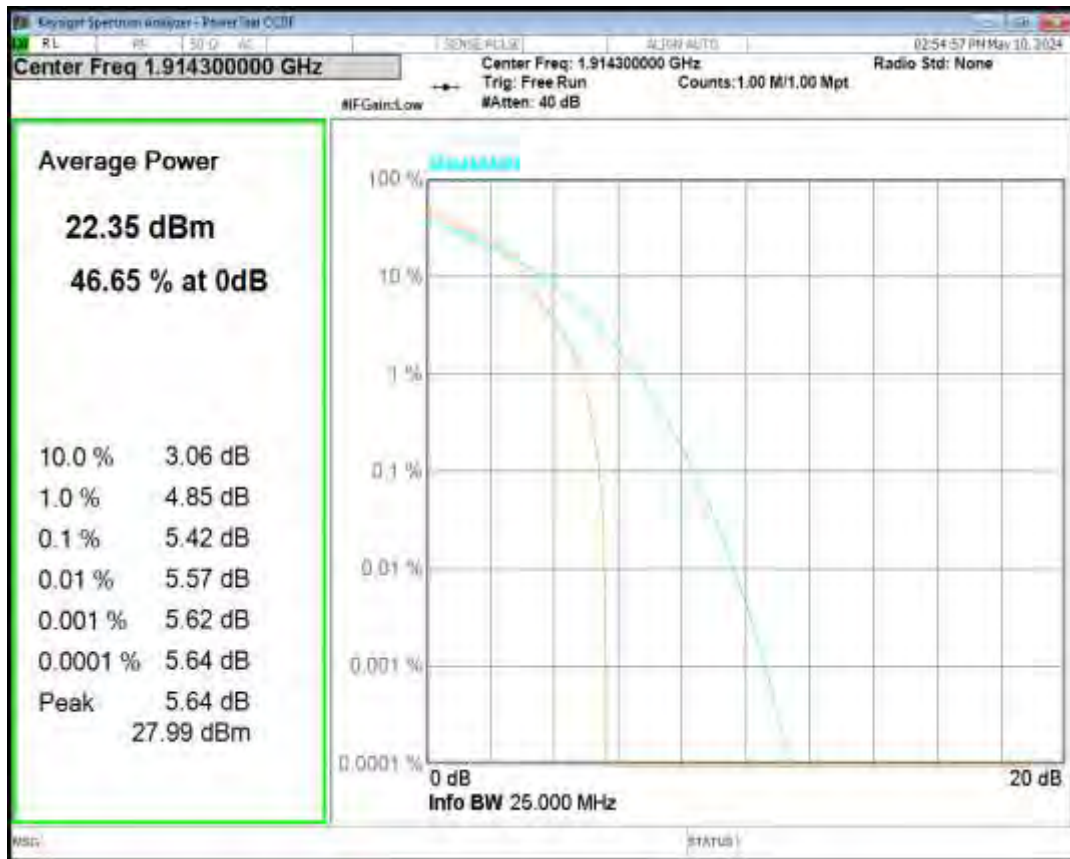
Band25 16QAM BW=3MHz Channel=26675 RB Size=1 Position=#0
