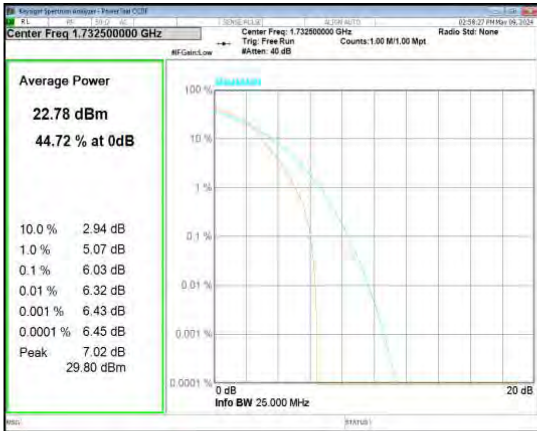
Band4 16QAM BW=5MHz Channel=19975 RB Size=1 Position=#0
