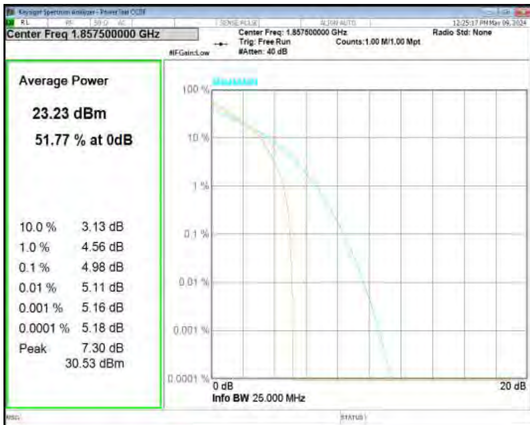
Band2 QPSK BW=10MHz Channel=18900 RB Size=1 Position=#0
