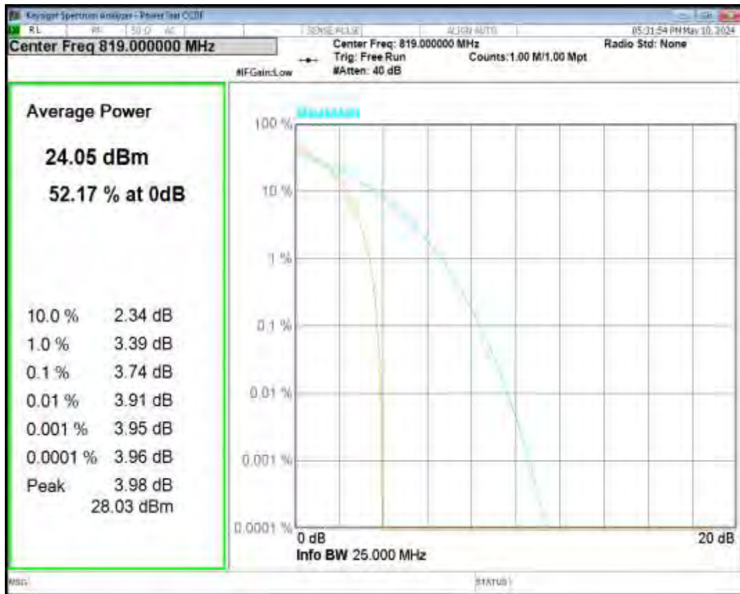
Band26(814-824) QPSK BW=5MHz Channel=26765 RB Size=1 Position=#0
