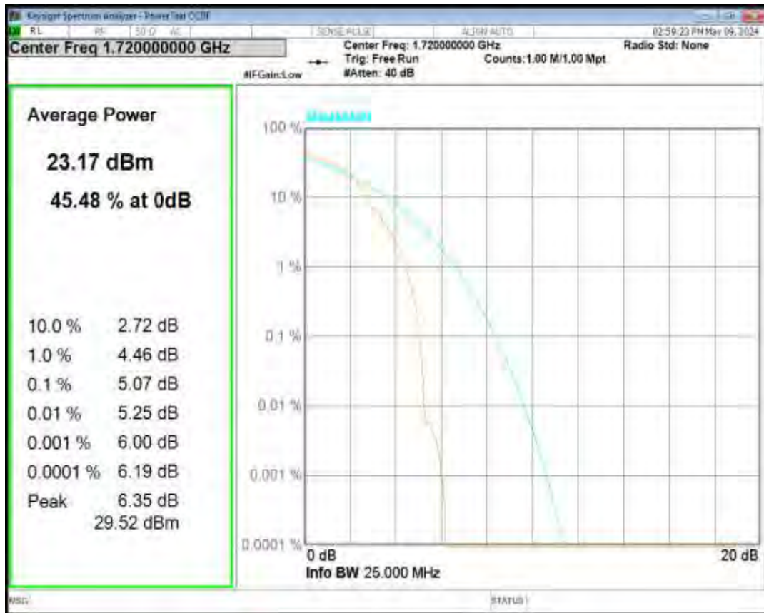
Band4 16QAM BW=20MHz Channel=20175 RB Size=1 Position=#0
