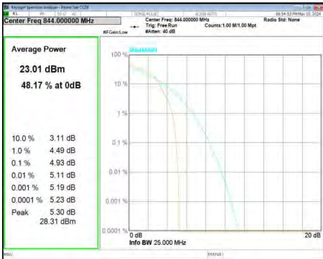
Band26(824-849) 16QAM BW=15MHz Channel=26865 RB Size=1 Position=#0
