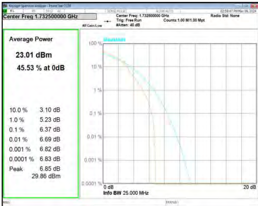
Band4 16QAM BW=15MHz Channel=20325 RB Size=1 Position=#0
