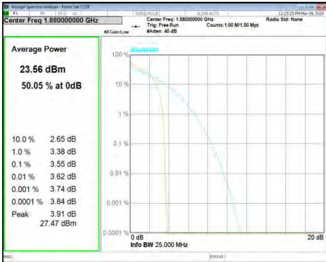
Band2 16QAM BW=15MHz Channel=18675 RB Size=1 Position=#0
