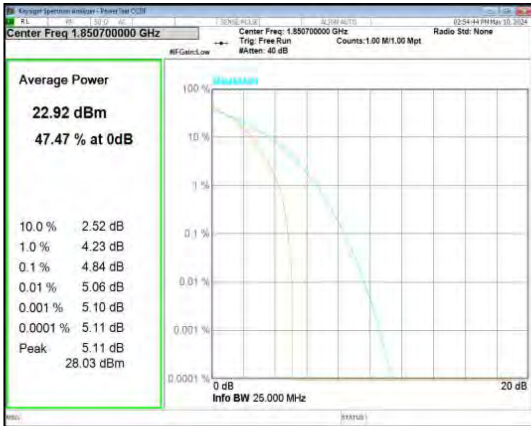
Band25 16QAM BW=5MHz Channel=26365 RB Size=1 Position=#0
