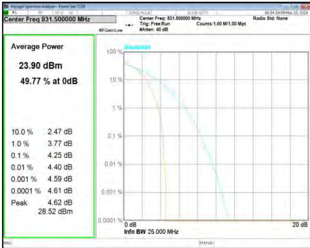
Band26(824-849) QPSK BW=10MHz Channel=26990 RB Size=1 Position=#0
