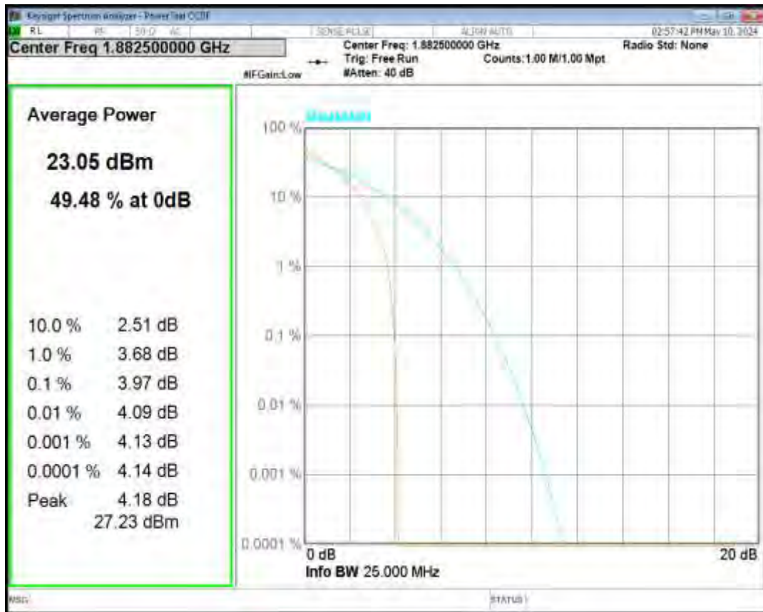
Band25 QPSK BW=15MHz Channel=26115 RB Size=1 Position=#0
