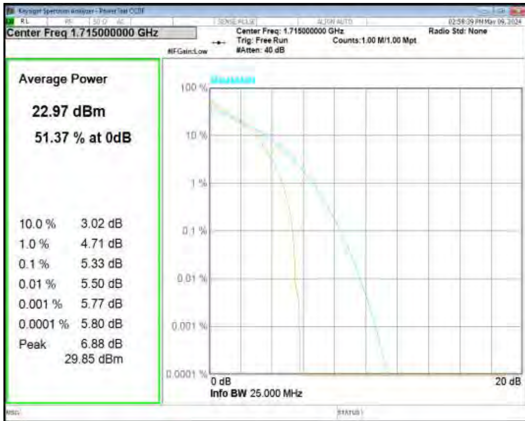
Band4 16QAM BW=5MHz Channel=20375 RB Size=1 Position=#0
