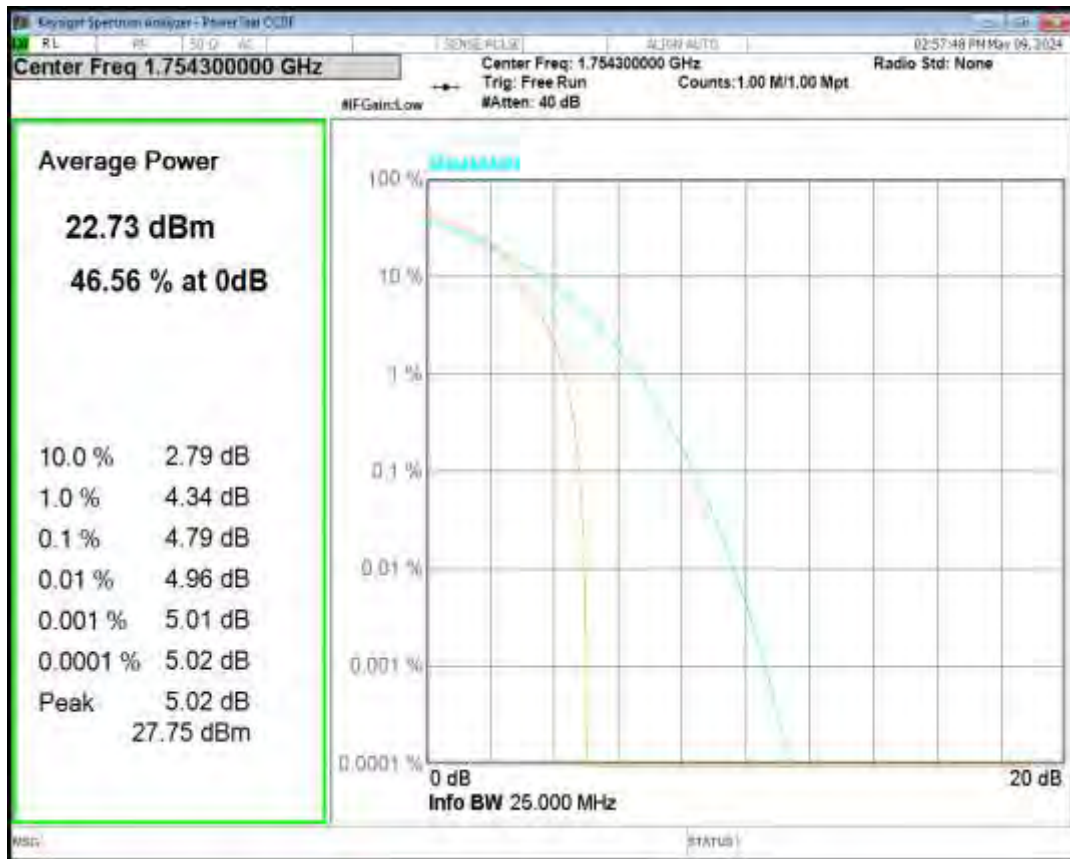
Band4 16QAM BW=10MHz Channel=20000 RB Size=1 Position=#0
