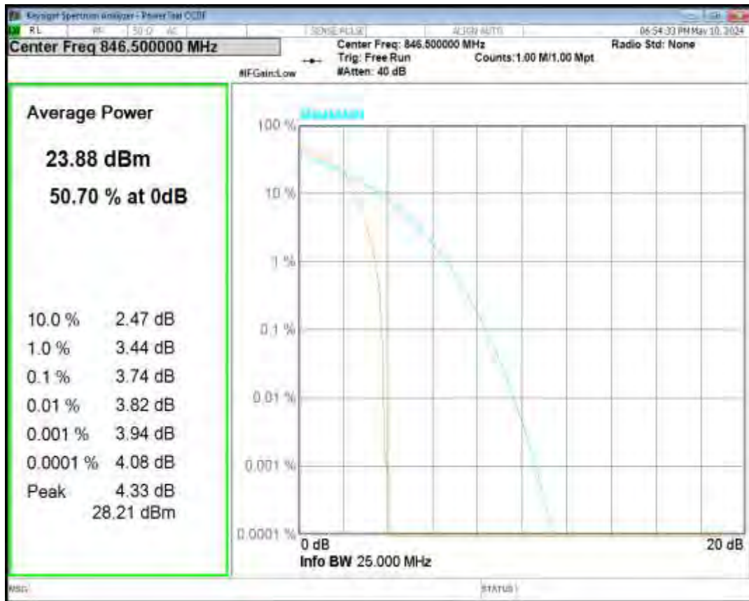
Band26(824-849) 16QAM BW=5MHz Channel=26915 RB Size=1 Position=#0
