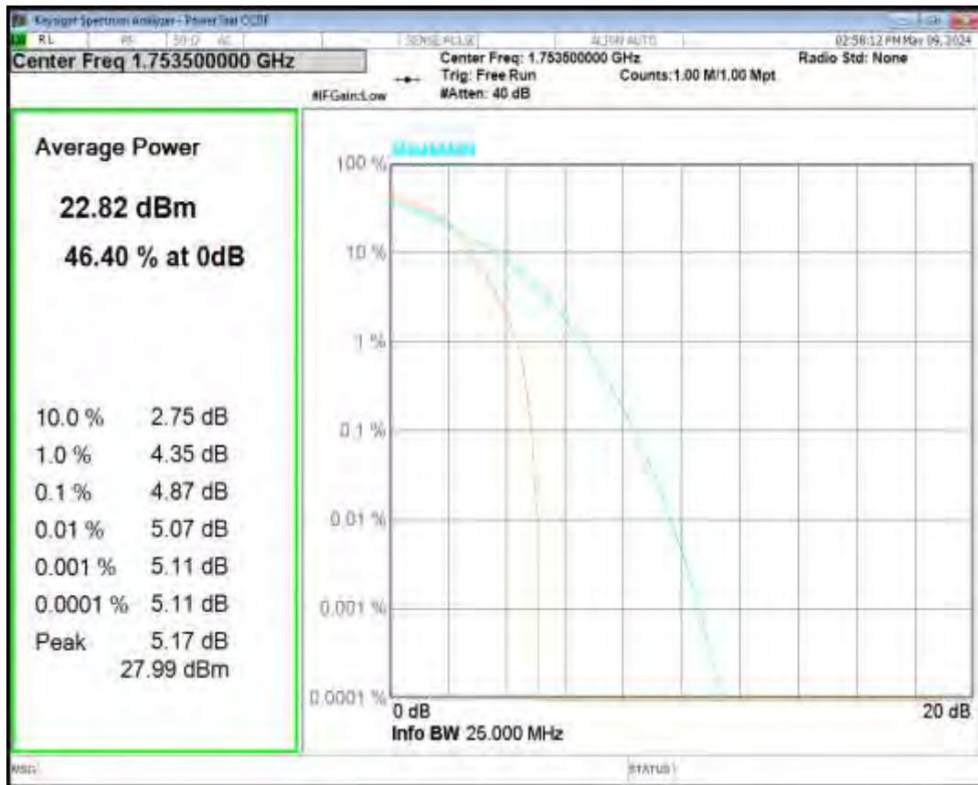
Band4 16QAM BW=3MHz Channel=20175 RB Size=1 Position=#0
