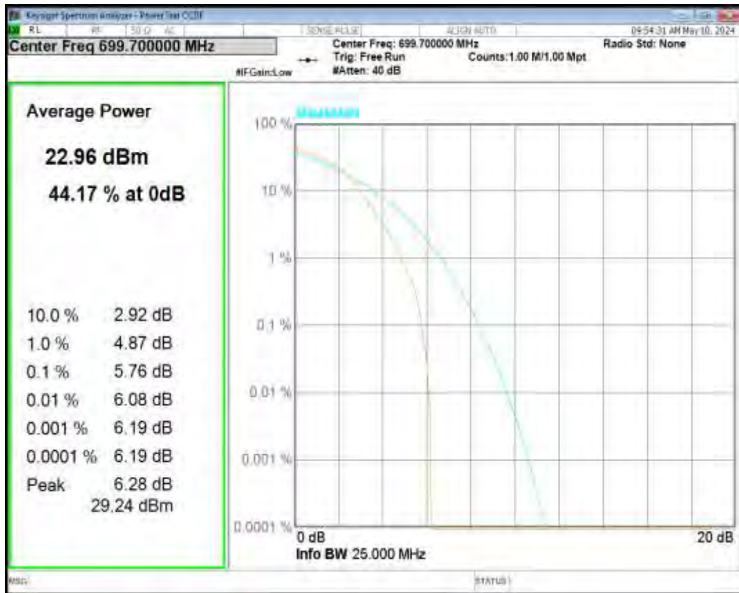
Band12 16QAM BW=1.4MHz Channel=23095 RB Size=1 Position=#0
