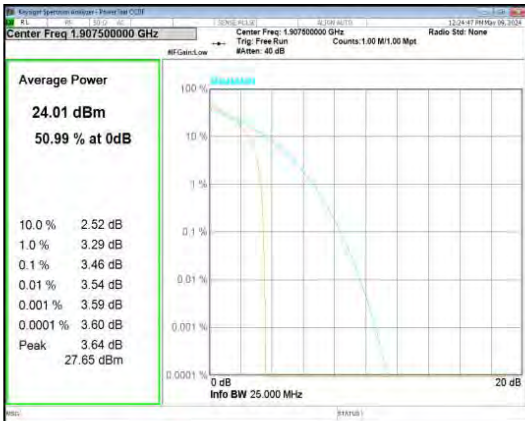
Band25 16QAM BW=1.4MHz Channel=26047 RB Size=1 Position=#0
