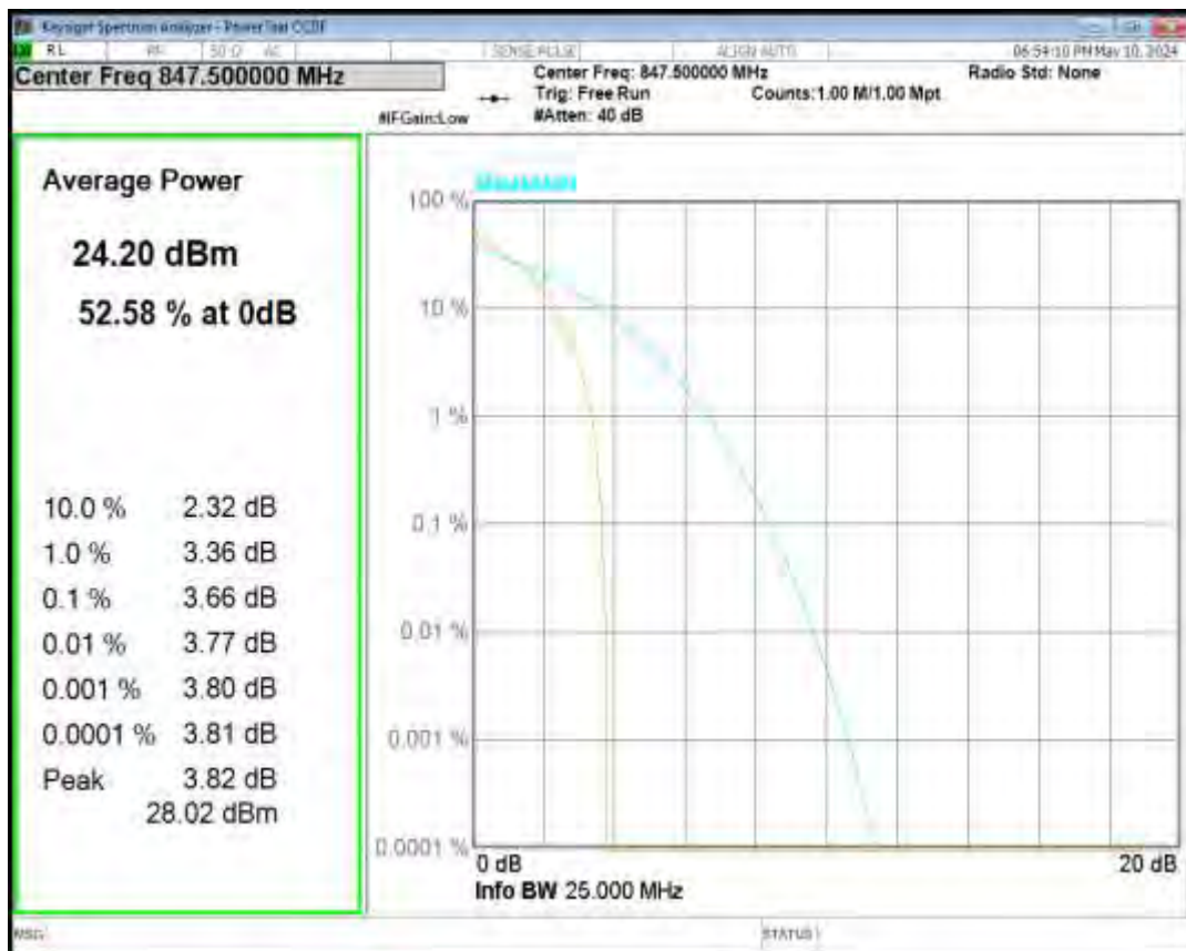
Band26(824-849) QPSK BW=5MHz Channel=26815 RB Size=1 Position=#0
