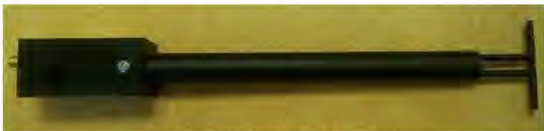
Figure 1 – MVG COMOSAR Validation Dipole
