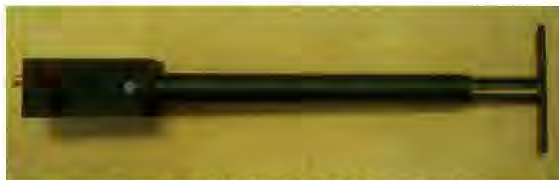
Figure 1 – MVG COMOSAR Validation Dipole
