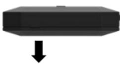
Remove the hotspot back cover by lifting the notch on the corner of the device. If the battery is present, remove it.
