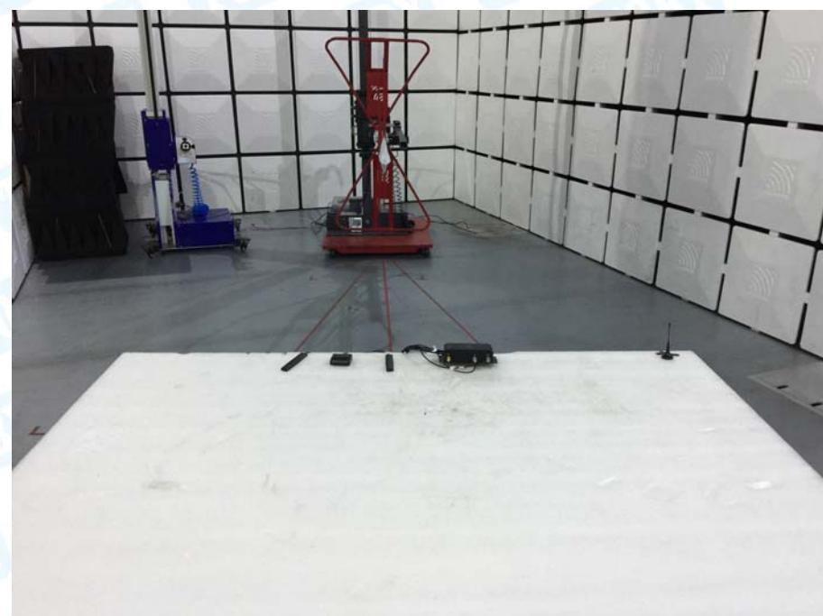
**FCC Part 15C Test Setup****Photo of Setup for Radiated Emission (Above 1 GHz)**
