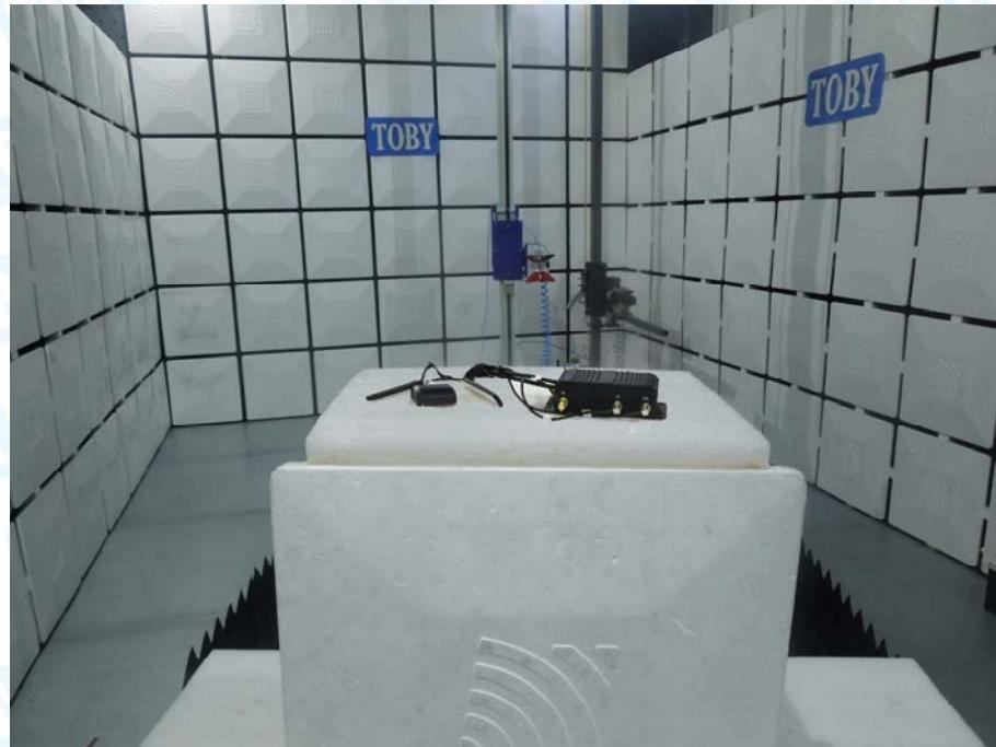
**Photo of Setup for Radiated Emission (Below 1 GHz)**
