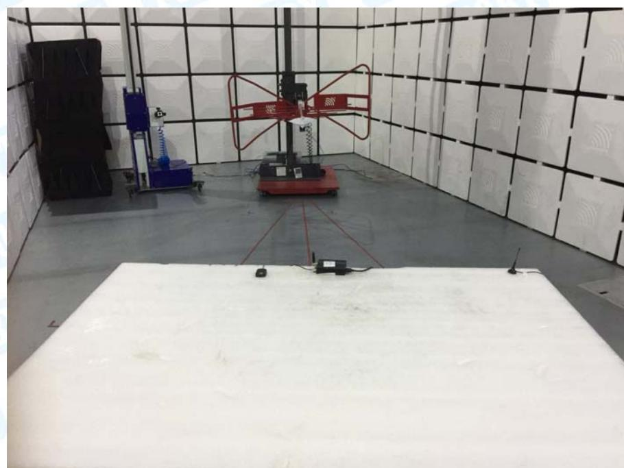
**Photo of Setup for Radiated Emission**
