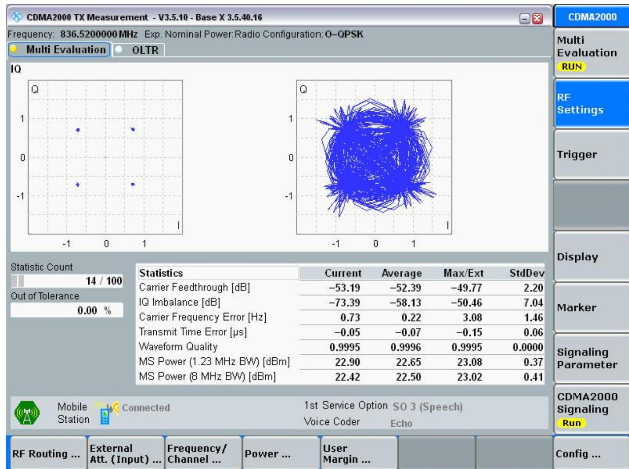
**3.1.2 Test Band = CDMA BC1****3.1.2.1 Test Mode = CDMA /TM1****3.1.2.1.1 Test Channel = MCH**
