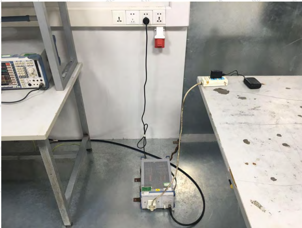
Photo of Conducted Emission Measurement
