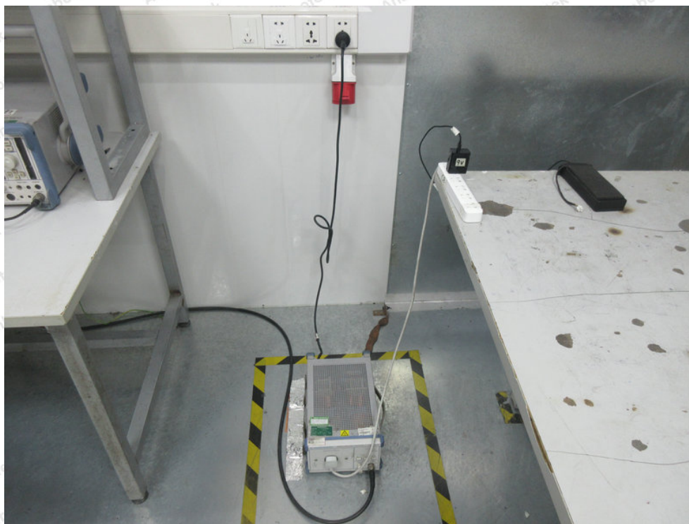
Photo of Power Line Conducted Emission Test
