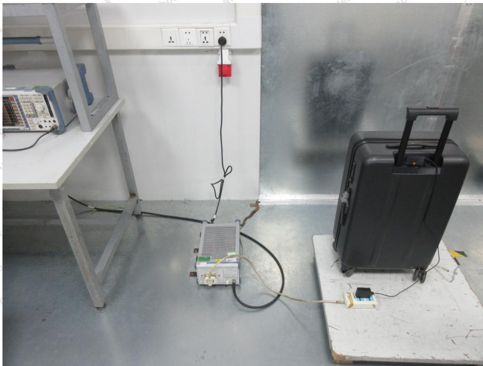
Photo of Power Line Conducted Emission Test
