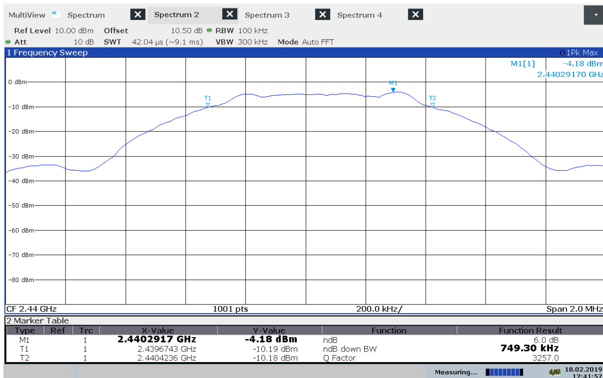
DTS Bandwidth, 2440 MHz
