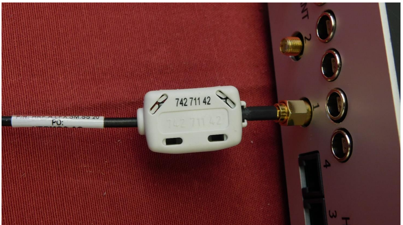
Picture 6: Antenna cable with ferrite
