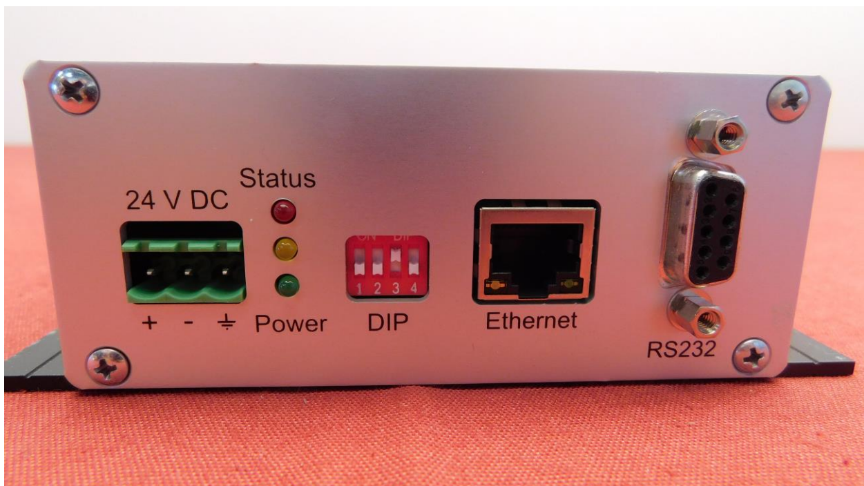
Picture 4: Ports – front view
