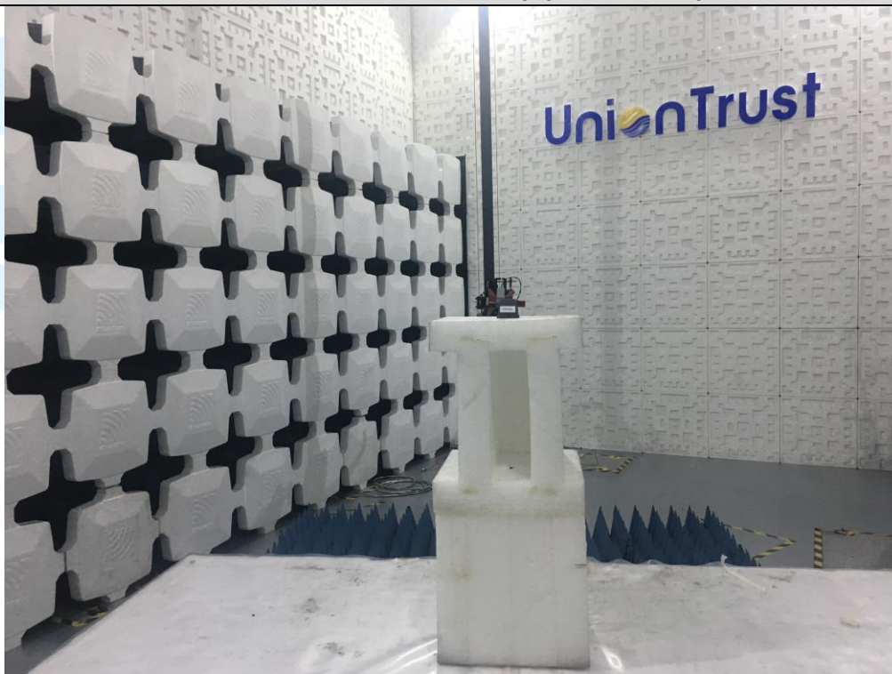
Radiated emission Test Setup (Above 1 GHz)
