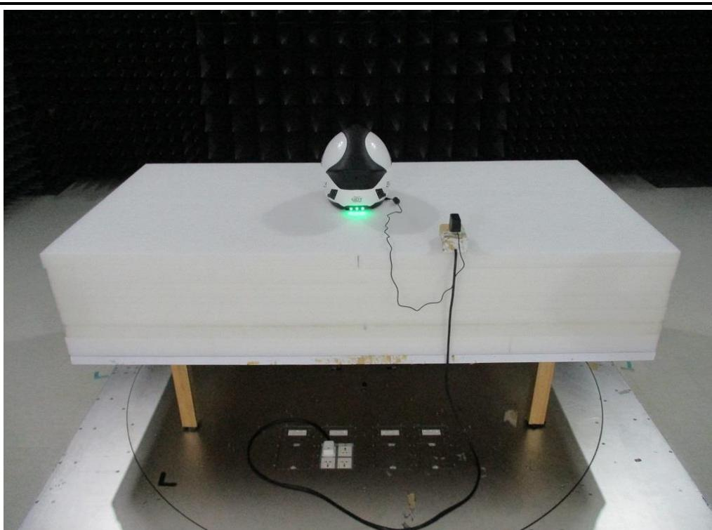
**Radiated Emission Above 1GHz Test**
