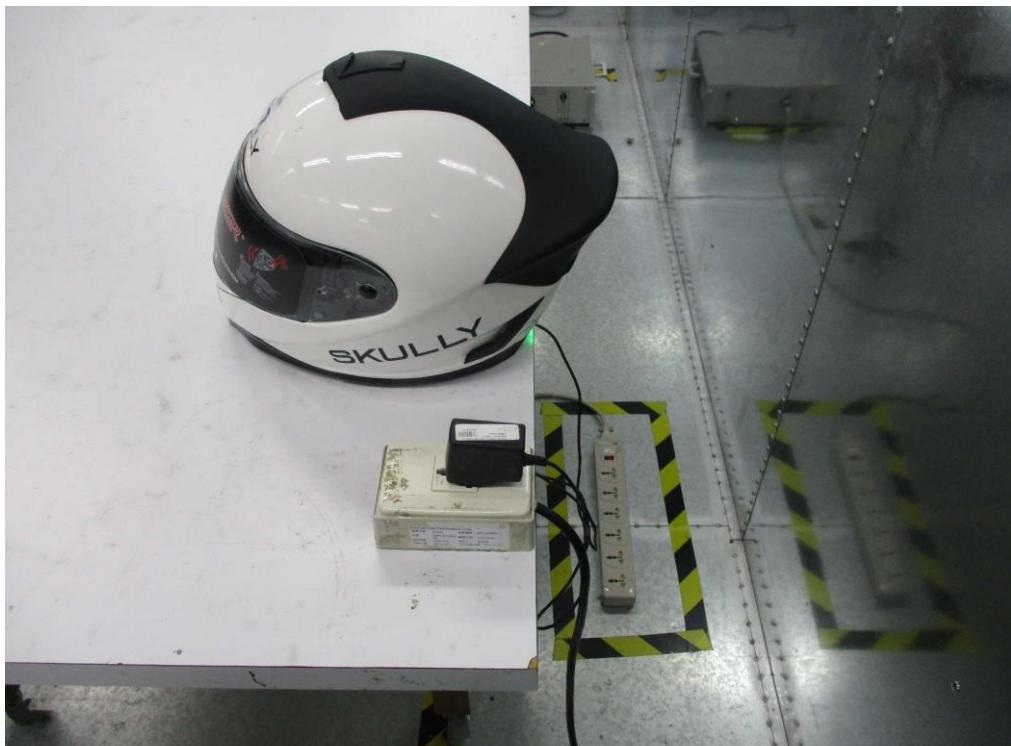
**Radiated Emission Below 1GHz Test (Battery Mode)**
