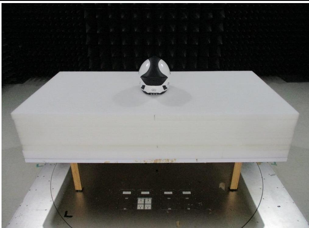
**Radiated Emission Below 1GHz Test (Charge Mode)**
