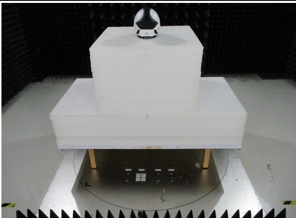
**Radiated Emission Above 1GHz Test**
