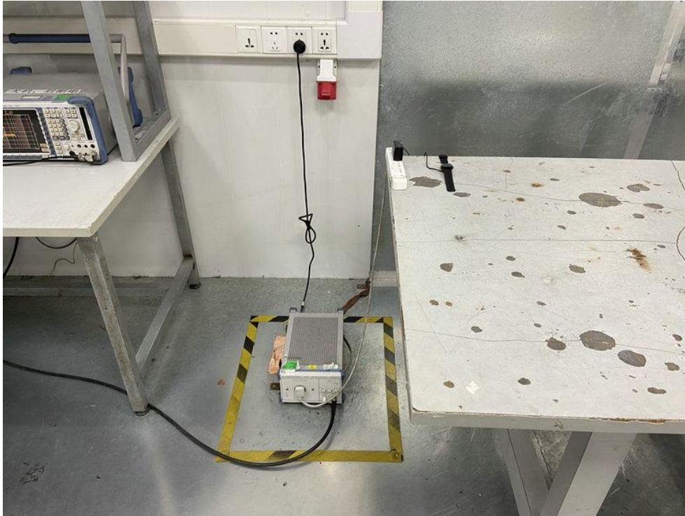
Photo of Conducted Emission Measurement
