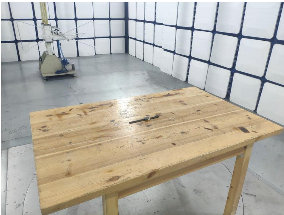
Photo of Radiation Emission Test
