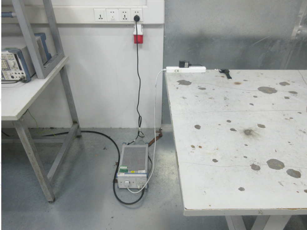
Photo of Conducted Emission Measurement
