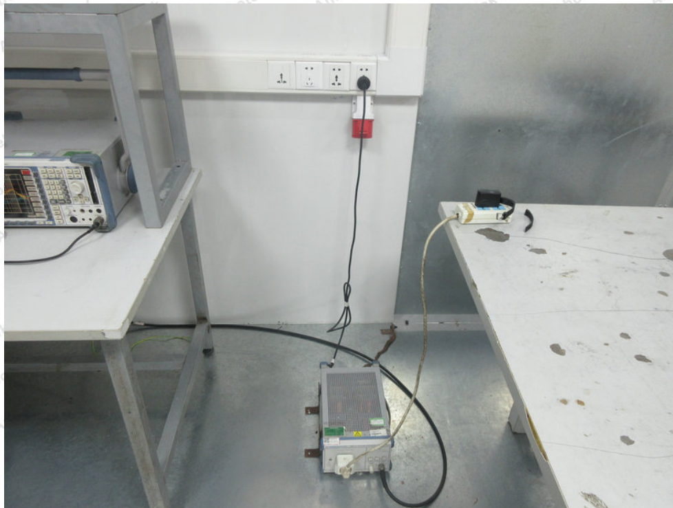
Photo of Conducted Emission Test
