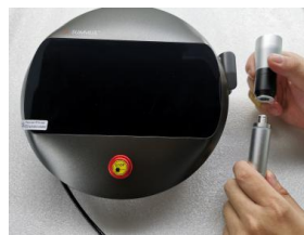
Select the treating head, and connect to base of hand piece.
