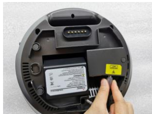
Insert fiber into laser port and screw it until fastened tight.
