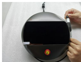
Remove black protective cap and place into case.
