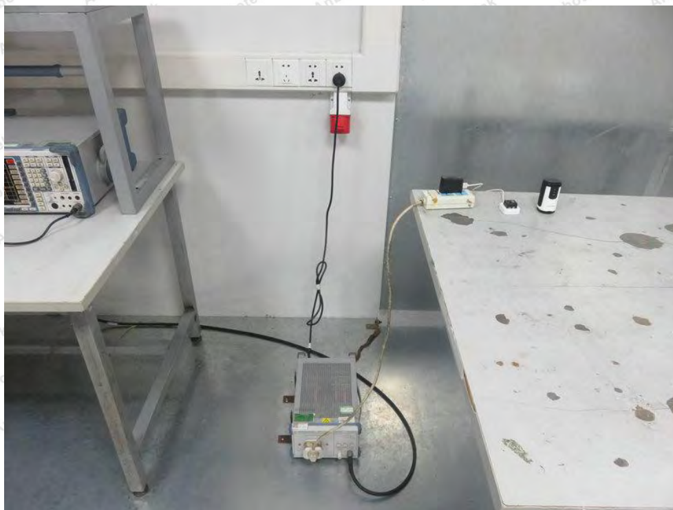
Photo of Conducted Emission Test
