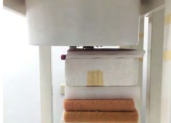
Fig.3 EUT Back side to flat phantom
