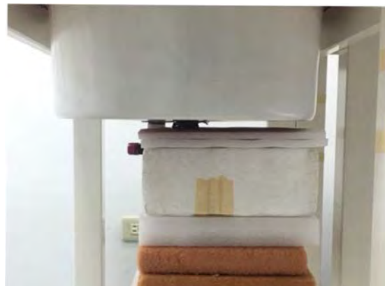
Fig.3 EUT Back side to flat phantom
