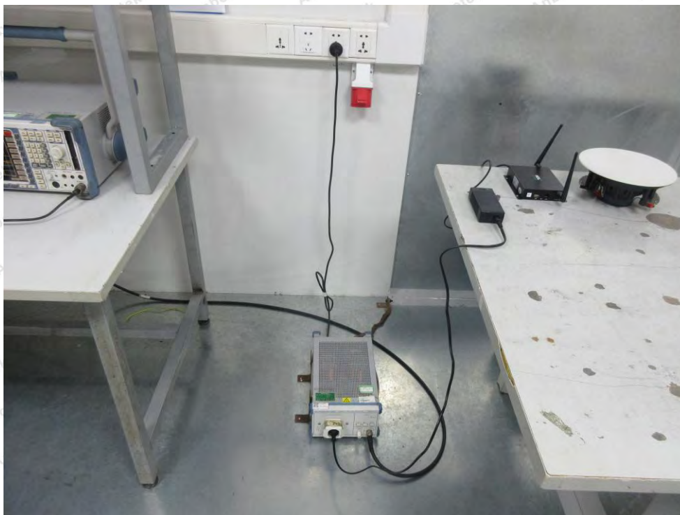
Photo of Conducted Emission Measurement
