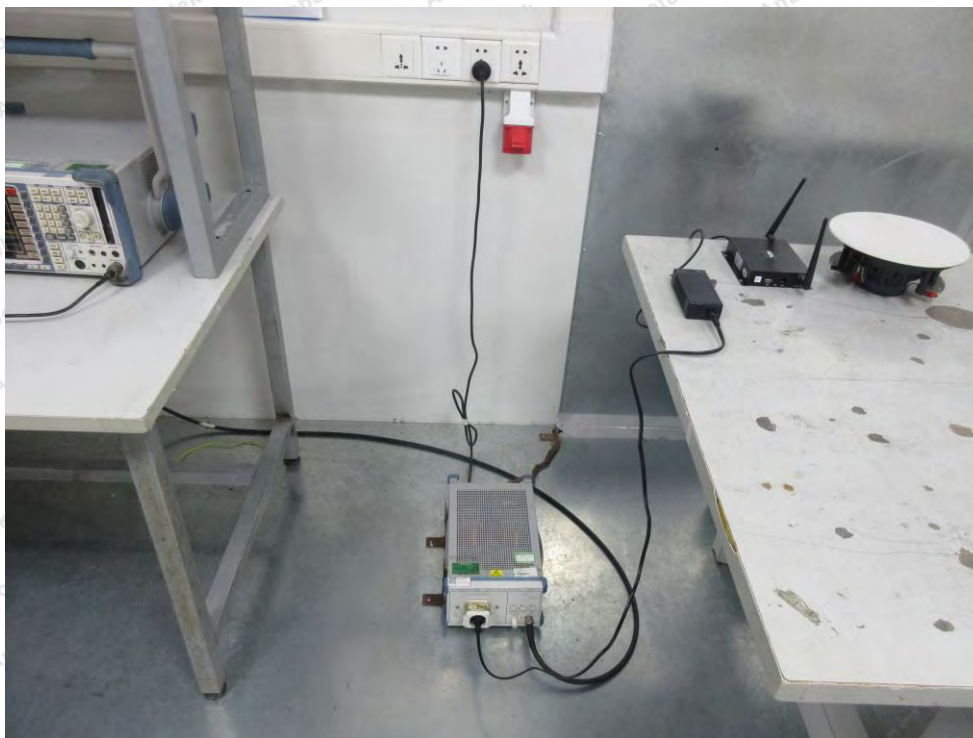
Photo of Conducted Emission Measurement
