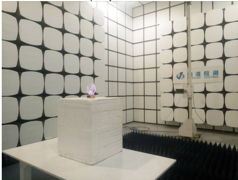
Test frequency from 1GHz-18GHz
