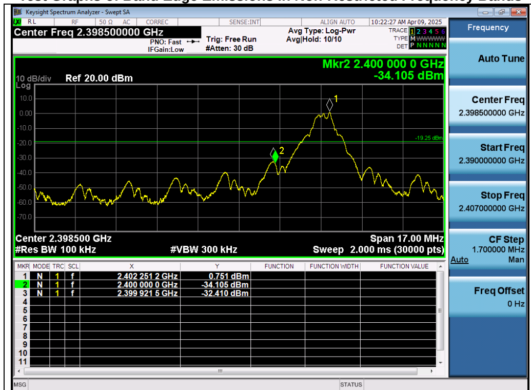
Test_Graph_LE1M_ANT1_2402_1Mbps_Lower Band Edge Emissions
