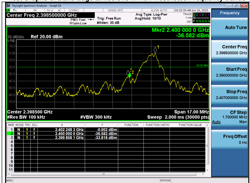
Test_Graph_LE1M_ANT1_2402_1Mbps_Lower Band Edge Emissions
