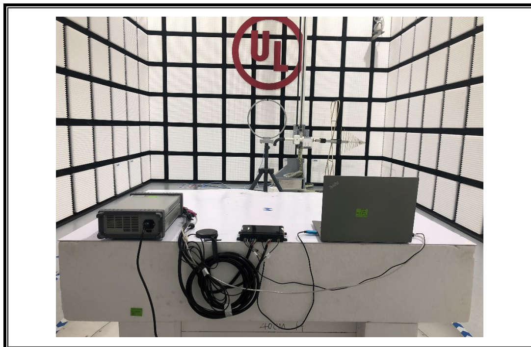
RADIATED RF MEASUREMENT SETUP (Below 30MHz)
